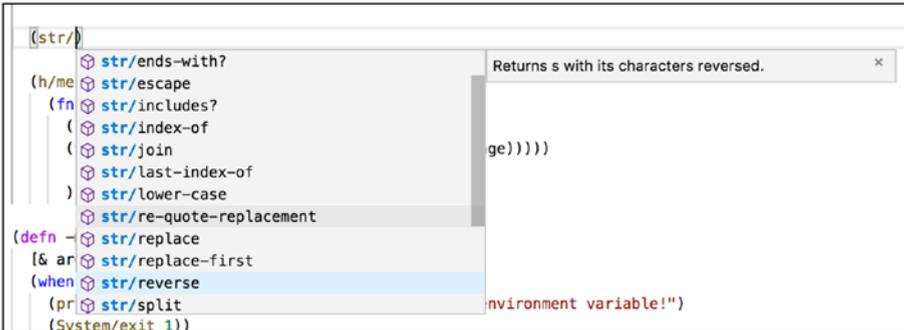
**Figure 7-5.** *reverse function, shown alongside all the str/ functions*
