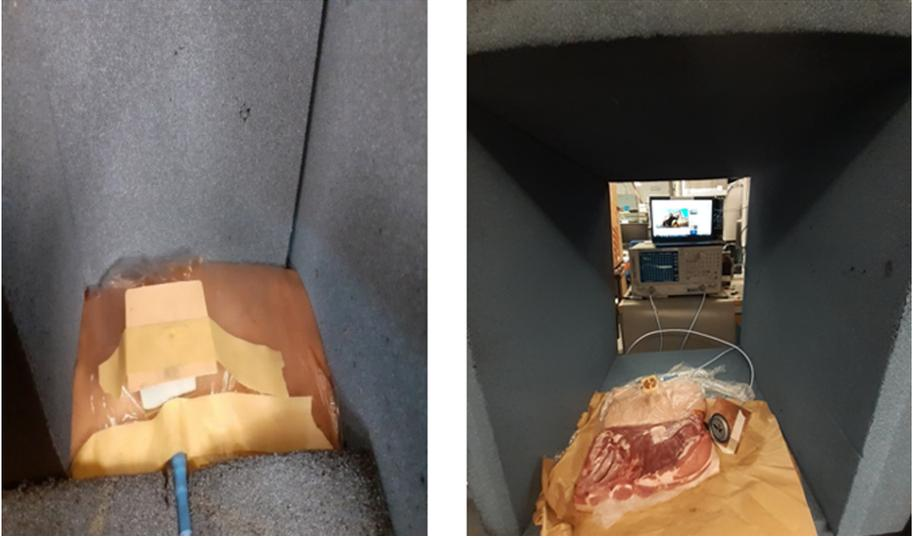
**Fig. 7.** UWB measurement setup inside the cube made from absorber pieces [3].
