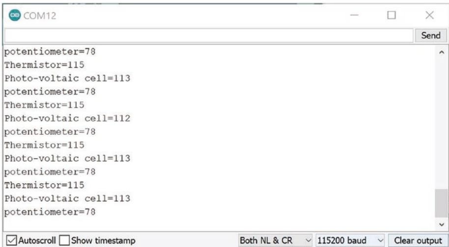
**Figure 2-24.** Program output for reading sensors over I2C
