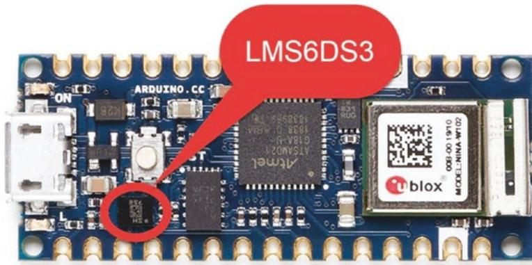
**Figure 3-1.** LSM6DS3 chip on Arduino Nano 33 IoT
