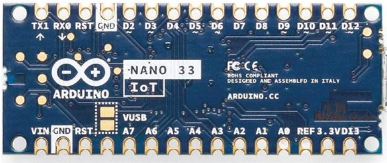
**Figure 2-9.** *Arduino Nano 33 IoT pinout*
