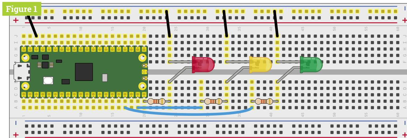
ground rail. Take another, and connect the ground rail to one of your Pico's ground (GND) pins – in **Figure 1**, we've used the ground pin on row three of the breadboard.
