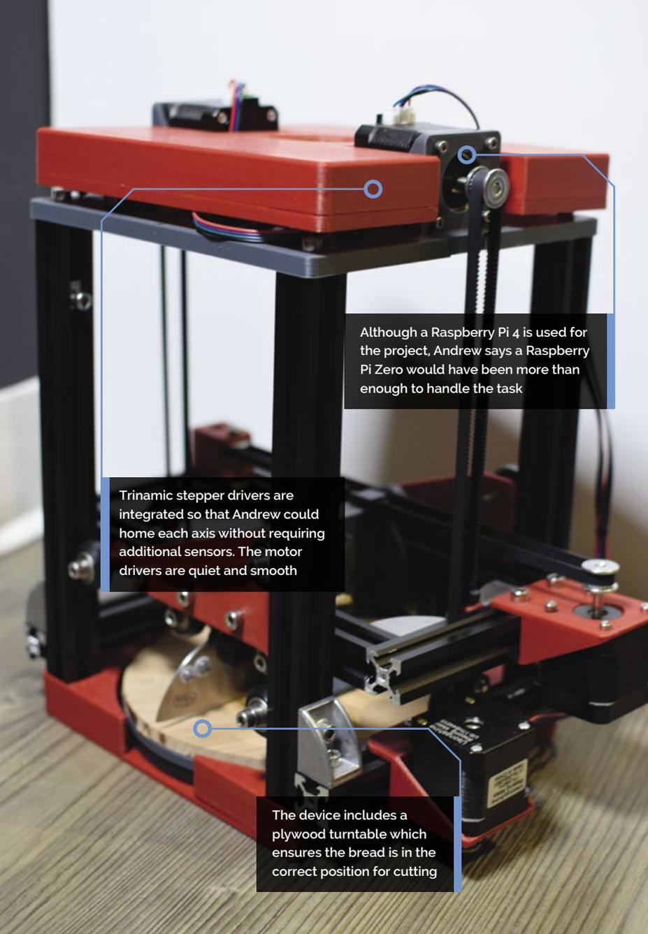
Although a Raspberry Pi 4 is used for the project, Andrew says a Raspberry Pi Zero would have been more than enough to handle the task
