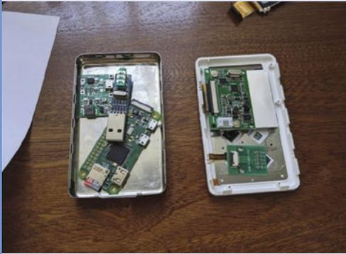
**01** Carefully open up the MP3 player you're repurposing, remove its existing components, retaining anything you'll reuse, then check the replacement parts will fit within the chassis.
