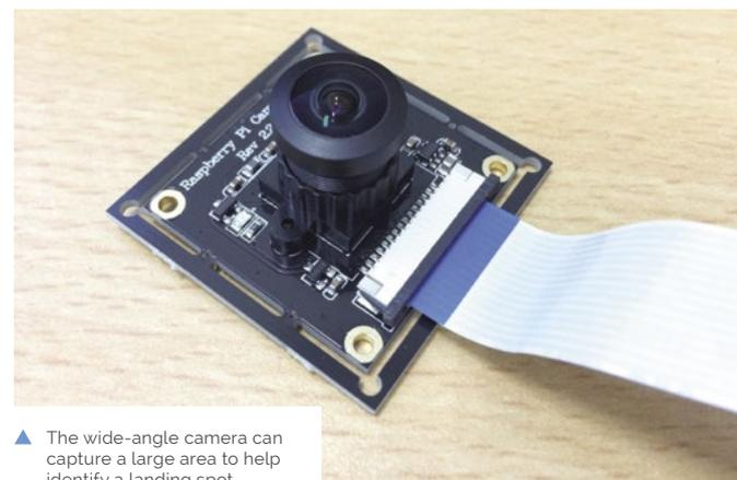
▲ The wide-angle camera can capture a large area to help identify a landing spot
