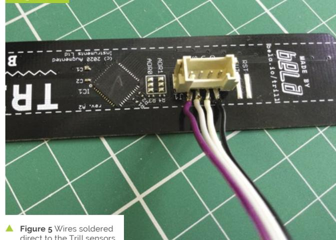
▲ Figure 5 Wires soldered direct to the Trill sensors
