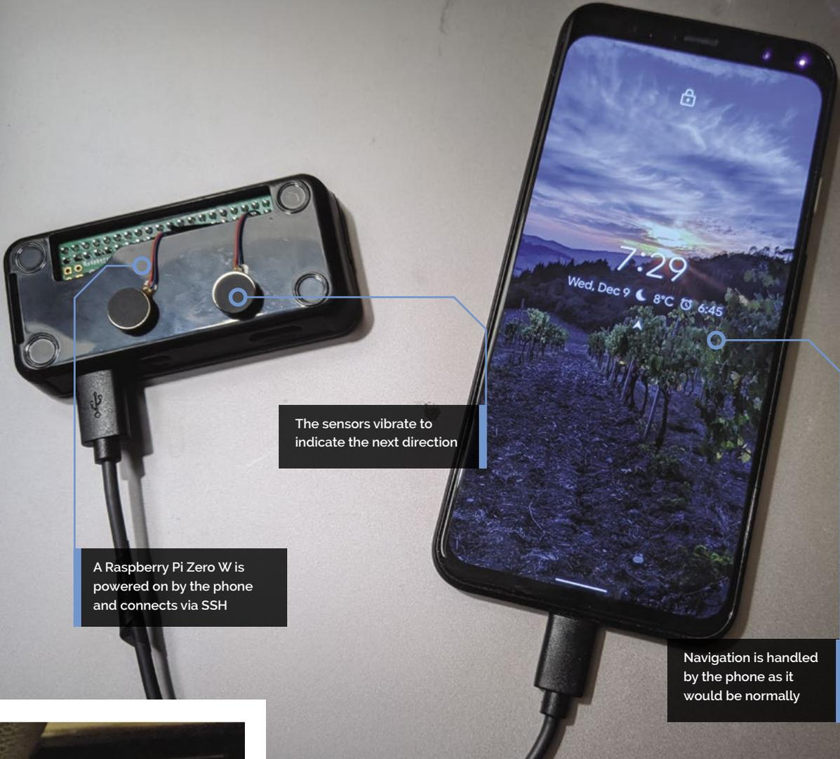
The sensors vibrate to indicate the next direction
