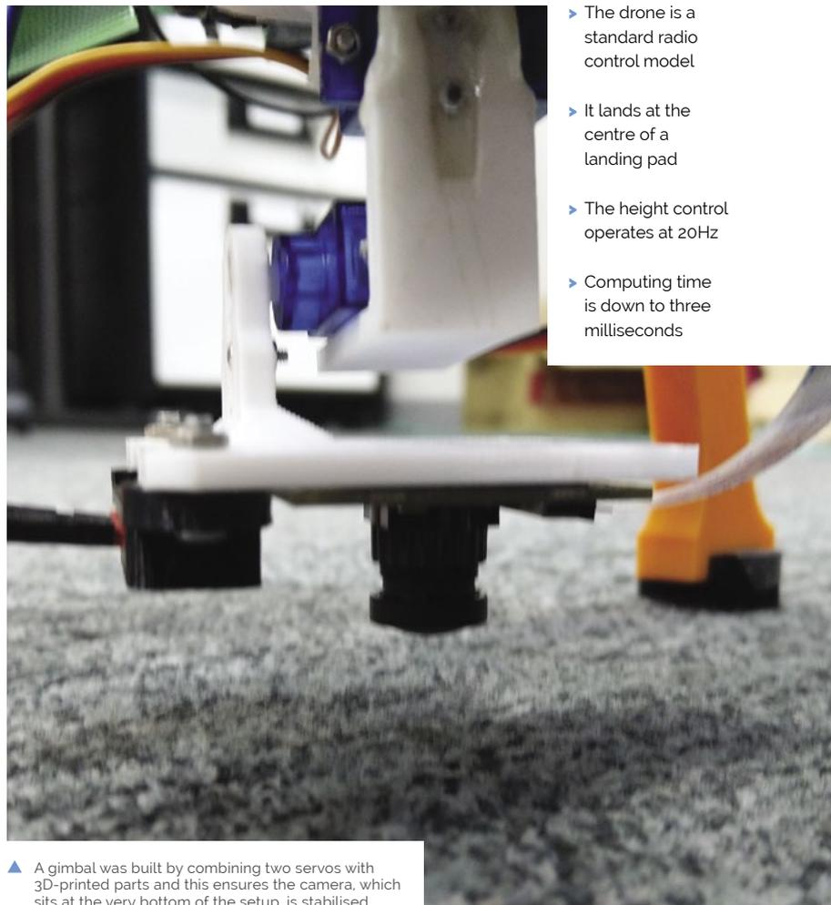
▲ A gimbal was built by combining two servos with 3D-printed parts and this ensures the camera, which sits at the very bottom of the setup, is stabilised
