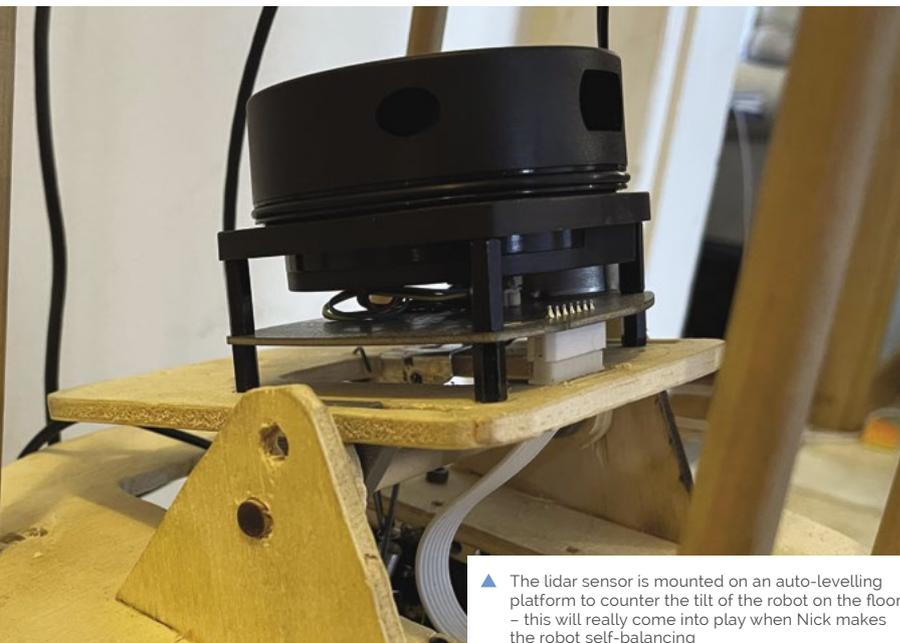
▲ The lidar sensor is mounted on an auto-levelling platform to counter the tilt of the robot on the floor – this will really come into play when Nick makes the robot self-balancing
