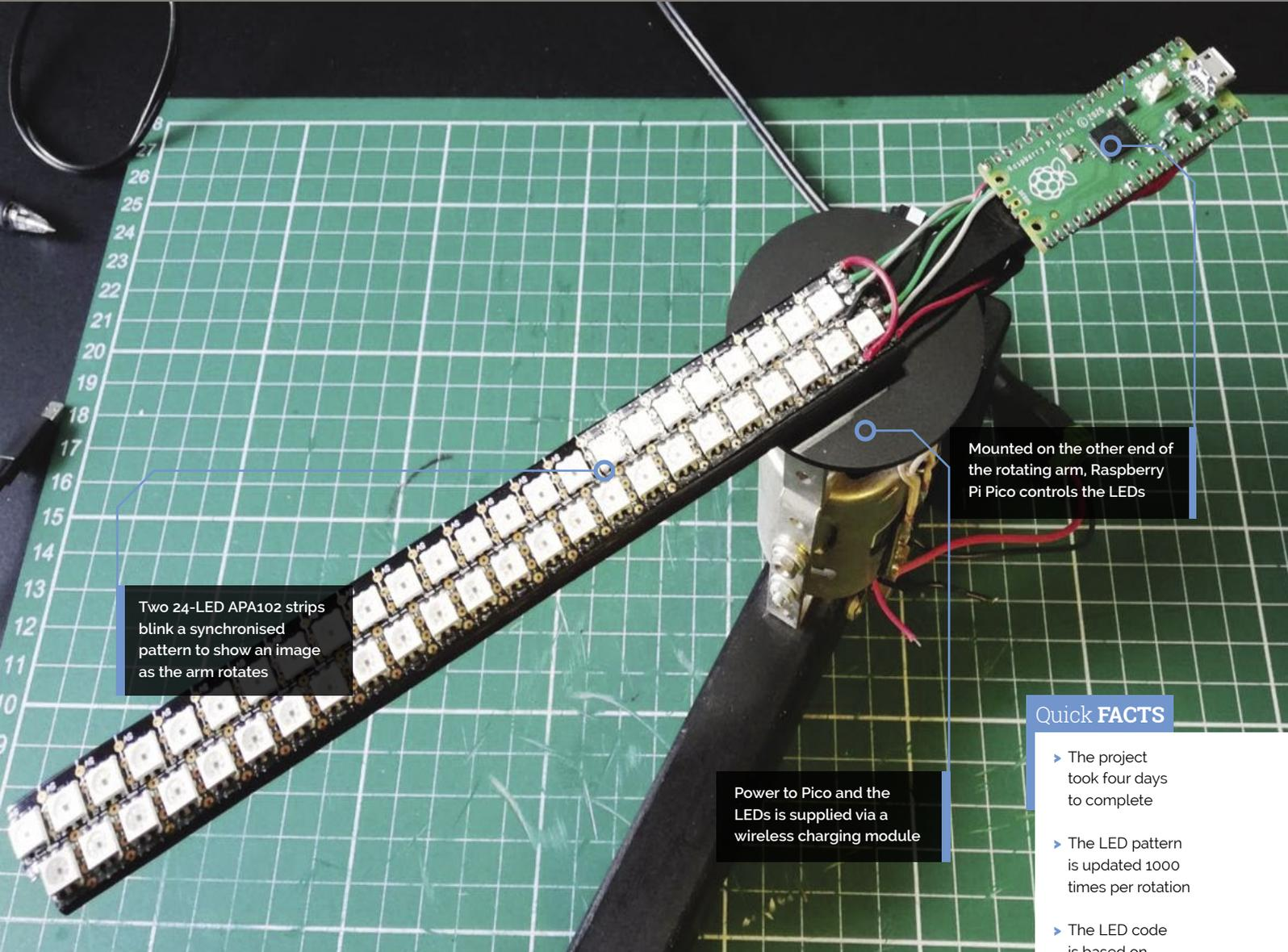
Two 24-LED APA102 strips blink a synchronised pattern to show an image as the arm rotates
