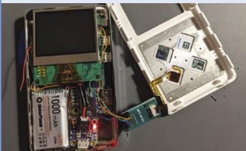
**03** Tape off any conductive elements in the case to prevent short-circuiting. Test Raspotify and install on Raspberry Pi Zero before mounting it in your new music player and powering it up.
