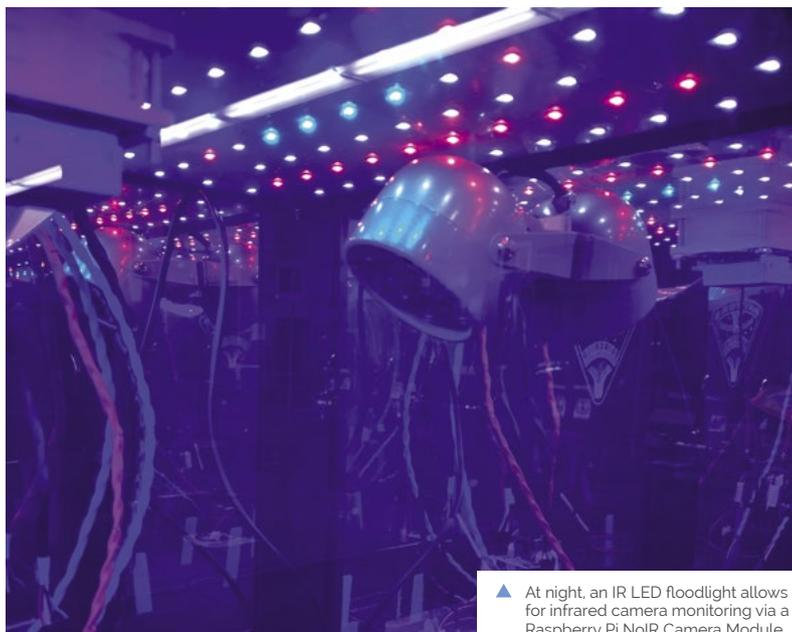
▲ At night, an IR LED floodlight allows for infrared camera monitoring via a Raspberry Pi NoIR Camera Module
