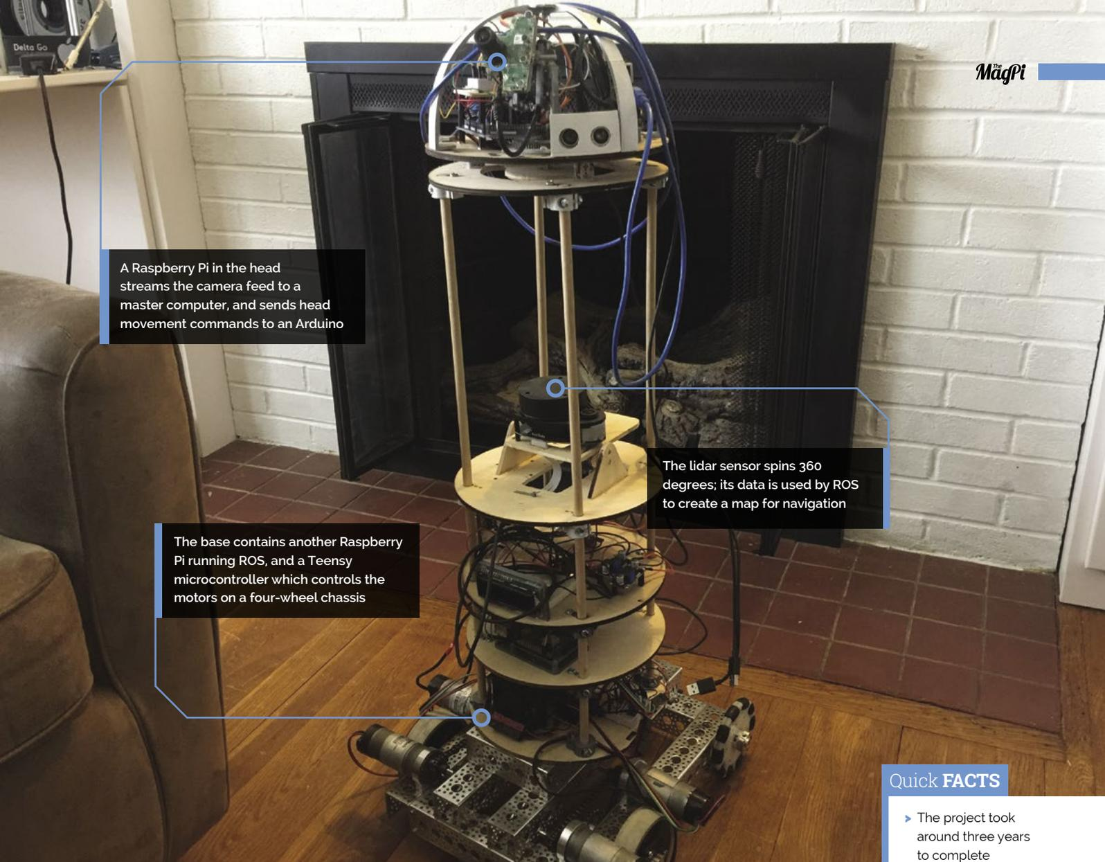
A Raspberry Pi in the head streams the camera feed to a master computer, and sends head movement commands to an Arduino
