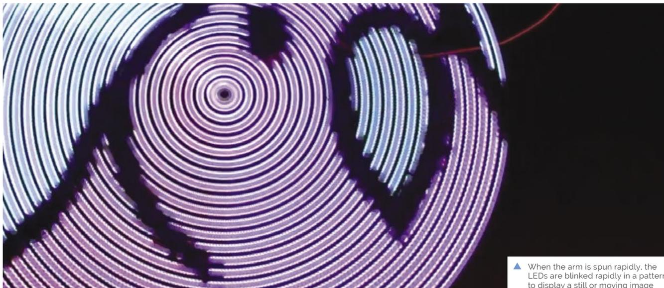
▲ When the arm is spun rapidly, the LEDs are blinked rapidly in a pattern to display a still or moving image
