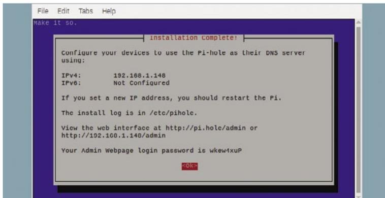
▲ When you've finished setting up Pi-hole, make a note of the IPv4 address and password for later use
