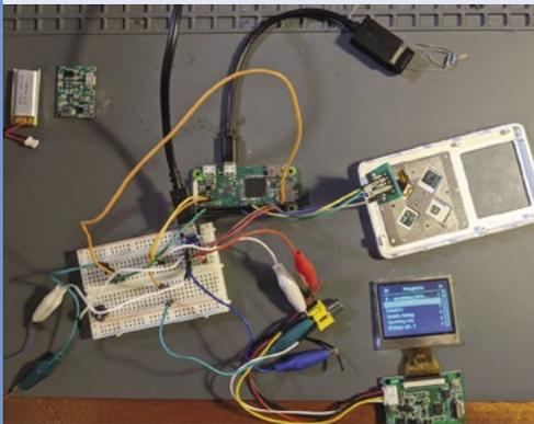
**02** Install the C-based haptic code on Raspberry Pi Zero. Connect Raspberry Pi, display, headers, and leads. Then power on and check the click wheel data is recognised and drives the haptic motor.
