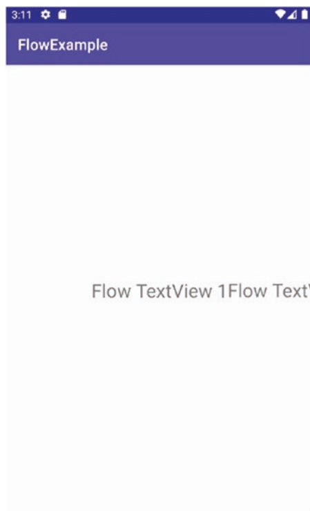
Figure 10-2. Without Flow, the ConstraintLayout renders widgets off-screen
