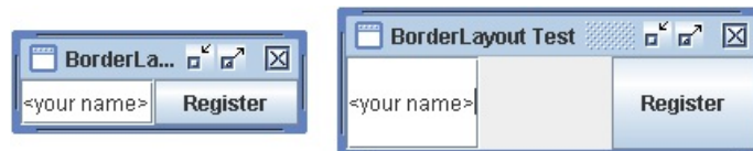
Figure 23.2: A JFrame that uses a BorderLayout (left) and the same JFrame resized (right)
