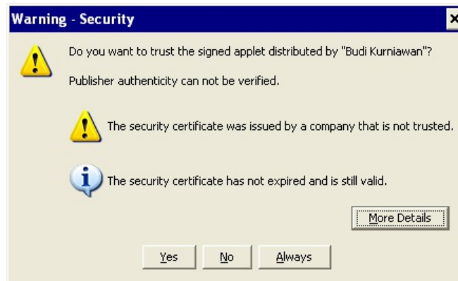
Figure 31.6: The security warning asking the user whether to grant permissions to an applet
