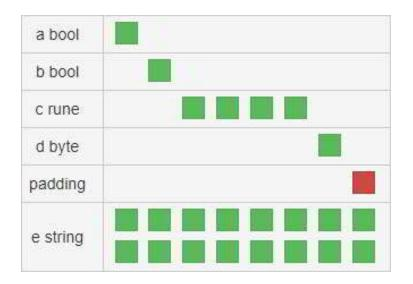
We can clearly see that both the Boolean variables, the rune and the byte, are in the same memory address, and a byte of padding is added to align the last field.
