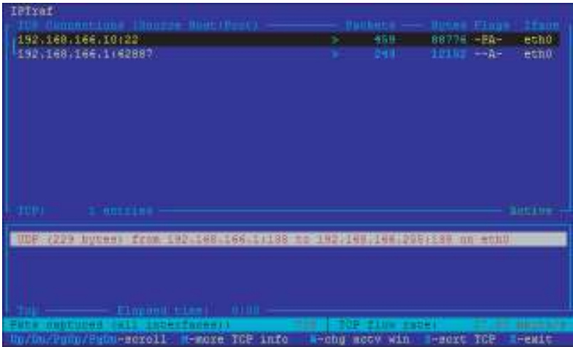
FIGURE 17.2 IPTraf provides a quick overview of the kind of traffic sent on an interface.
