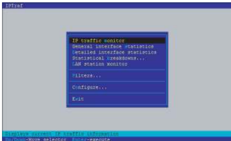
FIGURE 17.1 IPTraf allows you to analyze network traffic from a menu interface.
