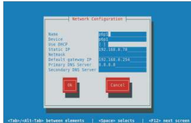
FIGURE 6.4 Entering network parameters in system-config-network
