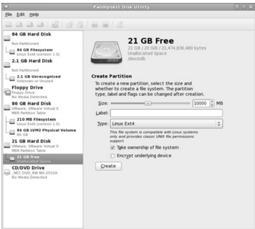
Figure 3-24 An empty disk with a partition table
