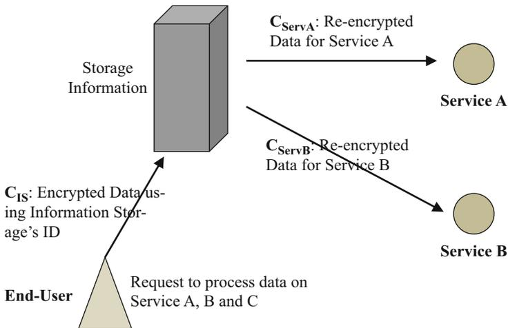
**Fig. 4.5** Proxy re-encryption
