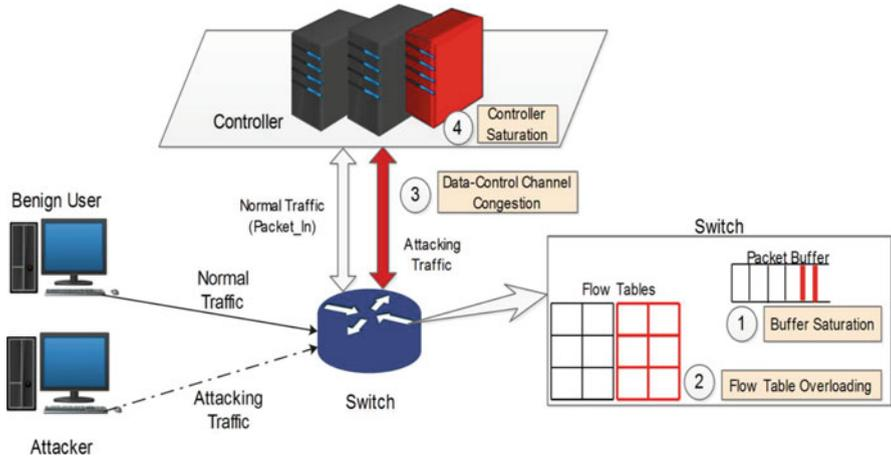
Fig. 15.9 DDoS attack in SDN
