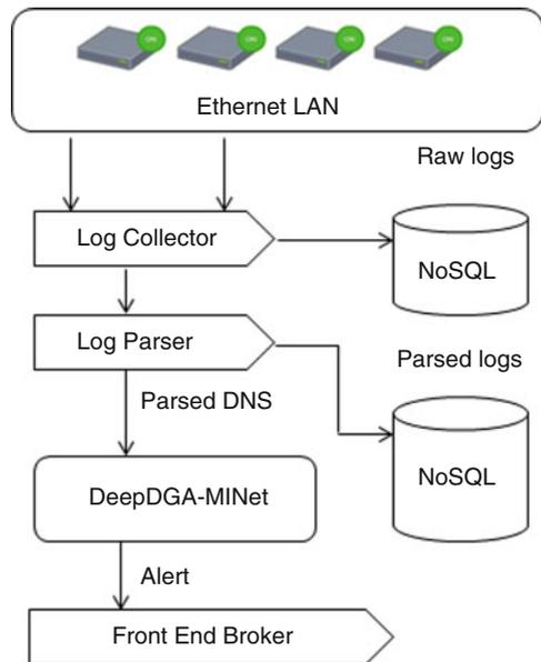
**Fig. 37.6** A detailed overview of DeepDGA-MINet
