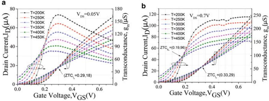
**Fig. 12.3**  $I_D$  and  $g_m$  versus  $V_{GS}$  characteristics of high-k SOI FinFET with temperature variation at (a)  $V_{DS} = 0.05$  V and (b)  $V_{DS} = 0.7$  V
