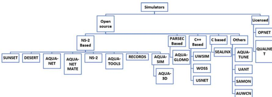
Fig. 9.2 Different simulators for underwater wireless sensor networks
