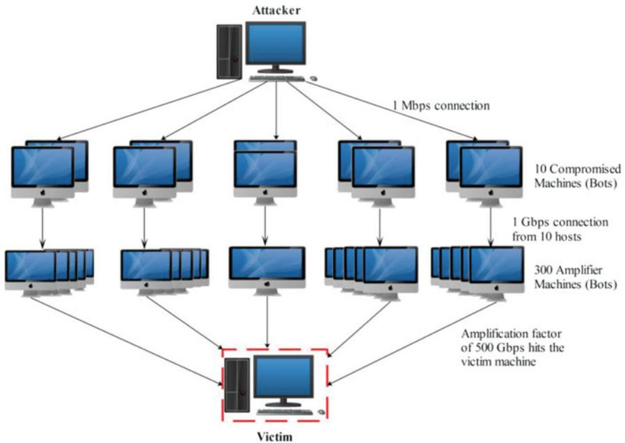
Fig. 15.6 Amplified DDoS attack
