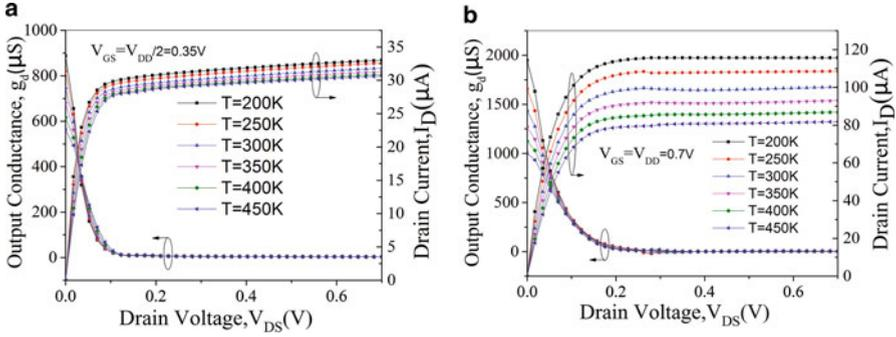
**Fig. 12.4**  $I_D$  and  $g_d$  versus  $V_{DS}$  characteristics of high- $k$  SOI FinFET with temperature variation at (a)  $V_{GS} = 0.35$  V and (b)  $V_{GS} = 0.7$  V
