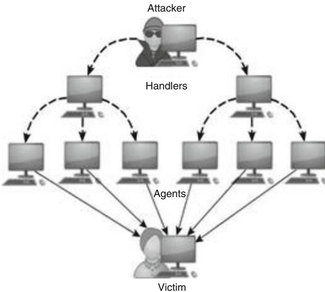
Fig. 16.5 IRC model of DDoS attack network
