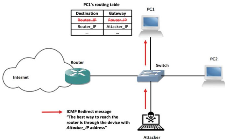
Fig. 6.22 Performing a MITM attack through ICMP redirect messages.
