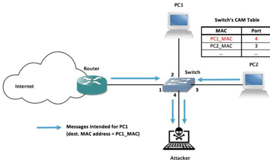
Fig. 6.9 Effects of the port stealing attack
