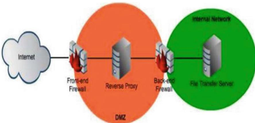
Fig. 13.6 Firewall architecture
