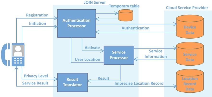
Fig. 1.7 Components of the proposed framework and their interactions
