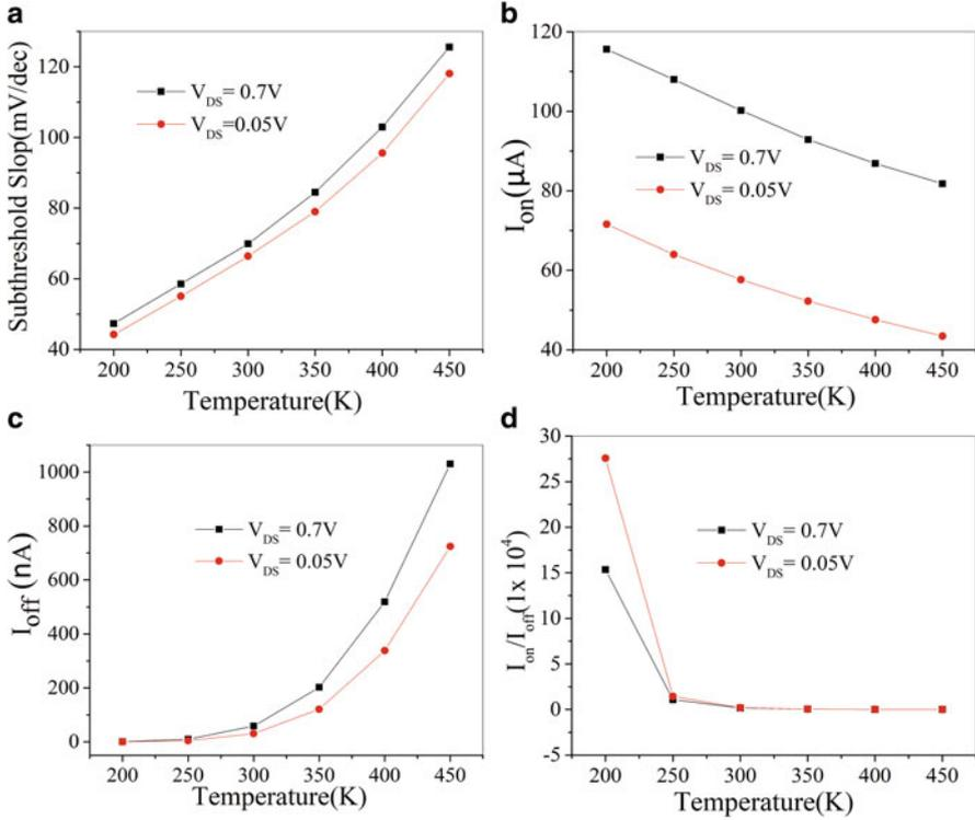
**Fig. 12.2** (a) SS, (b)  $I_{on}$  current, (c)  $I_{off}$  current, and (d)  $I_{on}/I_{off}$  ratio versus temperature characteristics for high-k SOI FinFET at  $V_{DS} = 0.05\text{ V}$  and  $V_{DS} = 0.7\text{ V}$
