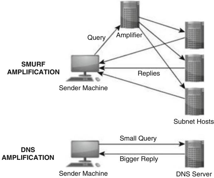
Fig. 16.8 Smurf vs DNS amplification
