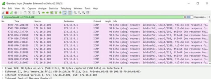
Fig. 6.5 The network capture on the link of the attacker shows that the attacker is receiving messages from the victim intended to the router
