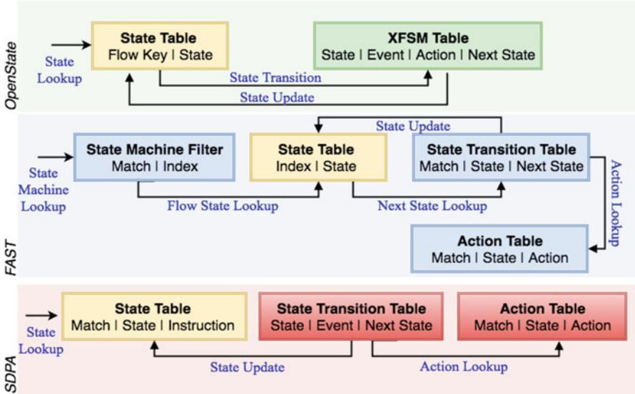
**Fig. 14.3** Tables used in OpenState, FAST, and SDPA architectures. Each table is represented as a rectangle containing the table name and the corresponding table columns separated with ‘|’
