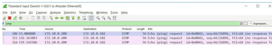
Fig. 6.20 The victim is receiving messages from an attacker located in a different VLAN
