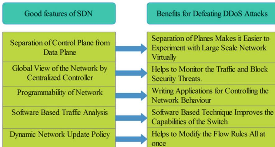
**Fig. 15.8** Good features in SDN for defeating DDoS attack
