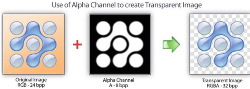
**Fig. 33.2** Creation of a transparent image with an Alpha channel
