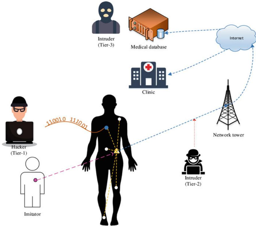
Fig. 8.2 Areas prone to attack in wireless body area networks
