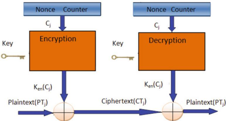
**Fig. 7.7** CTR encryption and decryption processes
