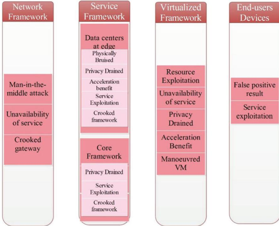
Fig. 20.7 Security threat model for fog computing
