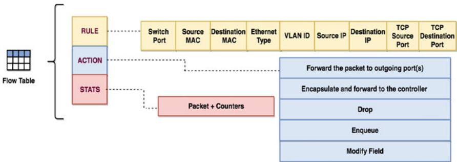
Fig. 14.2 Flow table of an OpenFlow-enabled forwarding device
