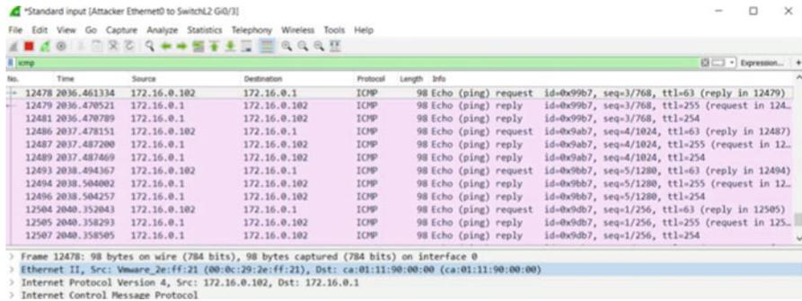
Fig. 6.6 Successful MITM attack; the messages are reaching both the victim and the router, but the attacker is in the middle of the communication
