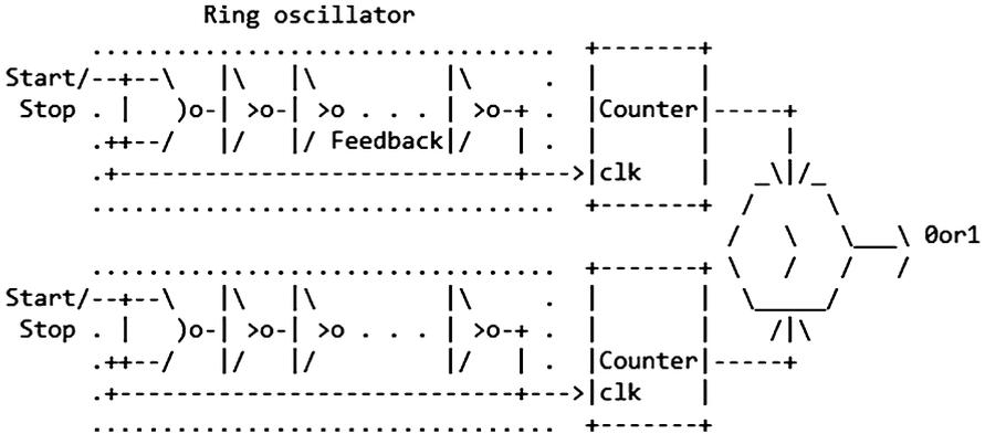
Fig. 18.3 Ring oscillator Physical Unclonable Function (PUF)
