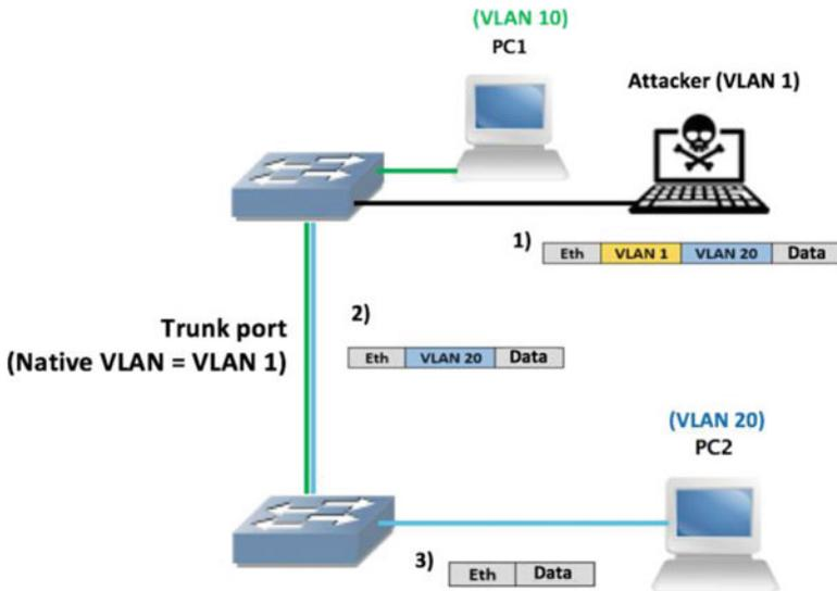
Fig. 6.16 VLAN hopping through the double-tagging technique
