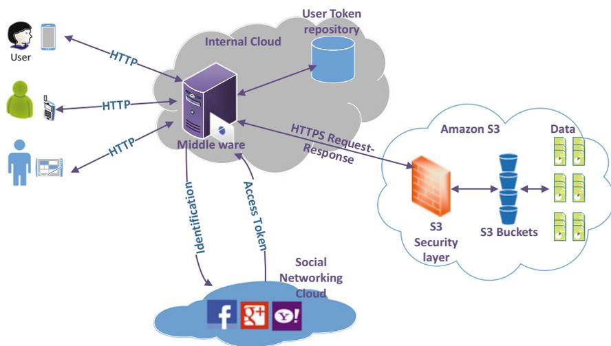
Fig. 1.5 Framework for authentication using middleware-layer for MCC
