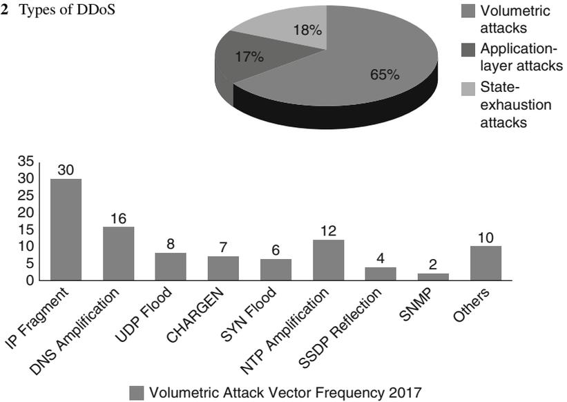
**Fig. 16.3** DDoS attack vectors recorded
