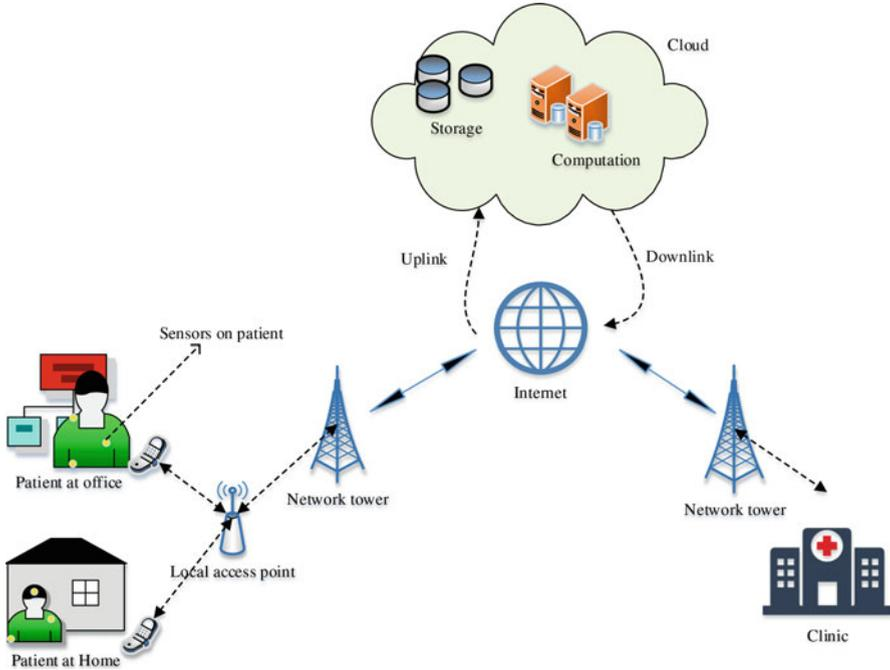
**Fig. 8.3** Architecture of cloud assisted wireless body area networks
