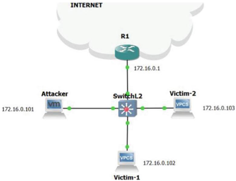
Fig. 6.2 Emulated network scenario for layer two attacks
