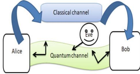
protocol announced by Bennett in 1992 (B92) [39]. Accordingly, in this study, we consider that Alice and Bob share information with the standard BB84 protocol using coherent states as an encoding basis. In fact, in the BB84 protocol each signal is transmitted by a single qubit sent by Alice and received by Bob. The qubit encrypted a key bit in one of the two conjugate orthonormal bases. When Alice uses the horizontal/vertical ( $H=V$ ) basis, her signal states are given by:
