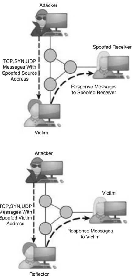
making the DDoS attack successful. Figure 16.9 illustrates the attack mechanism. The largest on record DDoS attack is caused by DNS amplification. The ratio of query to reply of DNS server is 1:70, whereas for NTP server, it ranges from 1:20 to 1:200.
