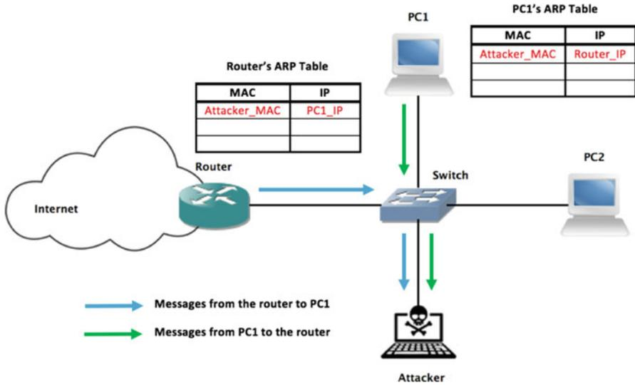
Fig. 6.1 Effects of a MITM attack
