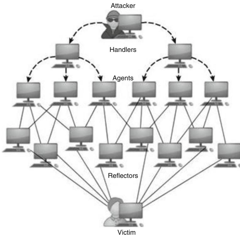
**Fig. 16.6** Reflector model of DDoS attack network
