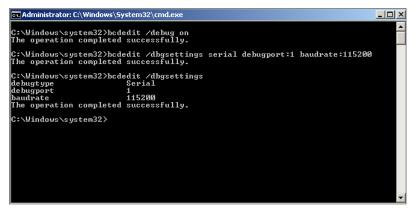
Figure 2-7: Setting up kernel debugging on Windows 7 with bcdedit
