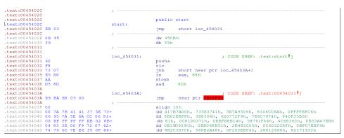
Figure 8-1: FlyStudio malware disassembled code
