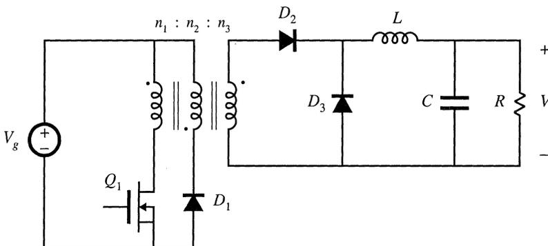
Fig. 6.22 Single-transistor forward converter.
