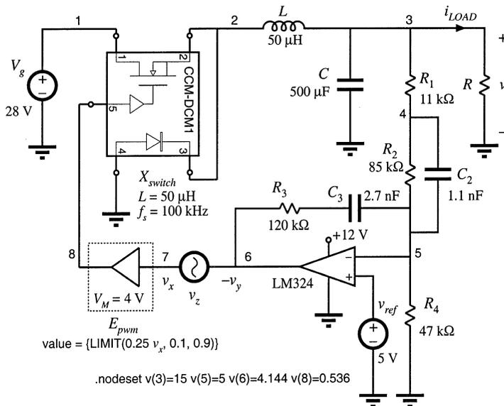
Fig. B.15 Buck voltage regulator example.
