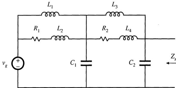
Fig. 8.69 Input filter circuit of Problem 8.13.
