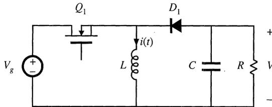
Fig. 5.21 Buck-boost converter of Problems 5.1 and 5.13.
