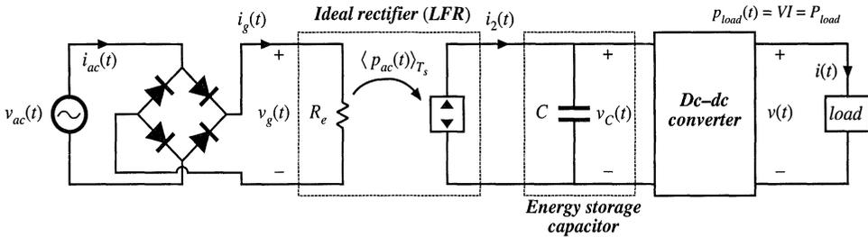
**Fig. 18.25** Elements of a single-phase-ac to dc power supply, in which the ac line current and dc load voltage are independently regulated with high bandwidth. An internal independent energy storage capacitor is required.
