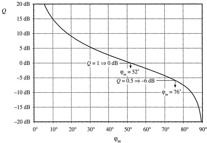
Fig. 9.13 Relationship between loop-gain phase margin  $\phi_m$  and closed-loop peaking factor  $Q$ .
