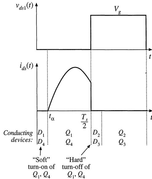
allel diodes conduct. Since the transistor voltage is zero during the entire turn on transition, switching loss due to slow turn-on times or due to energy storage in any of the device capacitances does not occur at turn-on.
