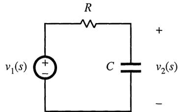
Fig. 8.4 Simple  $R$ - $C$  low-pass filter example.
