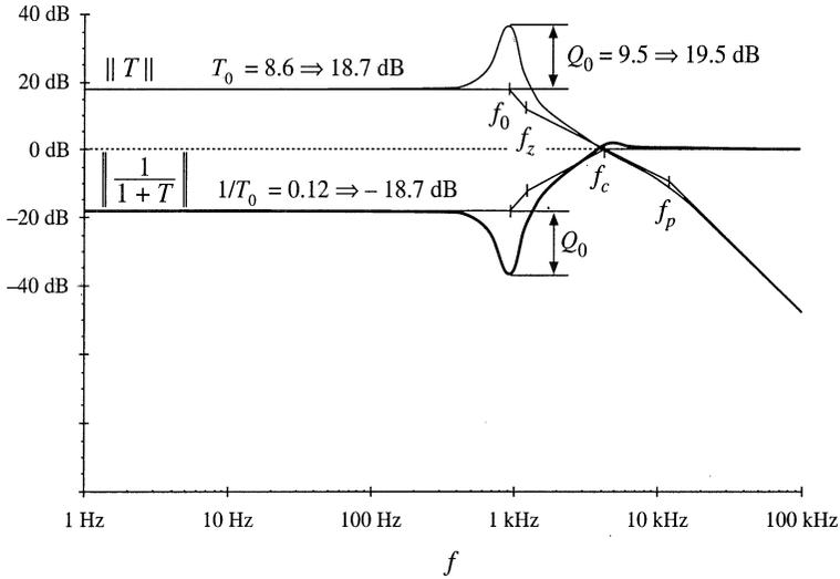
Fig. 9.29 Construction of  $\| 1/(1 + T) \|$  for the PD-compensated design example of Fig. 9.28.
