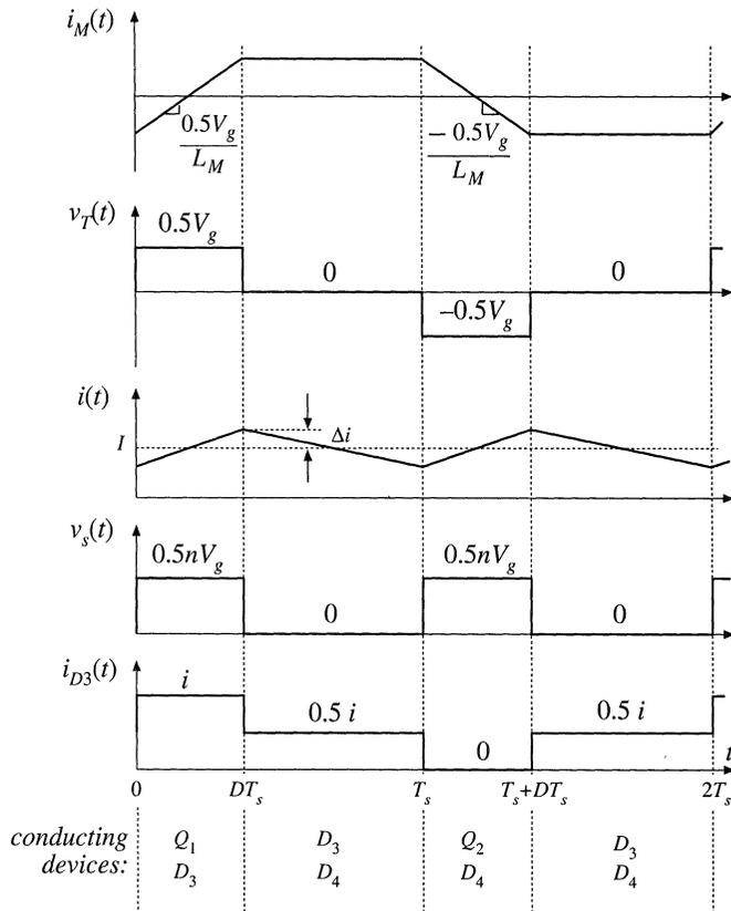
Fig. 6.21 Waveforms of the half-bridge transformer-isolated buck converter.
