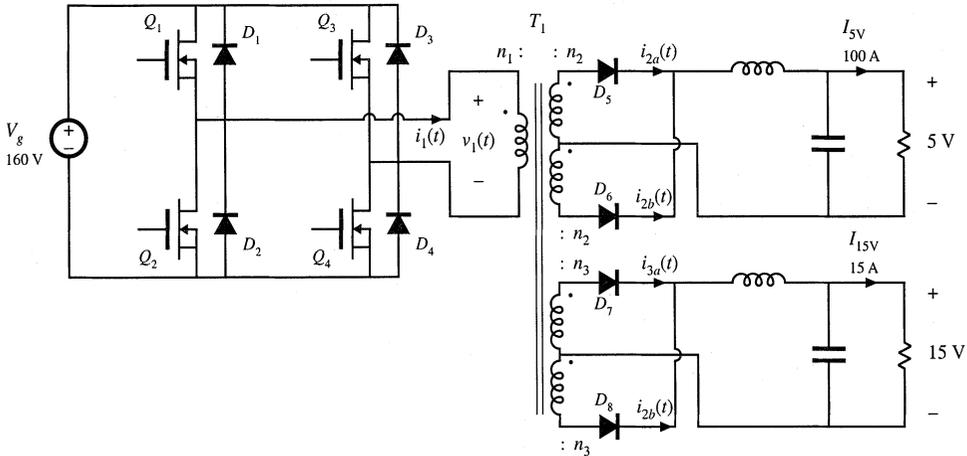
Fig. 15.8 Multiple-output full-bridge isolated buck converter example.
