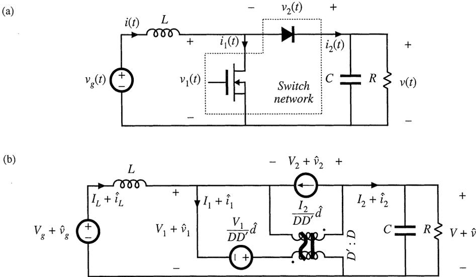
**Fig. 7.44** Construction of an averaged circuit model for an ideal boost converter example: (a) converter circuit with the switch network of Fig. 7.39(a) identified; (b) a dc and small-signal ac averaged circuit model obtained by replacing the switch network with the model of Fig. 7.39(d).
