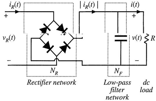
ple approximation as usual:  $v(t) \approx V$ ,  $i(t) \approx I$ . The diode rectifiers switch when  $i_R(t)$  passes through zero, as shown in Fig. 19.11. The rectifier input voltage  $v_R(t)$  is essentially a square wave, equal to  $+v(t)$  when  $i_R(t)$  is positive and  $-v(t)$  when  $i_R(t)$  is negative. Note that  $v_R(t)$  is in phase with  $i_R(t)$ .
