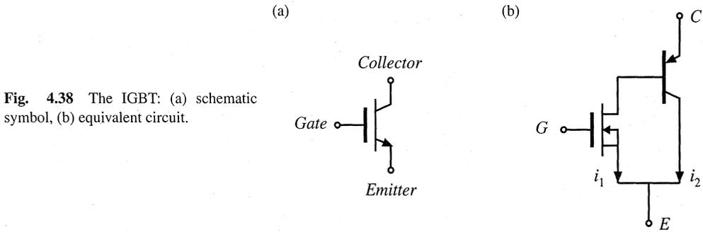
Fig. 4.38 The IGBT: (a) schematic symbol, (b) equivalent circuit.
