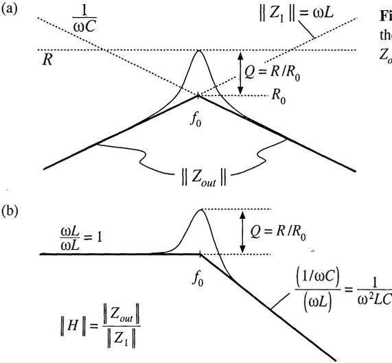
**Fig. 8.51** Graphical construction of  $H$  and  $Z_{out}$  of the voltage divider circuit: (a) output impedance  $Z_{out}$ ; (b) transfer function  $H$ .
