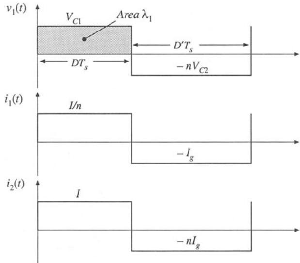
Fig. 15.6 Waveforms, Cuk converter transformer design example.
