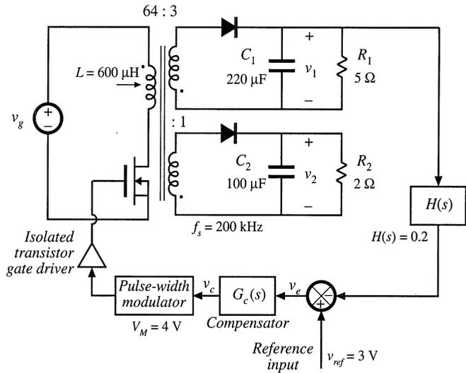
**Fig. 9.41** Flyback converter system of Problem 9.2.
