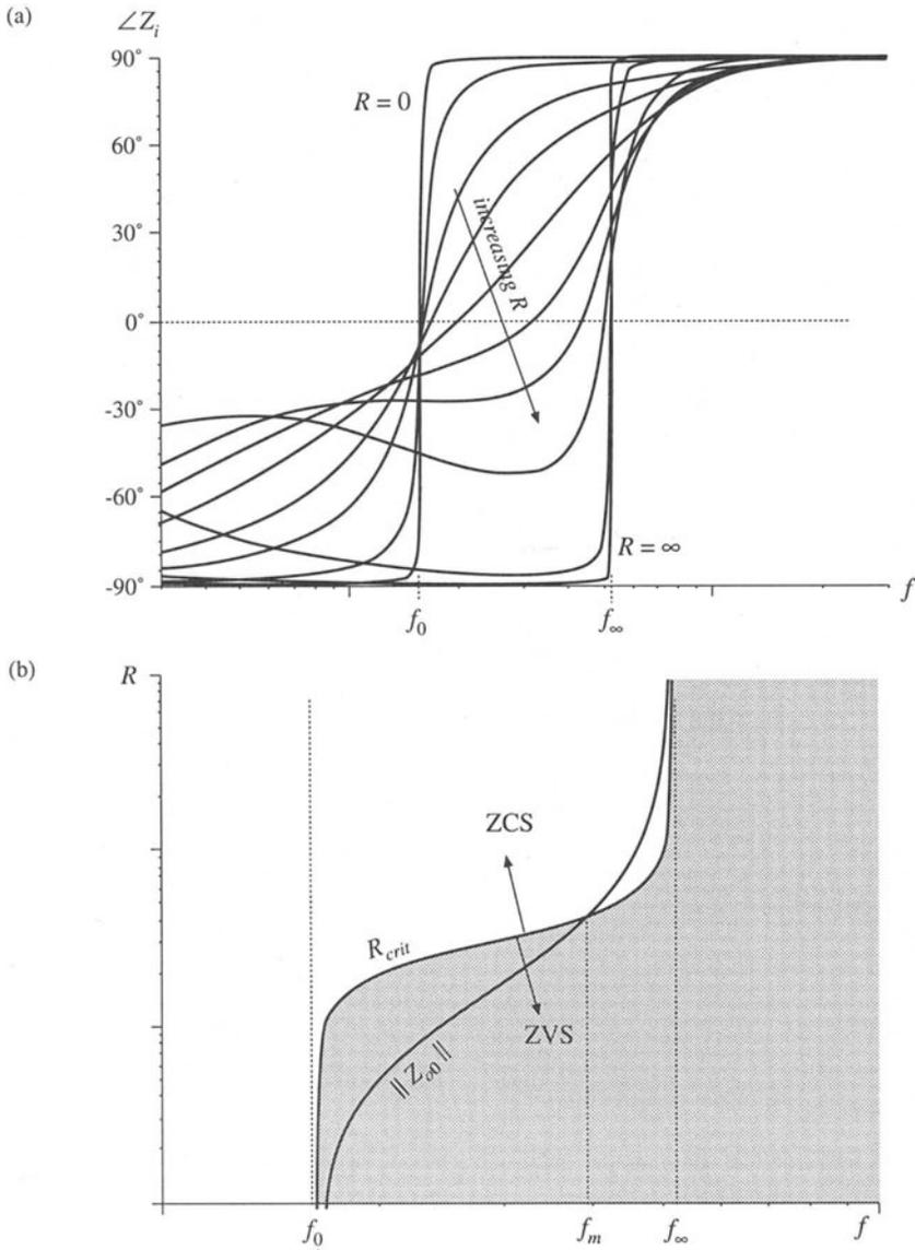
**Fig. 19.38** ZCS/ZVS boundary, LCC inverter example: (a) variation of tank network input impedance phase shift with load resistance, (b) Comparison of  $R_{crit}$  with matched-load impedance  $\parallel Z_{o0} \parallel$ .
