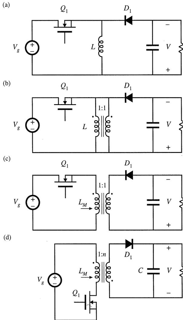
**Fig. 6.30** Derivation of the flyback converter: (a) buck-boost converter; (b) inductor  $L$  is wound with two parallel wires; (c) inductor windings are isolated, leading to the flyback converter; (d) with a 1:n turns ratio and positive output.
