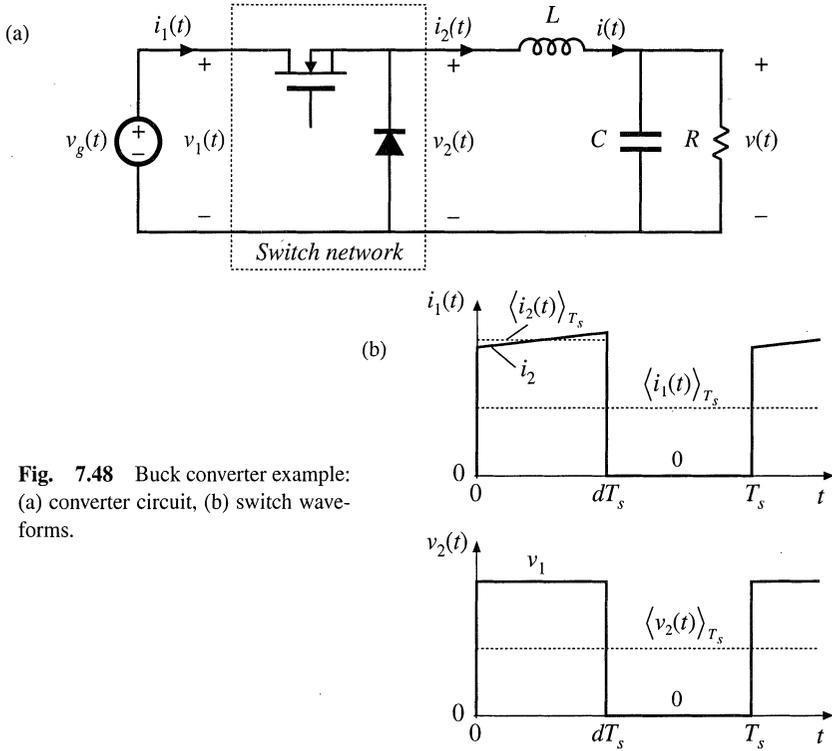
**Fig. 7.48** Buck converter example: (a) converter circuit, (b) switch waveforms.
