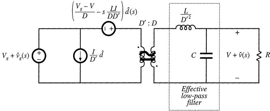
Fig. 7.61 The buck-boost converter model, in canonical form.
