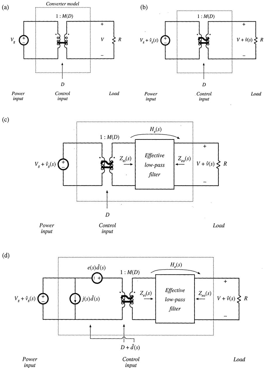
**Fig. 7.58** Development of the canonical circuit model, based on physical arguments: (a) dc transformer model, (b) inclusion of ac variations, (c) reactive elements introduce effective low-pass filter, (d) inclusion of ac duty cycle variations.
