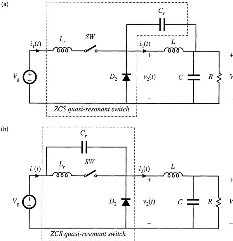
**Fig. 20.21** Connection of the tank capacitor of the ZCS quasi-resonant cell to other points at ac ground: (a) connection to the dc output, (b) connection to the dc input. In each case, the ac components of the waveforms are unchanged.
