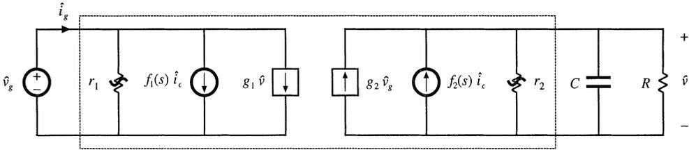
**Fig. 12.15** Two-port equivalent circuit used to model the current-programmed CCM buck, boost, and buck–boost converters.
