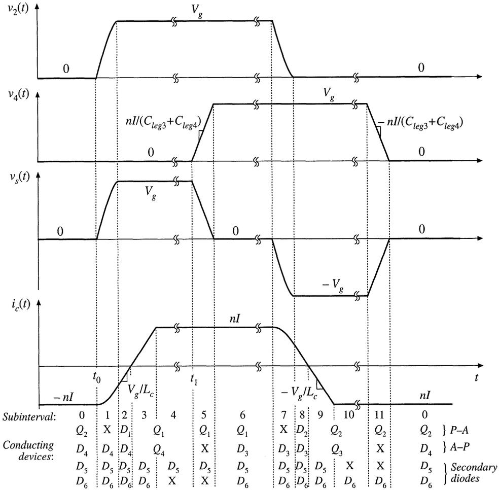
Fig. 20.38 Detailed diagram of primary-side waveforms of the ZVT full-bridge converter, illustrating the zero-voltage switching mechanisms. An ideal transformer is assumed.
