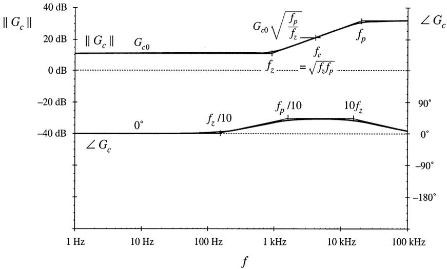
Fig. 9.27 PD compensator transfer function  $G_c$ , design example.
