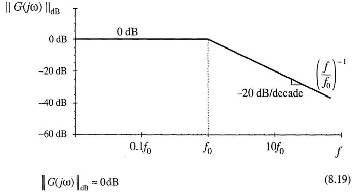
Thus, as illustrated in Fig. 8.6, at low frequency  $\|G(j\omega)\|_{\text{dB}}$  is asymptotic to 0 dB.
