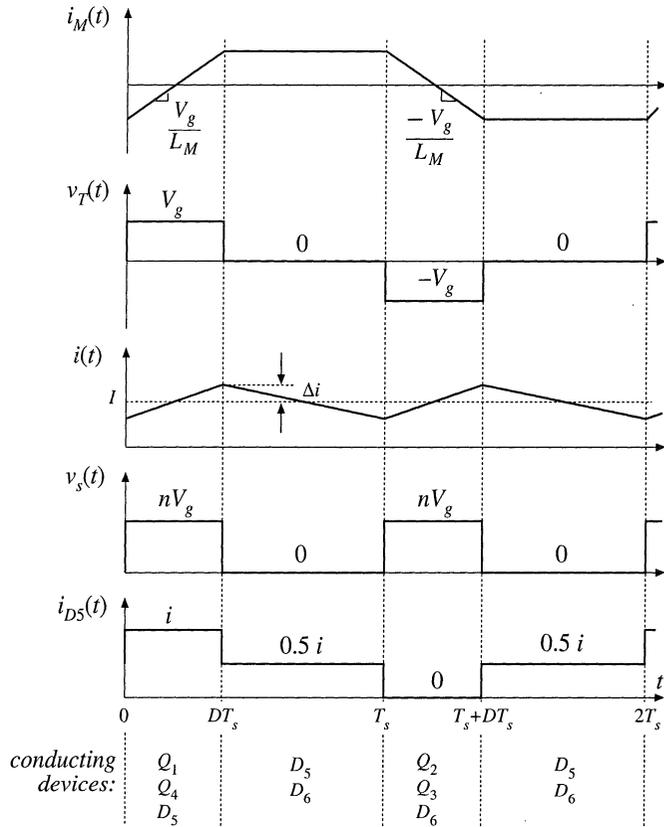
6.18(b) is obtained. Typical waveforms are illustrated in Fig. 6.19. The output portion of the converter is similar to the nonisolated buck converter—compare the  $v_s(t)$  and  $i(t)$  waveforms of Fig. 6.19 with Figs. 2.1(b) and 2.10.
