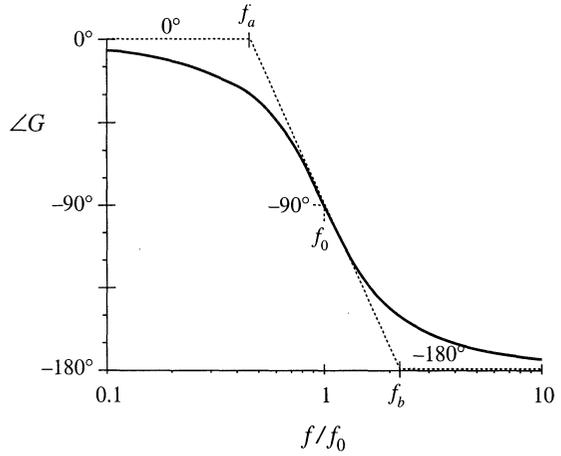
**Fig. 8.23** A simpler choice for the midfrequency phase asymptote, which better approximates the curve over the entire frequency range and is consistent with the asymptote used for real poles.
