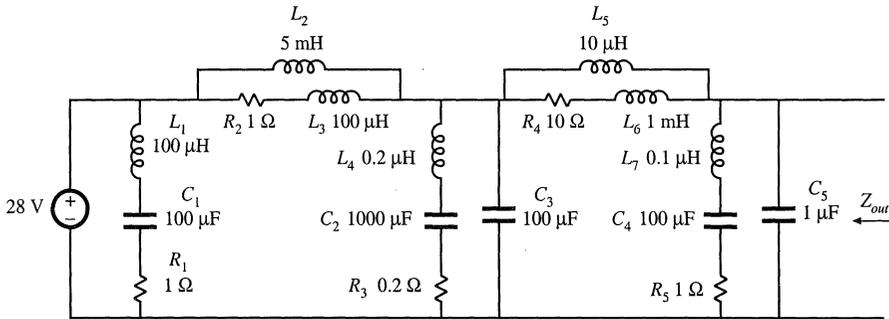
Fig. 8.70 Input filter circuit of Problem 8.14.
