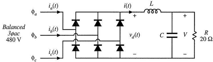
**Fig. 16.14** Three-phase rectifier circuit of Problem 16.2
