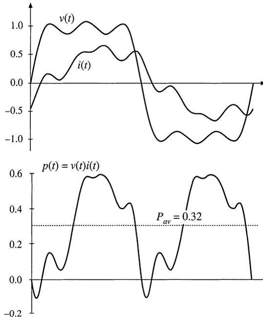
**Fig. 16.4** Voltage, current, and instantaneous power waveforms, example 3. The voltage contains fundamental, third, and fifth harmonics. The current contains fundamental, fifth, and seventh harmonics. Net energy is transmitted at the fundamental and fifth harmonic frequencies.
