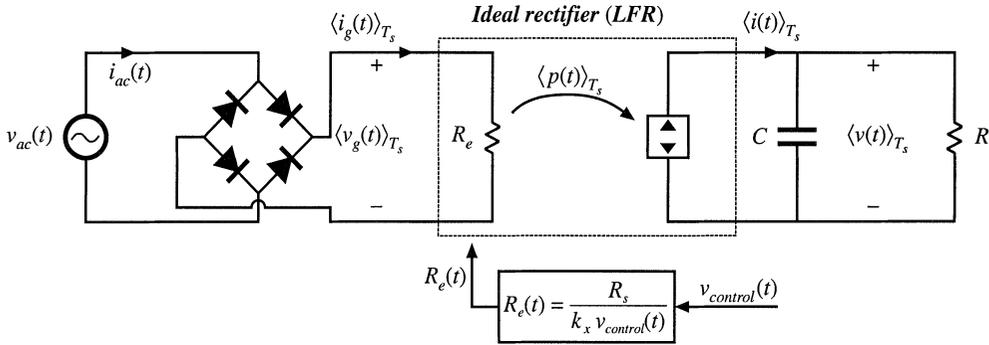
**Fig. 18.12** Model of the system of Fig. 18.5, based on the loss-free resistor model of Fig. 18.1(c), which predicts the low-frequency system waveforms. This model assumes that the feedback loop of Fig. 18.5 operates ideally.
