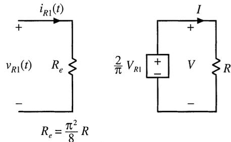
**Fig. 19.21** An equivalent circuit for the rectifier and inductive filter network of the parallel resonant converter, which models the fundamental components of the rectifier ac input waveforms and the dc components of the load waveforms.
