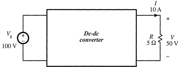
**Fig. 1.6** A simple power processing example: construction of a 500 W dc–dc converter.
