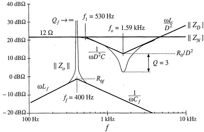
**Fig. 10.13** Impedance design criteria  $\|Z_N(j\omega)\|$  and  $\|Z_D(j\omega)\|$  from Fig. 10.10, with the filter output impedance  $\|Z_o(j\omega)\|$  of Fig. 10.12 superimposed. The design criteria of Eq. (10.13) are not satisfied at the input filter resonance.
