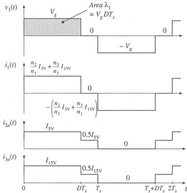
Fig. 15.9 Transformer waveforms, full-bridge converter example.
