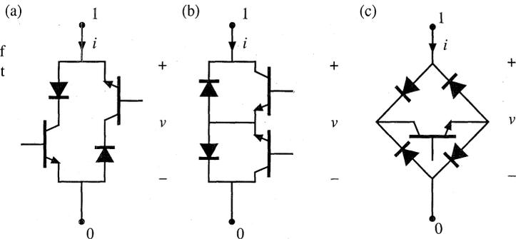
Fig. 4.20 Three ways of implementing a four-quadrant SPST switch.
