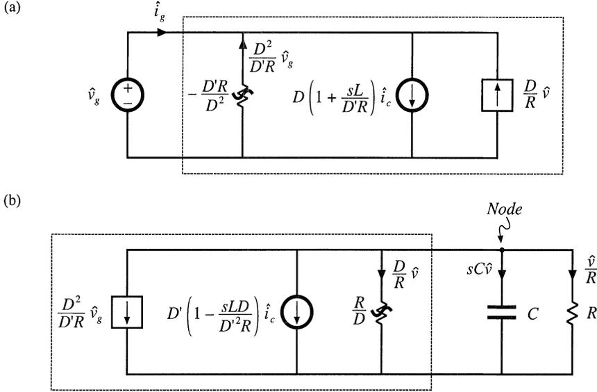
**Fig. 12.14** Construction of CPM CCM buck–boost converter equivalent circuit: (a) input port model, corresponding to Eq. (12.38); (b) output port model, corresponding to Eq. (12.37).
