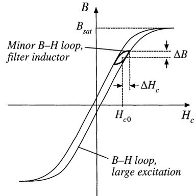
Fig. 13.42 Filter inductor minor B-H loop.
