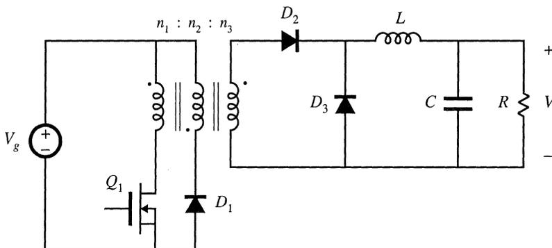
Fig. 6.22 Single-transistor forward converter.
