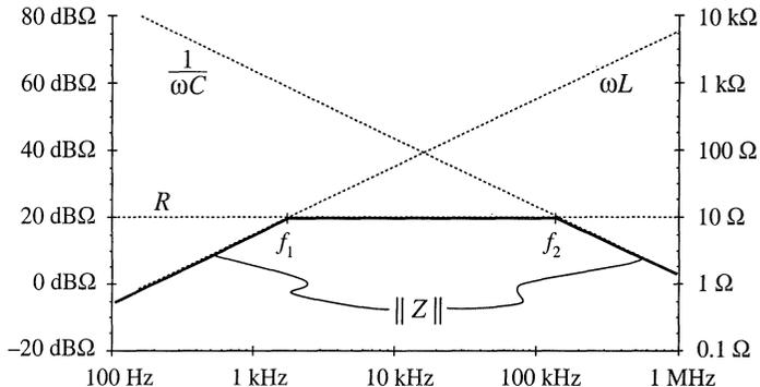
**Fig. 8.47** Graphical construction of impedance asymptotes for the parallel  $R$ - $L$ - $C$  example, with  $R$  increased to 1 k $\Omega$ .
