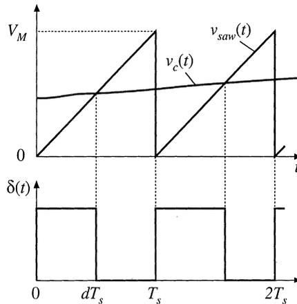
Fig. 7.64 Waveforms of the circuit of Fig. 7.63.
