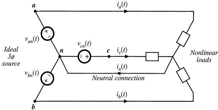
Fig. 16.9 Current flow in a three-phase four-wire network.
