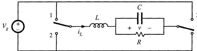
Fig. 2.30 H-bridge converter of Problems 2.4 and 2.6.
