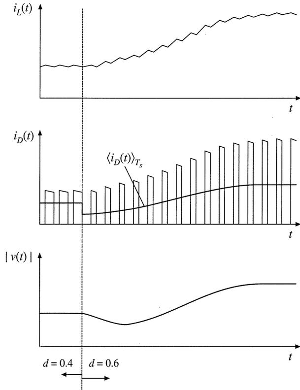
**Fig. 8.37** Waveforms of the converters of Fig. 8.36, for a step response in duty cycle. The average diode current and output voltage initially decrease, as predicted by the RHP zero. Eventually, the inductor current increases, causing the average diode current and the output voltage to increase.
