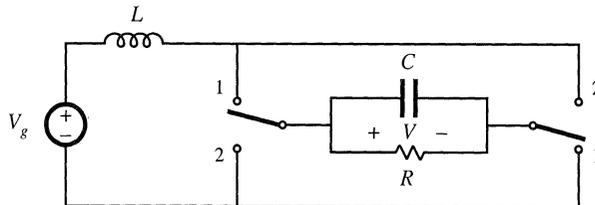
**Fig. 3.31** Nonideal current-fed bridge converter, Problems 3.3 and 3.4.
