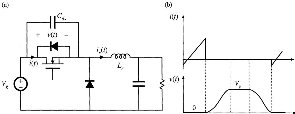
**Fig. 20.7** Zero-voltage switching of a MOSFET, ZVS quasi-squarewave buck converter example. The MOSFET, its body diode, and its output capacitance  $C_{ds}$  are illustrated. (a) converter schematic, (b) MOSFET voltage and current waveforms.
