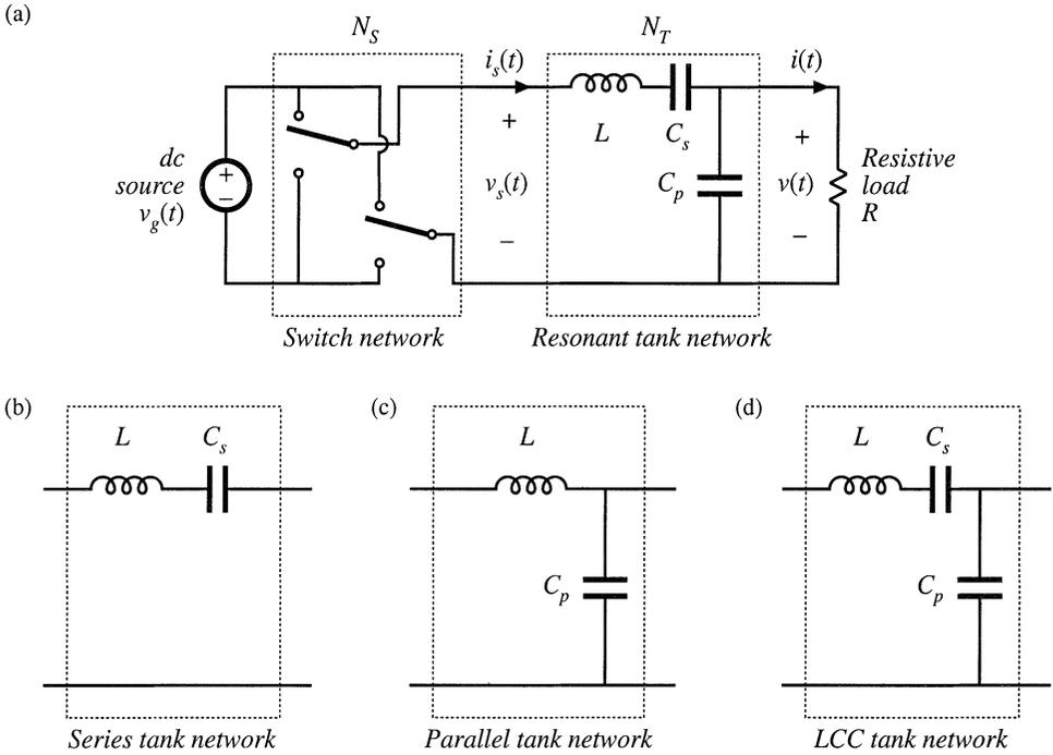
**Fig. 19.1** A basic class of resonant inverters that consist of (a) a switch network  $N_S$  that drives a resonant tank network  $N_T$  near resonance. Several common tank networks: (b) series, (c) parallel, (d) LCC.
