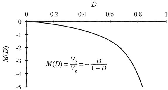
**Fig. 2.23** Dc conversion ratio  $M(D) = -V/V_g$  of the Ćuk converter.
