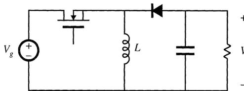
**Fig. 3.30** Nonideal buck–boost converter, Problems 3.1 and 3.2.
