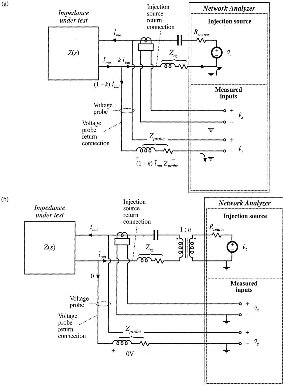
**Fig. 8.61** Measurement of a small impedance  $Z(s)$ : (a) current flowing in the return connection of the voltage probe induces a voltage drop that corrupts the measurement; (b) an improved experiment, incorporating isolation of the injection source.
