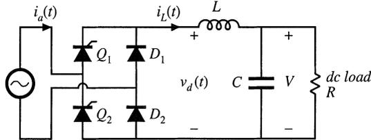
Fig. 17.28 Half-controlled rectifier circuit of Problem 17.1.
