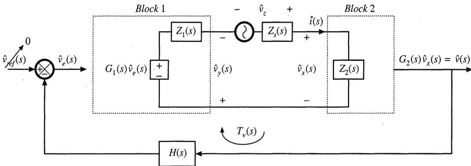
Fig. 9.35 Measurement of loop gain by voltage injection.
