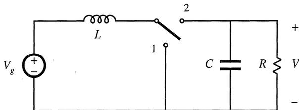
Fig. 1.12 The boost converter: (a) ideal converter circuit, (b) output voltage  $V$  vs. transistor duty cycle  $D$ .
