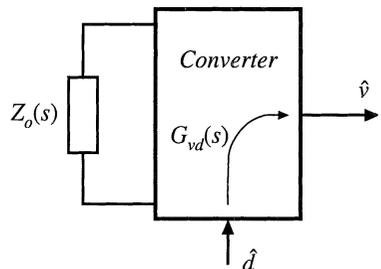
Fig. C.18 Determination of the control-to-output transfer function  $G_{vd}(s)$  for the system of Fig. C.17.
