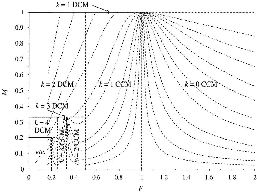
Fig. 19.46 Continuous and discontinuous conduction mode boundaries.
