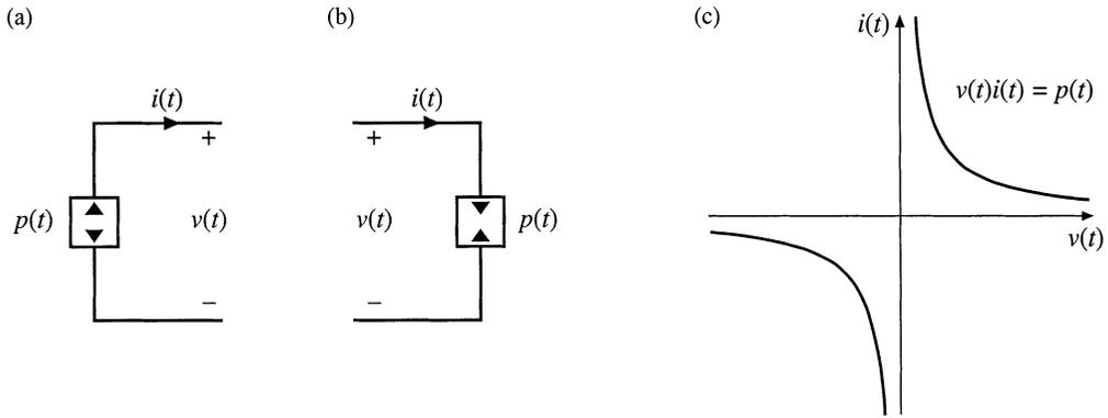
**Fig. 18.2** The dependent power source: (a) power source schematic symbol, (b) power sink schematic symbol, (c)  $i$ - $v$  characteristic.
