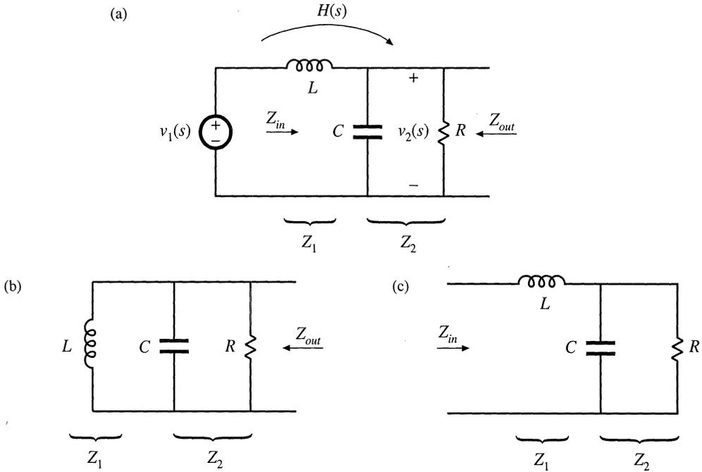
**Fig. 8.50** Two-pole low-pass filter based on voltage divider circuit: (a) transfer function  $H(s)$ , (b) determination of  $Z_{out}$ , by setting independent sources to zero, (c) determination of  $Z_{in}(s)$ .
