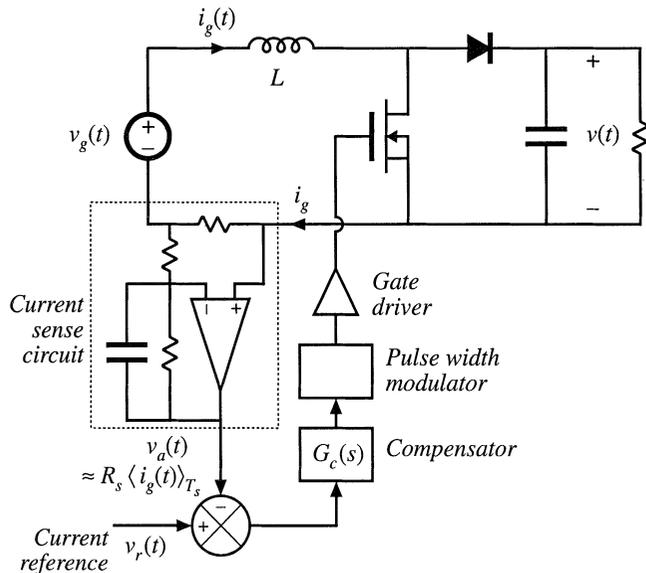
Fig. 18.10 Average current control of the input current in a boost converter.
