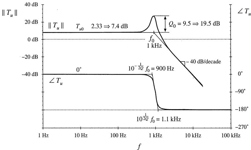
Fig. 9.26 Uncompensated loop gain  $T_u$ , design example.
