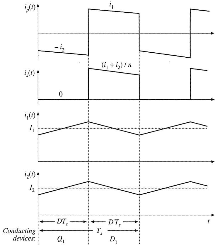
**Fig. 6.38** Waveforms of the isolated SEPIC, continuous conduction mode.
