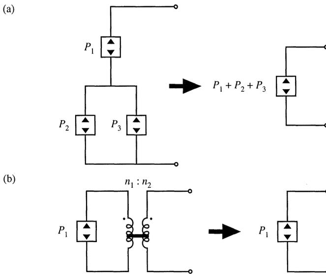
Fig. 11.6 Circuit manipulations of power source elements: (a) combination of series- and parallel- connected power sources into a single equivalent power source, (b) invariance of the power source to reflection through an ideal transformer of arbitrary turns ratio.
