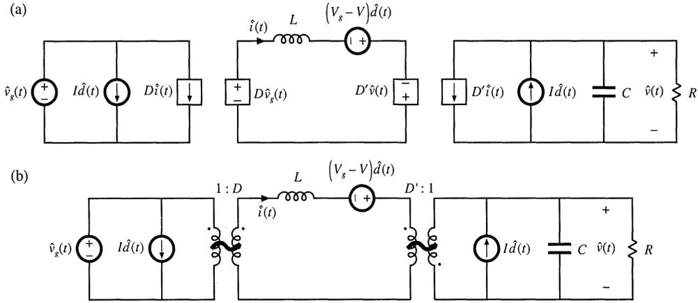
**Fig. 7.16** Buck-boost converter small-signal ac equivalent circuit: (a) the circuits of Figs. 7.13 to 7.15, collected together; (b) combination of dependent sources into effective ideal transformer, leading to the final model.
