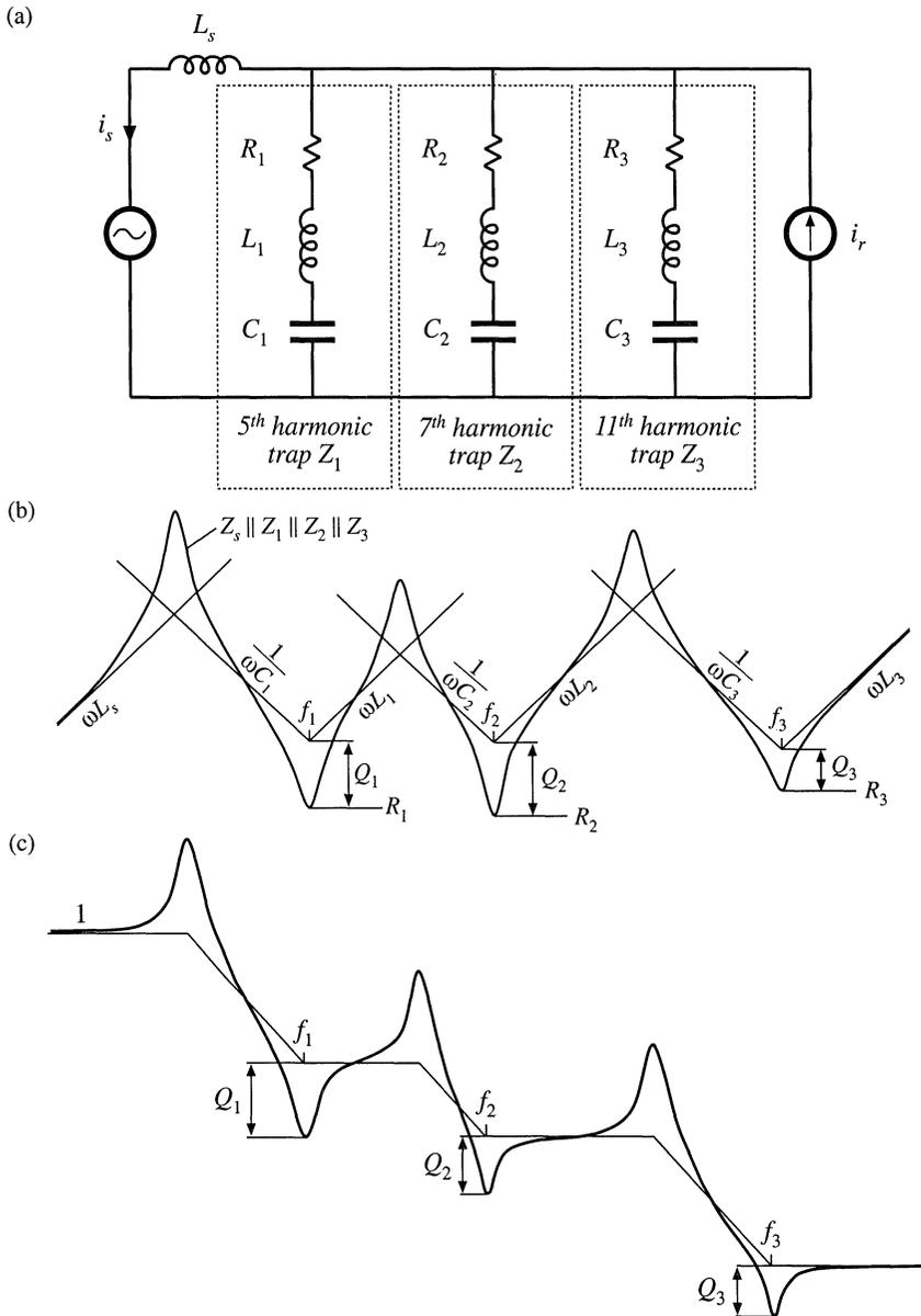
**Fig. 17.22** Construction of approximate frequency response for a harmonic trap filter that attenuates the fifth, seventh, and eleventh harmonics: (a) impedance asymptotes, (b) transfer function asymptotes.
