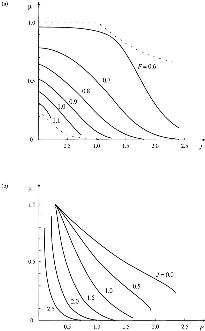
**Fig. 20.27** Conversion ratio  $\mu$  for the multi-resonant switch with  $C_d = 3C_s$ : (a) conversion ratio  $\mu$  vs. normalized current  $J$  (solid lines: conversion ratio; dashed lines: boundaries of zero-voltage switching), (b) conversion ratio  $\mu$  vs. normalized switching frequency  $F$ .
