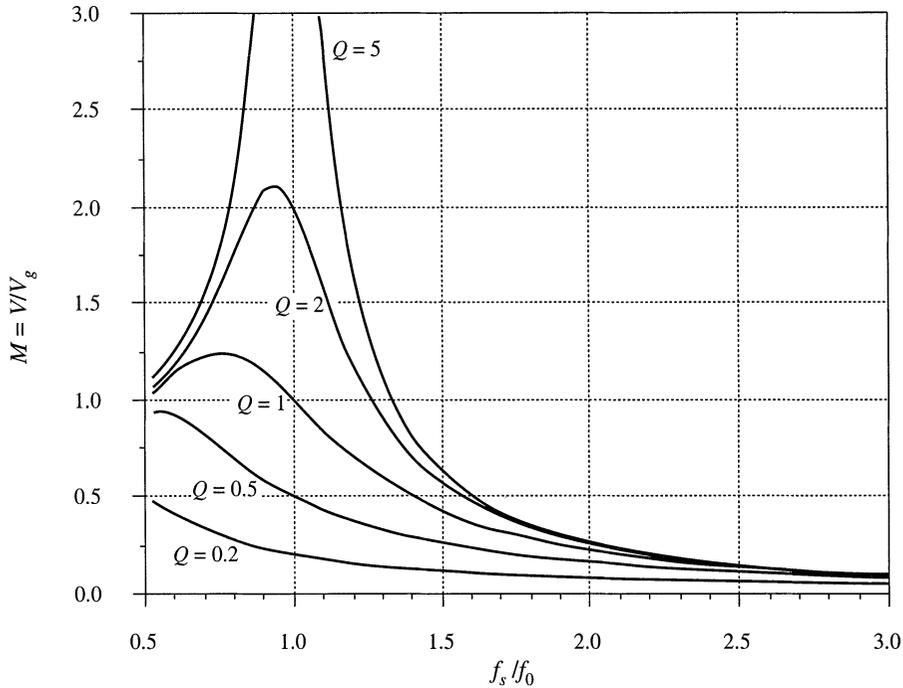
**Fig. 19.52** Exact control characteristics of the parallel resonant converter, with a resistive load. Both CCM and DCM operation is included, for  $0.5 \leq F \leq 3$ .
