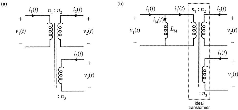
**Fig. 6.16** Simplified model of a multiple-winding transformer: (a) schematic symbol, (b) equivalent circuit containing a magnetizing inductance and ideal transformer.
