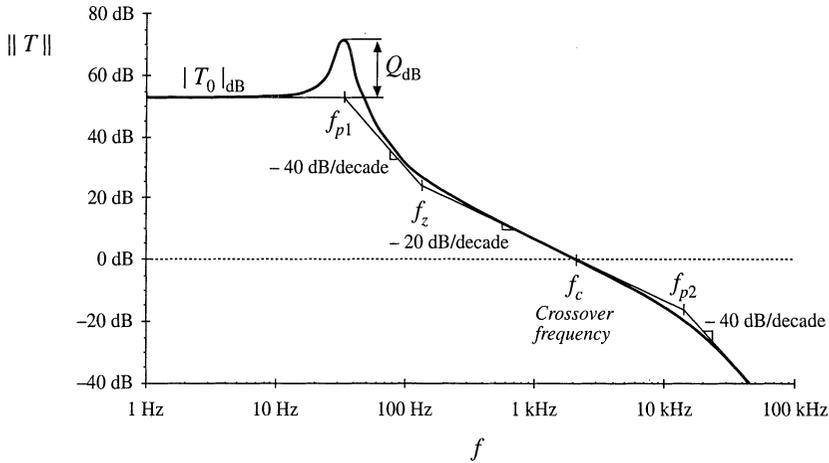
**Fig. 9.5** Magnitude of the loop gain example, Eq. (9.10).
