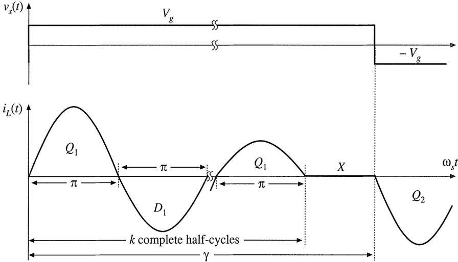
**Fig. 19.42** Tank inductor current waveform, type  $k$  DCM, for odd  $k$ . normally purposely designed to operate in odd discontinuous conduction modes, because the output voltage is not controllable. Nonetheless, when the load is removed with  $f_s < f_0$ , the series resonant converter operates in  $k = 1$  DCM with  $M = 1$ .
