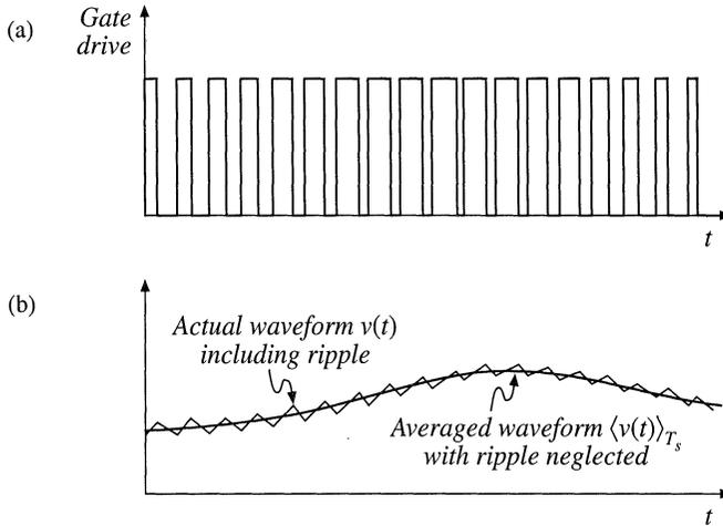
**Fig. 7.2** Ac variation of the converter signals: (a) transistor gate drive signal, in which the duty cycle varies slowly, and (b) the resulting converter output voltage waveform. Both the actual waveform  $v(t)$  (including high frequency switching ripple) and its averaged, low-frequency component,  $\langle v(t) \rangle_{T_s}$ , are illustrated.
