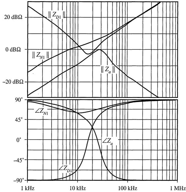
**Fig. 10.26** Bode plot of  $Z_{N1}$  and  $Z_{D1}$  for filter section 1. Also shown is the Bode plot for the output impedance  $Z_a$  of filter section 2.
