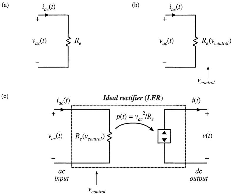
**Fig. 18.1** Development of the ideal rectifier equivalent circuit model: (a) input port resistor emulation; (b) the value of the emulated resistance, and hence the power throughput, is controllable; (c) output port power source characteristic, and complete model.
