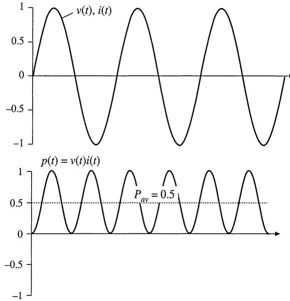
**Fig. 16.3** Voltage, current, and instantaneous power waveforms, example 2. The voltage and current each contain only third harmonic, and are in phase. Net energy is transmitted at the third harmonic frequency.
