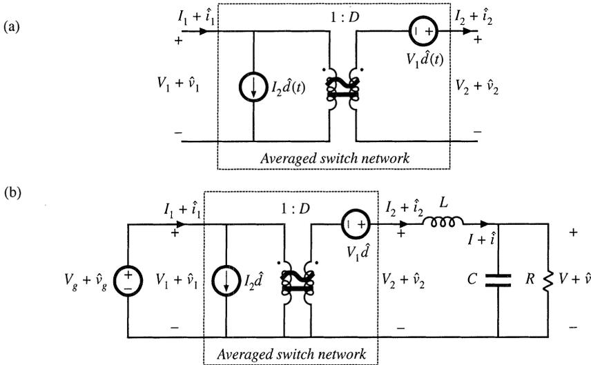
**Fig. 7.49** Averaged switch modeling, buck converter example: (a) dc and small-signal ac averaged switch model; (b) Averaged circuit model of the buck converter obtained by replacement of the switch network by the averaged switch model.
