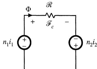
The MMF generators are additive, because the currents  $i_1$  and  $i_2$  pass in the same direction through the core window. Solution of Fig. 13.14 yields
