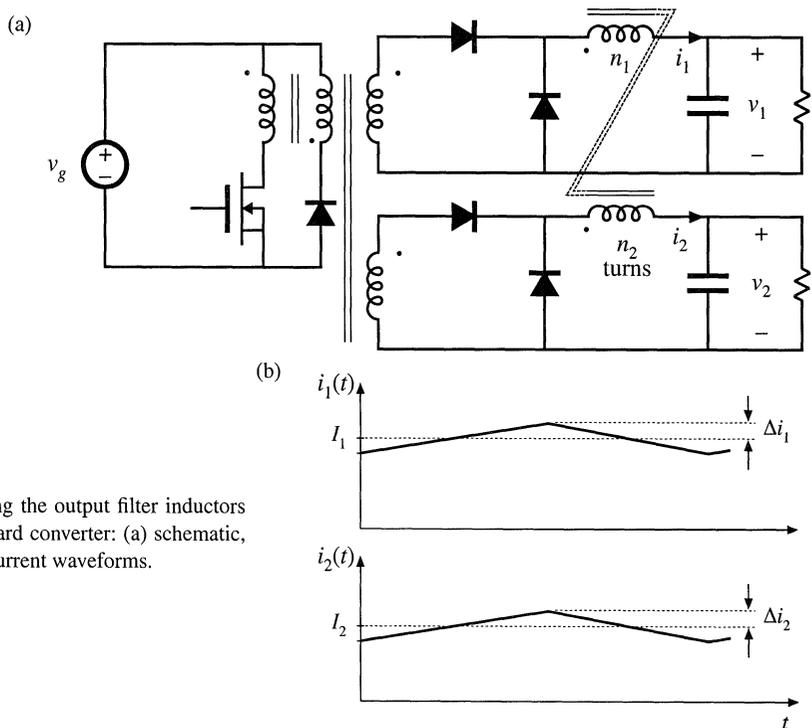
**Fig. 13.47** Coupling the output filter inductors of a two-output forward converter: (a) schematic, (b) typical inductor current waveforms.
