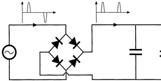
Fig. 16.6 Conventional peak detection rectifier.
