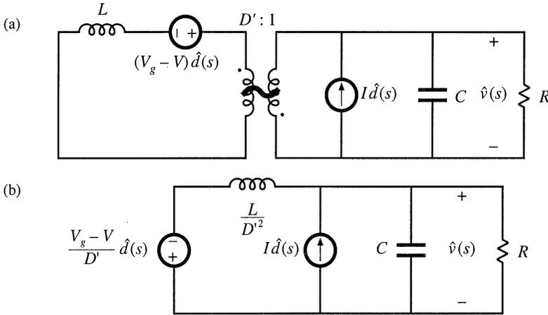
**Fig. 8.31** Manipulation of buck-boost equivalent circuit to find the control-to-output transfer function  $G_{vd}(s)$ : (a) set  $\hat{v}_g$  source to zero; (b) push inductor and voltage source through transformer.
