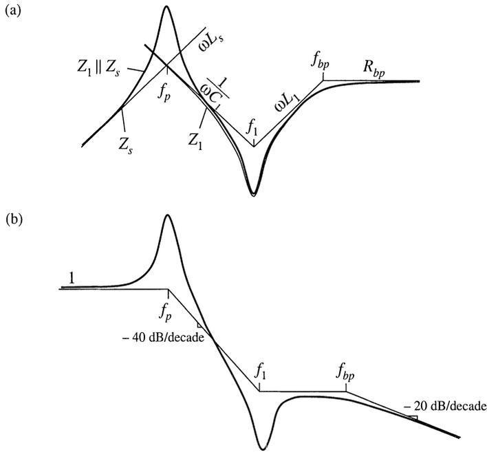
**Fig. 17.24** Construction of approximate frequency response for a harmonic trap filter containing bypass resistor: (a) impedance asymptotes, (b) transfer function asymptotes.
