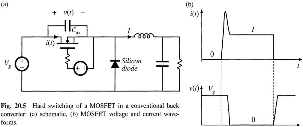
**Fig. 20.5** Hard switching of a MOSFET in a conventional buck converter: (a) schematic, (b) MOSFET voltage and current waveforms.
