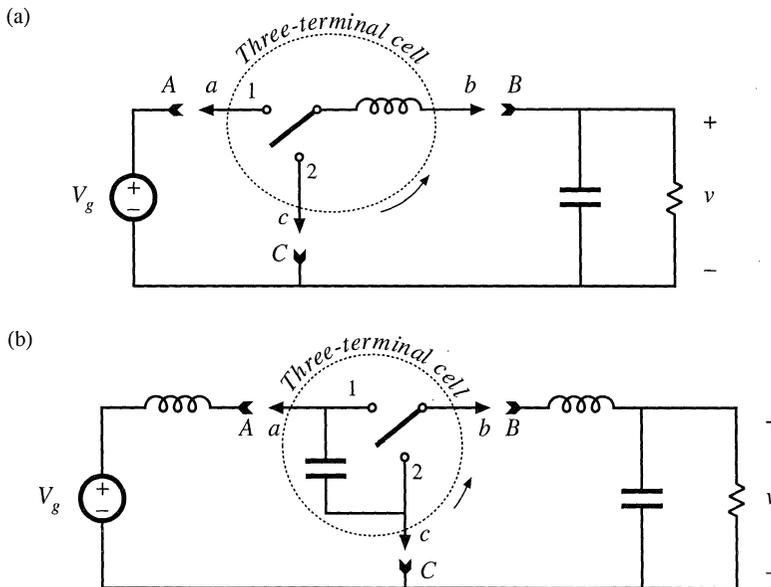
**Fig. 6.9** Rotation of three-terminal switch cells: (a) switch/inductor cell, (b) switch/capacitor cell.
