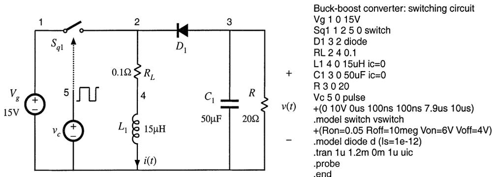
Fig. B.7 Buck-boost converter simulation example, switching circuit model.
