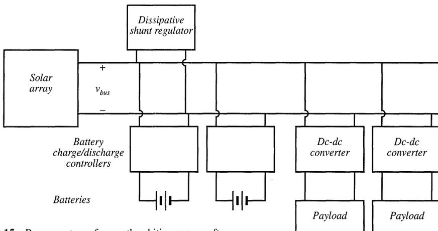
Fig. 1.15 Power system of an earth-orbiting spacecraft.
