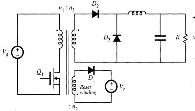
Fig. 6.45 Forward converter with auxiliary reset winding, Problem 6.9
