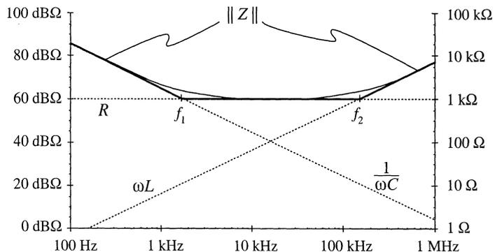
Fig. 8.42 Graphical construction of  $\|Z\|$  of the series  $R-L-C$  network of Fig. 8.41, for the element values specified by Eq. (8.143).
