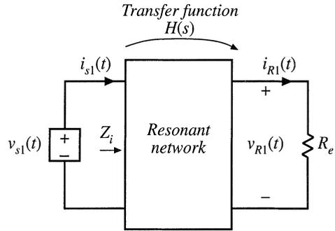
**Fig. 19.13** The linear tank network, excited by an effective sinusoidal input source and driving an effective resistive load.
