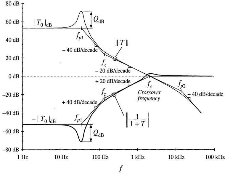
**Fig. 9.7** Graphical construction of  $\| 1/(1 + T) \|$ .
