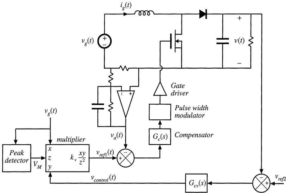
Fig. 18.14 Average current control incorporating input voltage feedforward.
