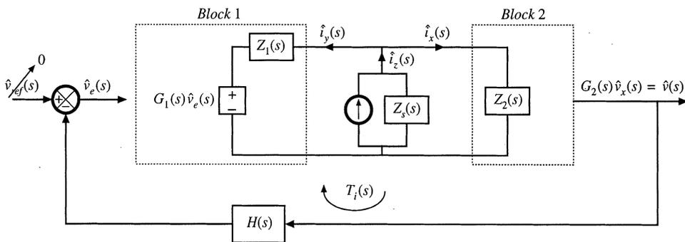
Fig. 9.38 Measurement of loop gain by current injection.
