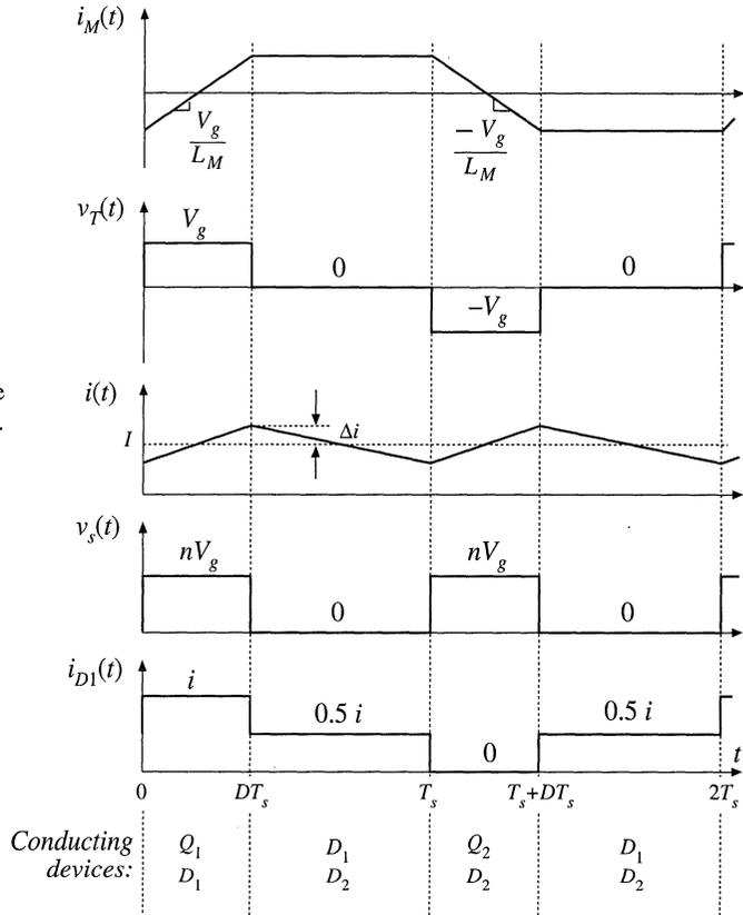
Fig. 6.29 Waveforms of the push-pull isolated buck converter.
