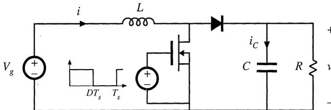
**Fig. 3.22** Boost converter example.
