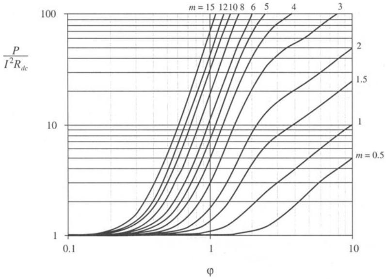
**Fig. 13.31** Increase of layer copper loss due to the proximity effect, as a function of  $\phi$  and MMF ratio  $m$ , for sinusoidal excitation.
