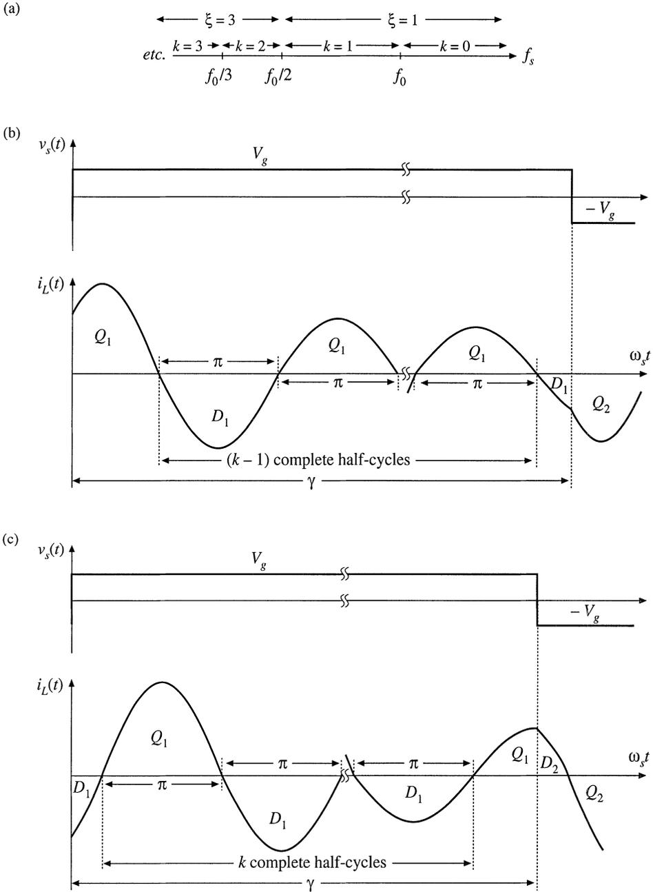
**Fig. 19.41** Continuous conduction modes of the series resonant converter: (a) switching frequency ranges over which various mode indices  $k$  and subharmonic numbers  $\xi$  occur; (b) tank inductor current waveform, type  $k$  CCM, for odd  $k$ ; (c) tank inductor current waveform, type  $k$  CCM, for even  $k$ .
