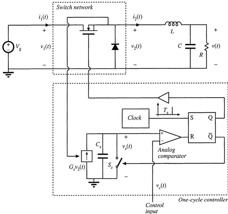
Fig. 12.38 Buck converter with one-cycle controller, Problem 12.12.
