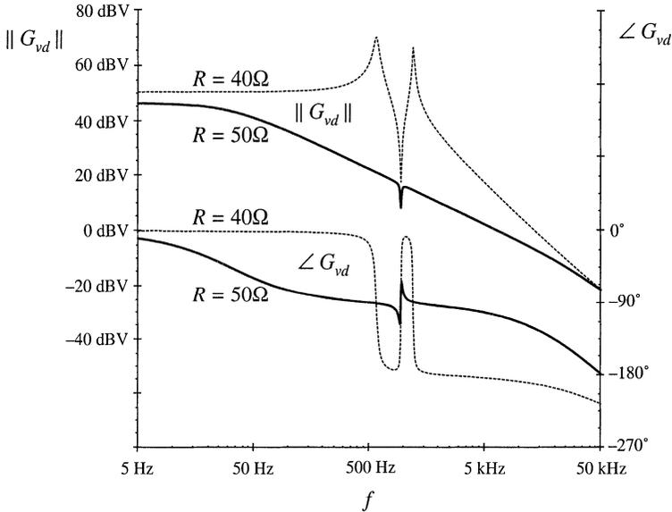
Fig. 11.21 Magnitude and phase of the control-to-output transfer function obtained by simulation of the SEPIC example shown in Fig. 11.20, for two values of the load resistance:  $R = 50\Omega$  when the converter operates in DCM (solid lines), and  $R = 40\Omega$  for which the converter operates in CCM (dashed lines).
