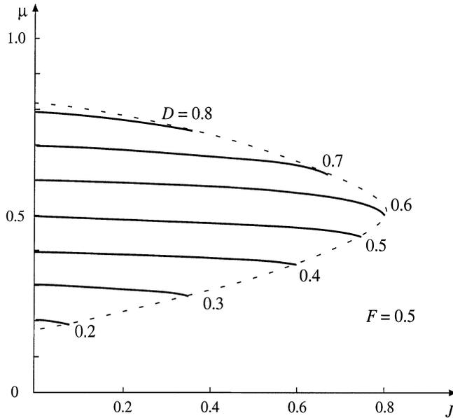
**Fig. 20.35** Conversion ratio  $\mu$ , as a function of duty cycle  $D$  and normalized load current  $J$ , for the two-switch QSW-ZVS switch illustrated in Fig. 20.33. Curves are plotted for constant-frequency control with  $F = 0.5$ . The dashed line is the zero-voltage switching boundary.
