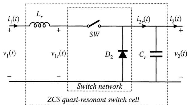
Fig. 20.20 Basic ZCS quasi-resonant switch cell.
