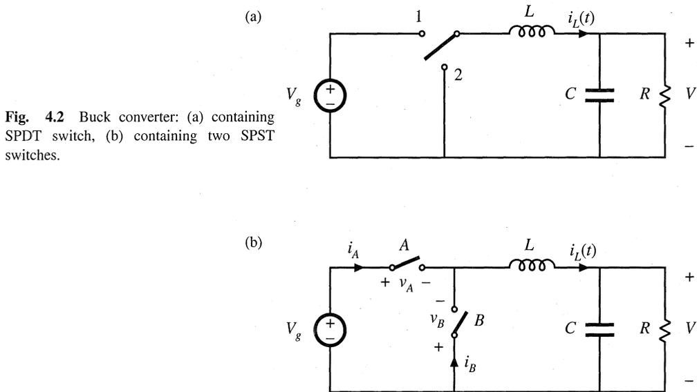
**Fig. 4.2** Buck converter: (a) containing SPDT switch, (b) containing two SPST switches.
