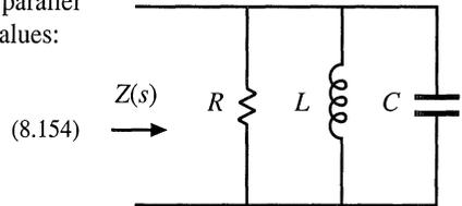
Impedance magnitudes of the individual elements are illustrated in Fig. 8.45. The asymptotes for the total parallel impedance  $Z$  are approximated by simply selecting the smallest individual element impedance, as shown by the heavy line in Fig. 8.46. So the parallel impedance is dominated by the inductor at low frequency, by the resistor at mid frequencies, and by the capacitor at high frequency. Approximate expressions for the angular corner frequencies are again found by equating asymptotes:
