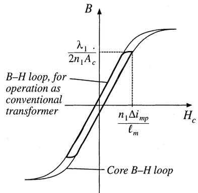
**Fig. 13.46** Operational  $B$ - $H$  loop of a conventional transformer.
