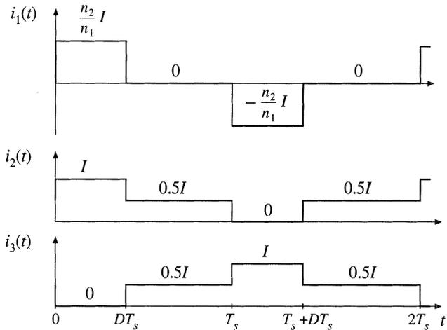
**Fig. 14.10** Transformer waveforms, PWM full-bridge converter example.
