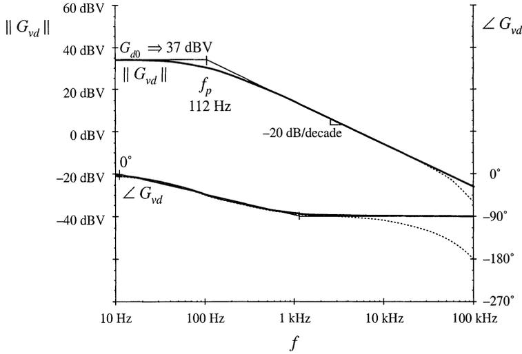
**Fig. 11.19** Magnitude and phase of the control-to-output transfer function, DCM boost example. Solid lines: function and its asymptotes, approximate single-pole response predicted by the model of Fig. 11.18. Dashed lines: more accurate response that includes high-frequency inductor dynamics.
