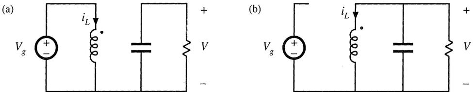
**Fig. 6.7** Reversal of the output voltage polarity, by reversing the inductor connections while the switches are in position 2: (a) connections with the switches in position 1, (b) connections with the switches in position 2.
