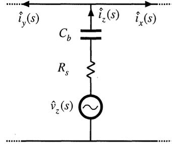
**Fig. 9.39** Current injection using Thevenin-equivalent source.
