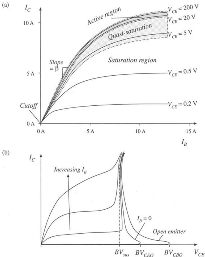
**Fig. 4.35** BJT static characteristics: (a)  $I_C$  vs.  $I_B$ , illustrating the regions of operation; (b)  $I_C$  vs.  $V_{CE}$ , illustrating voltage breakdown characteristics.
