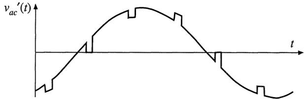
essentially only the power system source impedance, then commutation causes significant notching of the ac voltage waveforms (Fig. 17.18) at the point of common coupling of the rectifier to the power system. Other elements connected locally to the power system will experience voltage distortion. Limits for the areas of these notches are suggested in IEEE/ANSI standard 519.
