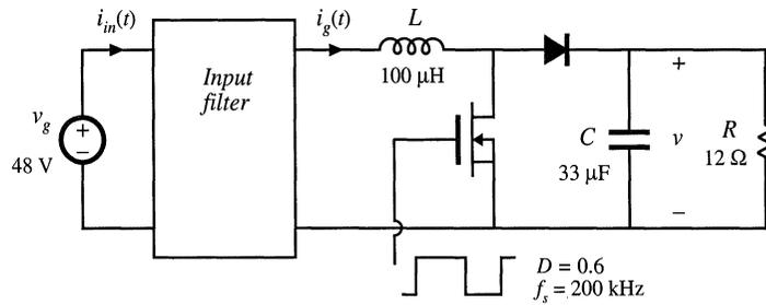
**Fig. 10.31** Boost converter, Problems 10.2, 10.5, 10.7, and 10.9.
