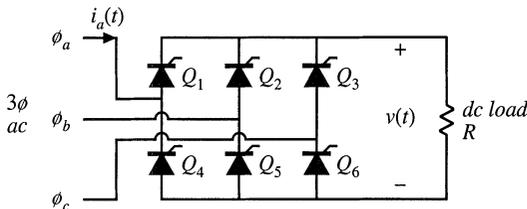
Fig. 17.30 Three-phase controlled rectifier circuit of Problem 17.3.
