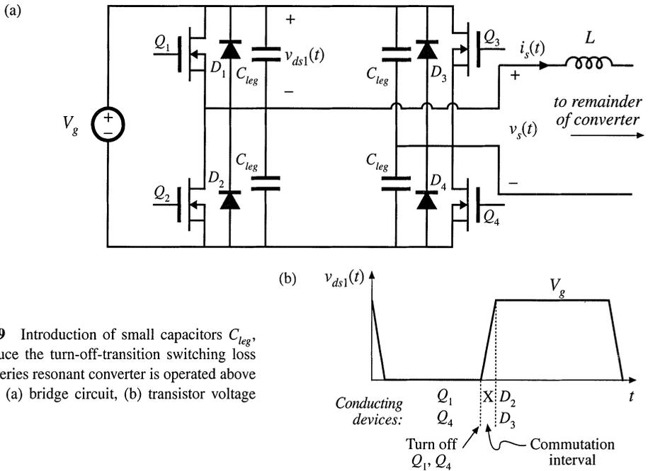
**Fig. 19.29** Introduction of small capacitors  $C_{leg}$ , which reduce the turn-off-transition switching loss when the series resonant converter is operated above resonance: (a) bridge circuit, (b) transistor voltage waveform.
