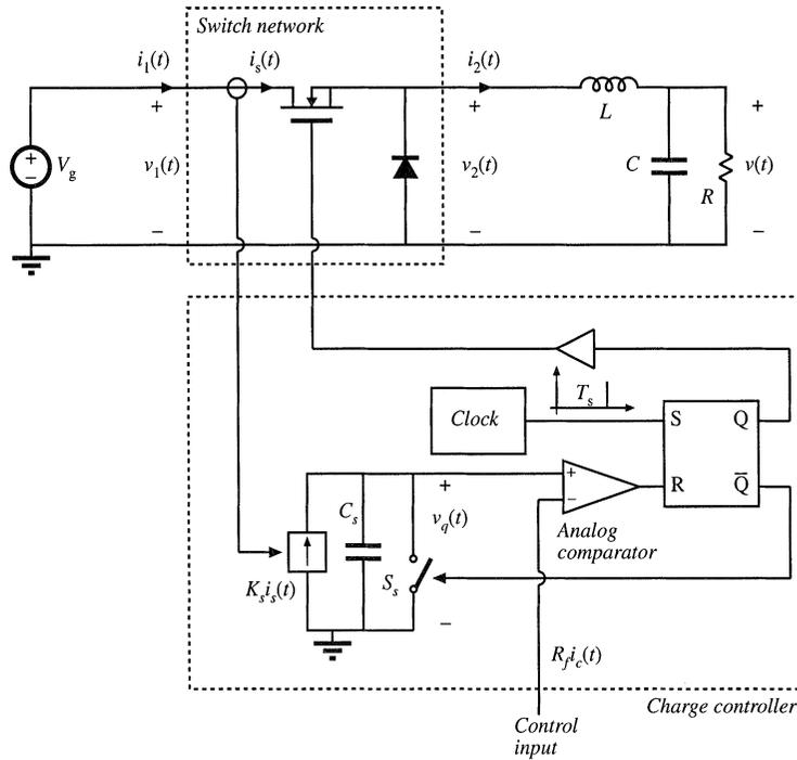
Fig. 12.37 Buck converter with charge controller, Problem 12.11.
