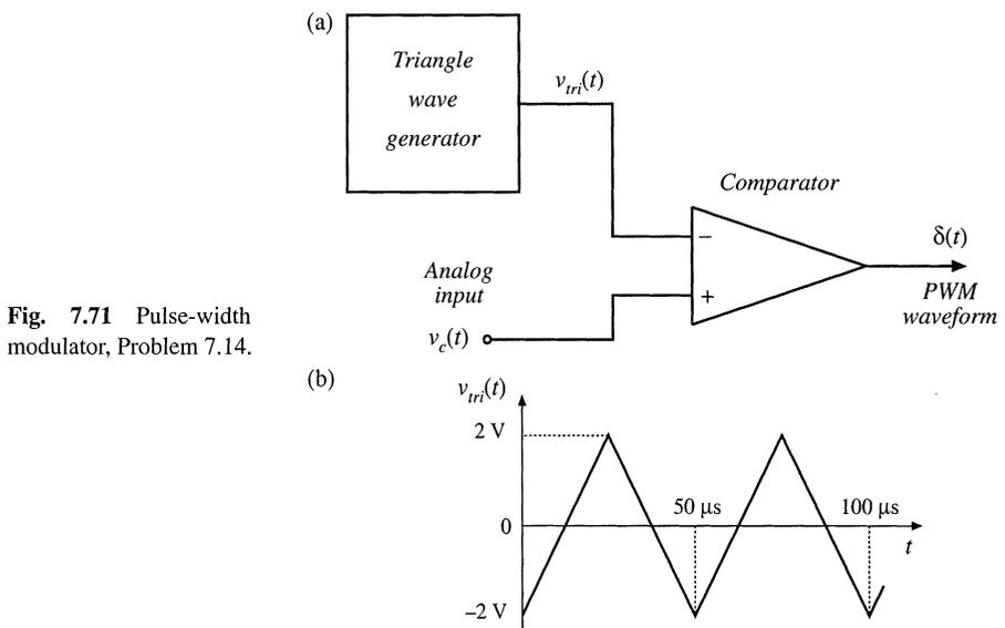
**Fig. 7.71** Pulse-width modulator, Problem 7.14.
