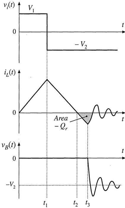
Fig. 4.54 Waveforms of the circuit of Fig. 4.53.
