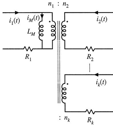
Fig. 15.4 Computed elements of simple transformer model.
