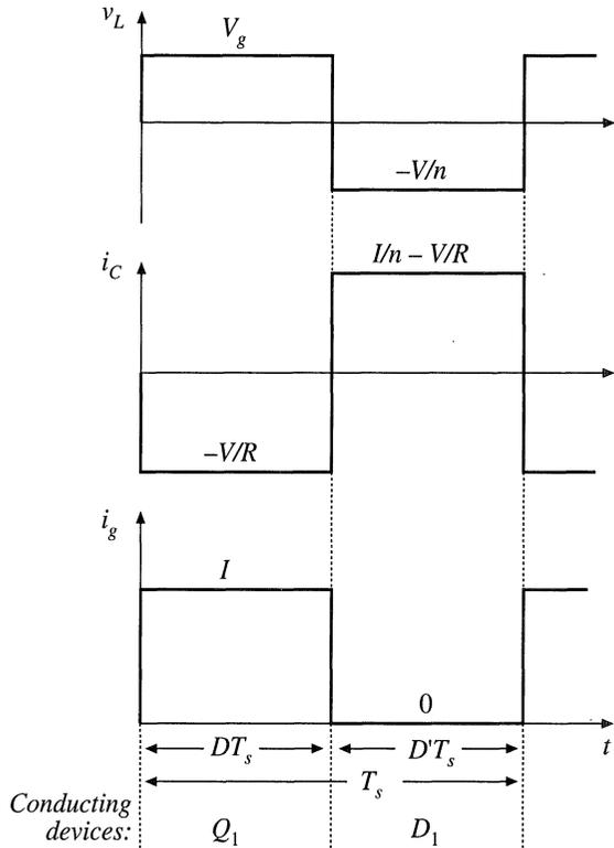
**Fig. 6.32** Flyback converter waveforms, continuous conduction mode.
