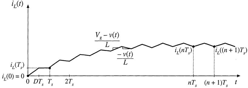
**Fig. 2.11** Inductor current waveform during converter turn-on transient.
