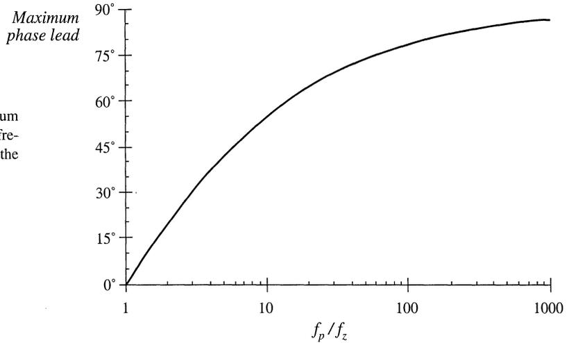
**Fig. 9.16** Maximum phase lead  $\theta$  vs. frequency ratio  $f_p/f_z$  for the lead compensator.
