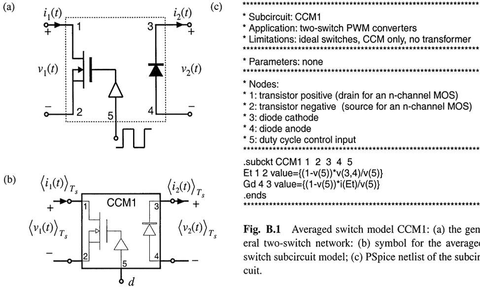
**Fig. B.1** Averaged switch model CCM1: (a) the general two-switch network; (b) symbol for the averaged switch subcircuit model; (c) PSpice netlist of the subcircuit.
