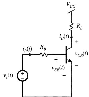
**Fig. 4.31** Circuit for BJT switching time example.
