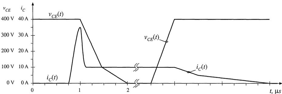
Fig. 4.57 IGBT voltage and current waveforms, Problem 4.7.
