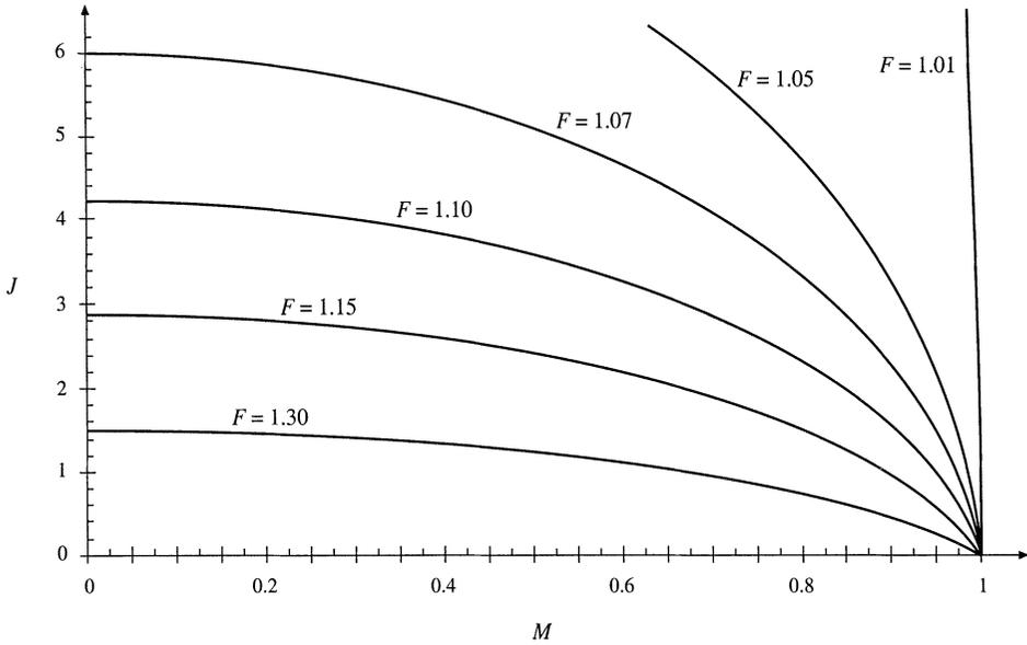
**Fig. 19.47** Output characteristics,  $k = 0$  CCM (above resonance).
