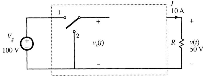
**Fig. 1.8** Insertion of SPDT switch which changes the dc component of the voltage.
