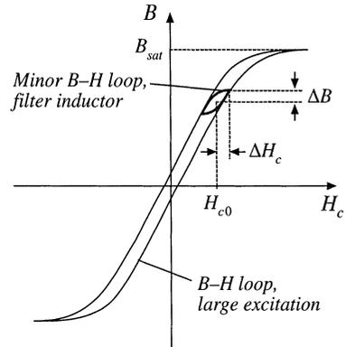
Fig. 13.42 Filter inductor minor B-H loop.
