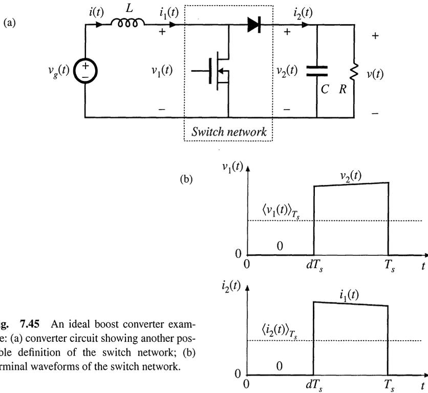
**Fig. 7.45** An ideal boost converter example: (a) converter circuit showing another possible definition of the switch network; (b) terminal waveforms of the switch network.
