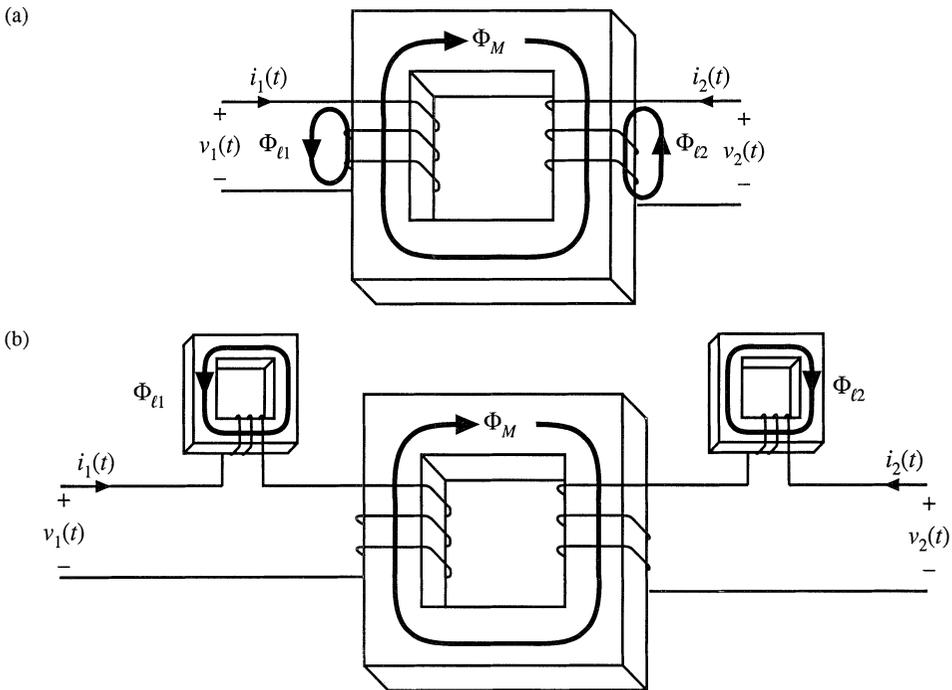
Fig. 13.17 Leakage flux in a two-winding transformer: (a) transformer geometry, (b) an equivalent system.
