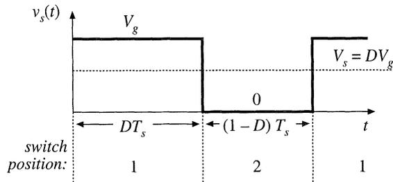
**Fig. 1.9** Switch output voltage waveform  $v_s(t)$ .
