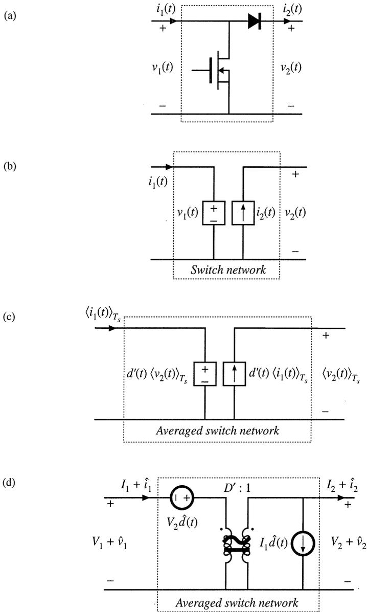
**Fig. 7.46** Derivation of the averaged switch model for the CCM boost of Fig. 7.45: (a) switch network; (b) switch network where the switches are replaced by dependent sources whose waveforms match the switch terminal waveforms; (c) large-signal, nonlinear averaged switch model obtained by averaging the switch network terminal waveforms; (d) dc and ac small-signal averaged switch network model.
