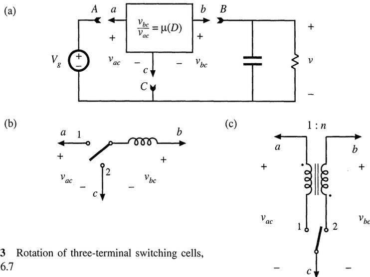
Fig. 6.43 Rotation of three-terminal switching cells, Problem 6.7
