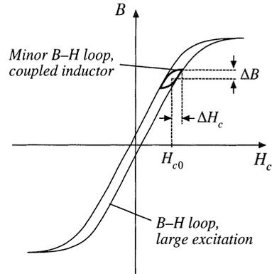
Fig. 13.48 Coupled inductor minor  $B$ - $H$  loop.
