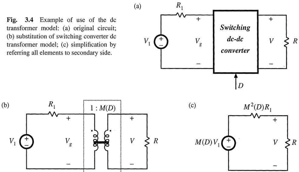
**Fig. 3.4** Example of use of the dc transformer model: (a) original circuit; (b) substitution of switching converter dc transformer model; (c) simplification by referring all elements to secondary side.
