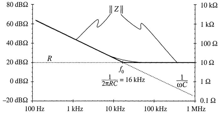
**Fig. 8.40** Construction of the composite asymptotes of  $\| Z \|$ . The asymptotes of the series combination can be approximated by simply selecting the larger of the individual resistor and capacitor asymptotes.
