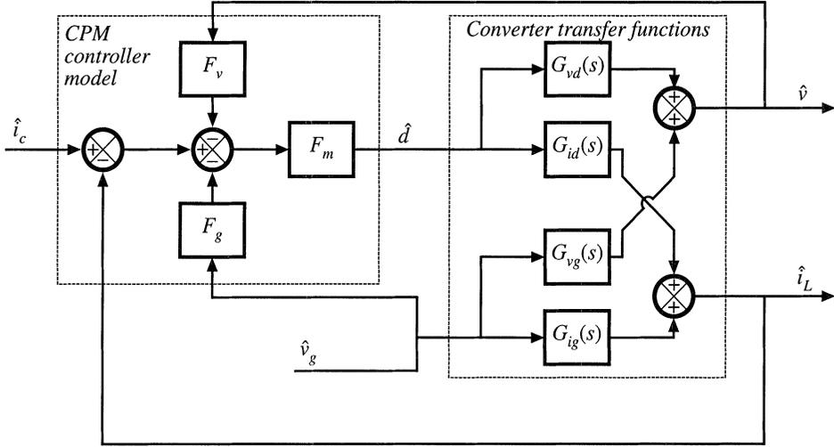
Fig. 12.26 Block diagram that models the current-programmed converters of Fig. 12.25.
