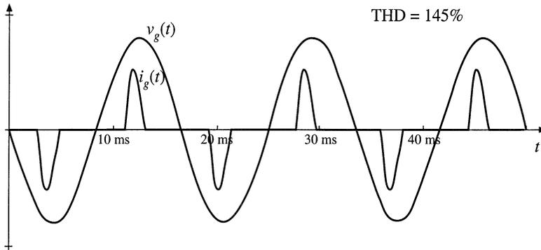
Fig. 17.3 Typical ac line current and voltage waveforms, discontinuous conduction mode.  $f_0/f_L = 8.4$ ,  $Q = 121$ .
