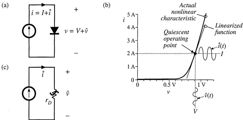
**Fig. 7.4** Small-signal equivalent circuit modeling of the diode: (a) a nonlinear diode conducting current  $i$ ; (b) linearization of the diode characteristic around a quiescent operating point; (c) a linearized small-signal model.
