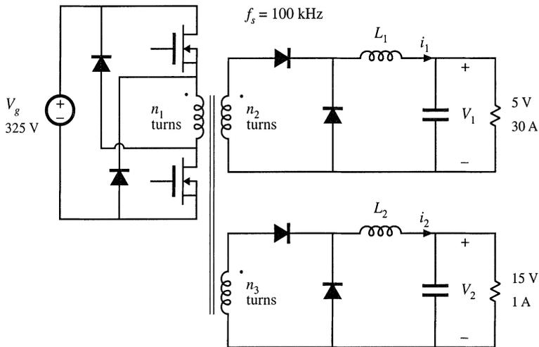
Fig. 15.11 Two-output forward converter of Problem 15.1.
