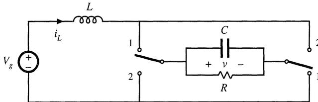
Fig. 2.31 Current-fed bridge converter of Problems 2.5, 2.7, and 2.8.
