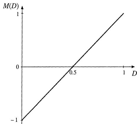
Fig. 6.12 Conversion ratio of the H-bridge inverter circuit.
