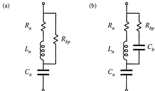
**Fig. 17.23** Addition of bypass resistor  $R_{bp}$  to a series resonant network, to obtain a high-frequency rolloff characteristic: (a) basic circuit, (b) addition of blocking capacitor  $C_b$  to reduce power consumption at the fundamental frequency.
