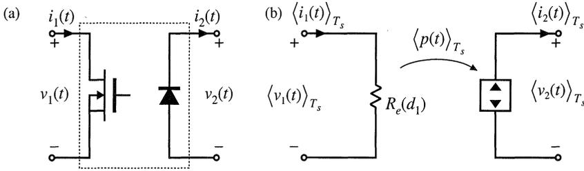
**Fig. 11.7** (a) the general two-switch network, and (b) the corresponding averaged switch model in the discontinuous conduction mode: the average transistor waveforms obey Ohm’s law, while the average diode waveforms behave as a dependent power source.
