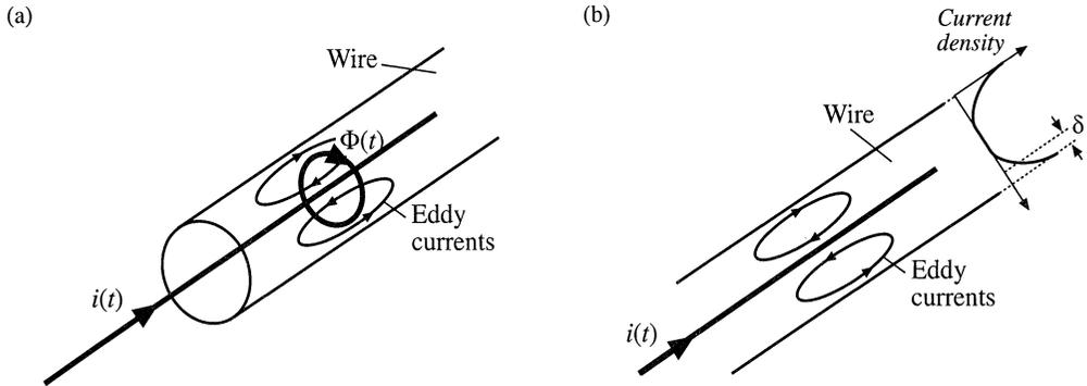
**Fig. 13.22** The skin effect: (a) current  $i(t)$  induces flux  $\Phi(t)$ , which in turn induces eddy currents in conductor; (b) the eddy currents tend to oppose the current  $i(t)$  in the center of the wire, and increase the current on the surface of the wire.
