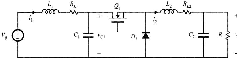
Fig. 3.33 Buck converter with input filter, Problem 3.6.
