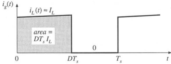
Fig. 3.19 Converter input port dc equivalent circuit.
