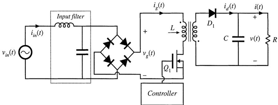
**Fig. 18.46** Low-harmonic rectifier system based on the CCM flyback converter, Problem 18.11.
