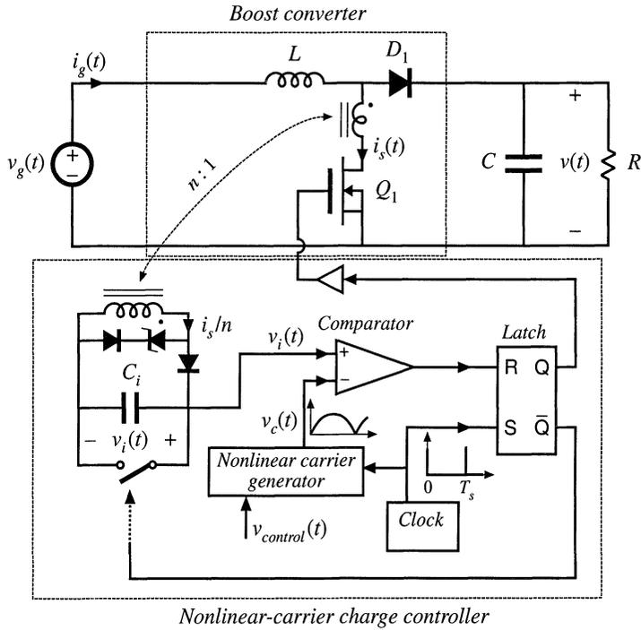
Fig. 18.21 Nonlinear-carrier charge control of a boost converter.
