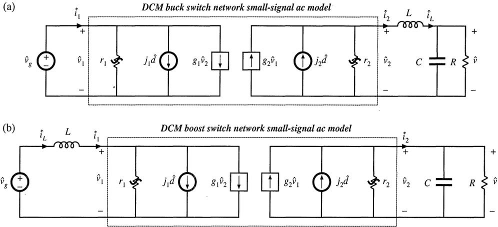
**Fig. 11.17** Small-signal ac models of (a) the DCM buck converter, and (b) the DCM boost converter, obtained by replacing the switch networks defined in Fig. 11.16(a) and (b) with the small-signal switch model of Fig. 11.16(c).
