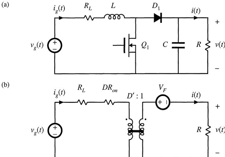
**Fig. 18.32** Dc–dc boost converter, (a), and a steady-state equivalent circuit, (b), which models the inductor resistance  $R_L$ , MOSFET on-resistance  $R_{on}$ , and diode forward voltage drop  $V_F$ .
