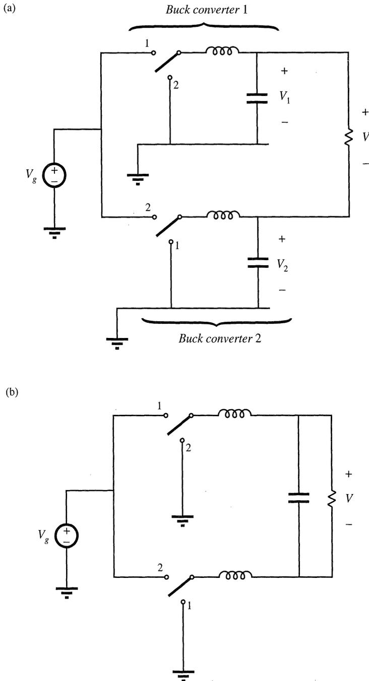
**Fig. 6.11** Derivation of bridge inverter (H-bridge): (a) differential connection of load across outputs of buck converters, (b) bypassing load by capacitor, (c) combining series inductors, (d) circuit (c) redrawn in its usual form.
