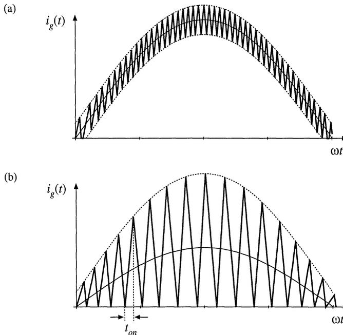
**Fig. 18.19** Input current waveforms of two boost converters with hysteretic control: (a)  $\pm 10\%$  regulation band, (b) critical conduction mode operation ( $\pm 100\%$  regulation band).
