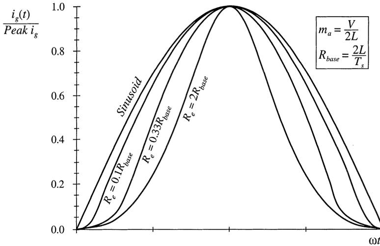
**Fig. 18.18** Input current waveshapes predicted by the static input characteristics of Fig. 18.17, compared with a pure sinusoid. Curves are plotted for the case  $V_M = 0.8V$ , with minimum stabilizing artificial ramp.
