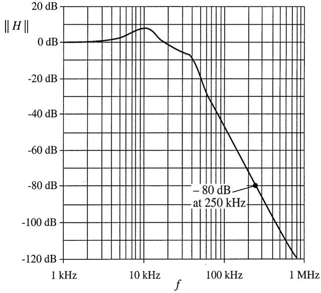
**Fig. 10.28** Input filter transfer function, cascaded two-section design.
