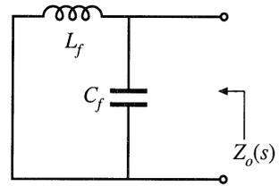
**Fig. 10.11** Determination of the filter output impedance  $Z_o(s)$ .
