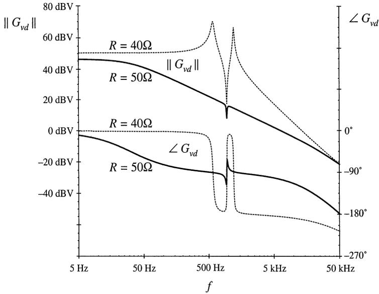
**Fig. B.14** Magnitude and phase responses of the control-to-output transfer function obtained by simulation of the SEPIC example, for two values of the load resistance. For  $R = 50 \Omega$ , the converter operates in DCM (solid lines), and for  $R = 40 \Omega$ , the converter operates in CCM (dotted lines).
