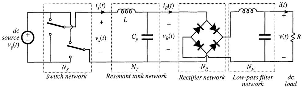
Fig. 19.19 Block diagram of the parallel resonant converter.
