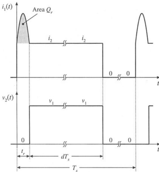
Fig. 7.55 Switch waveforms, buck converter switching loss example.
