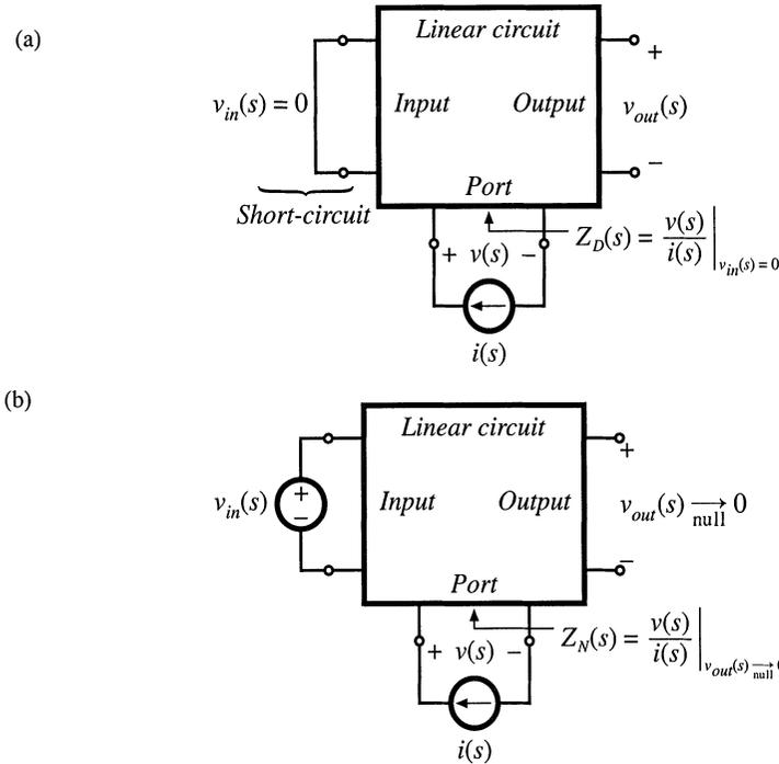
**Fig. C.3** Determination of the quantities  $Z_N(s)$  and  $Z_D(s)$ : (a)  $Z_D(s)$  is the Thevenin-equivalent impedance at the port, and is measured with the input  $v_{in}(s)$  set to zero; (b)  $Z_N(s)$  is the impedance seen at the port under the condition that the output is nulled.
