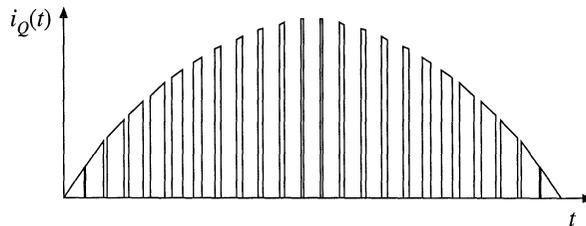
Fig. 18.31 Modulated transistor current waveform, boost rectifier.
