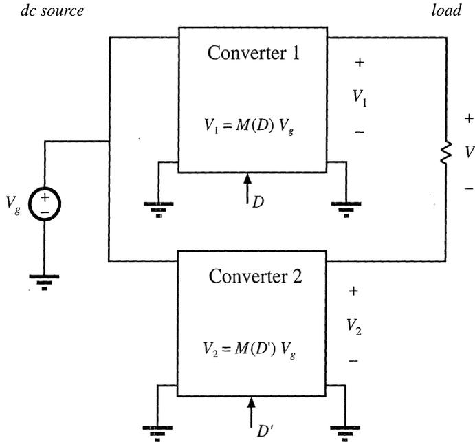
Fig. 6.10 Obtaining a bipolar output by differential connection of load.
