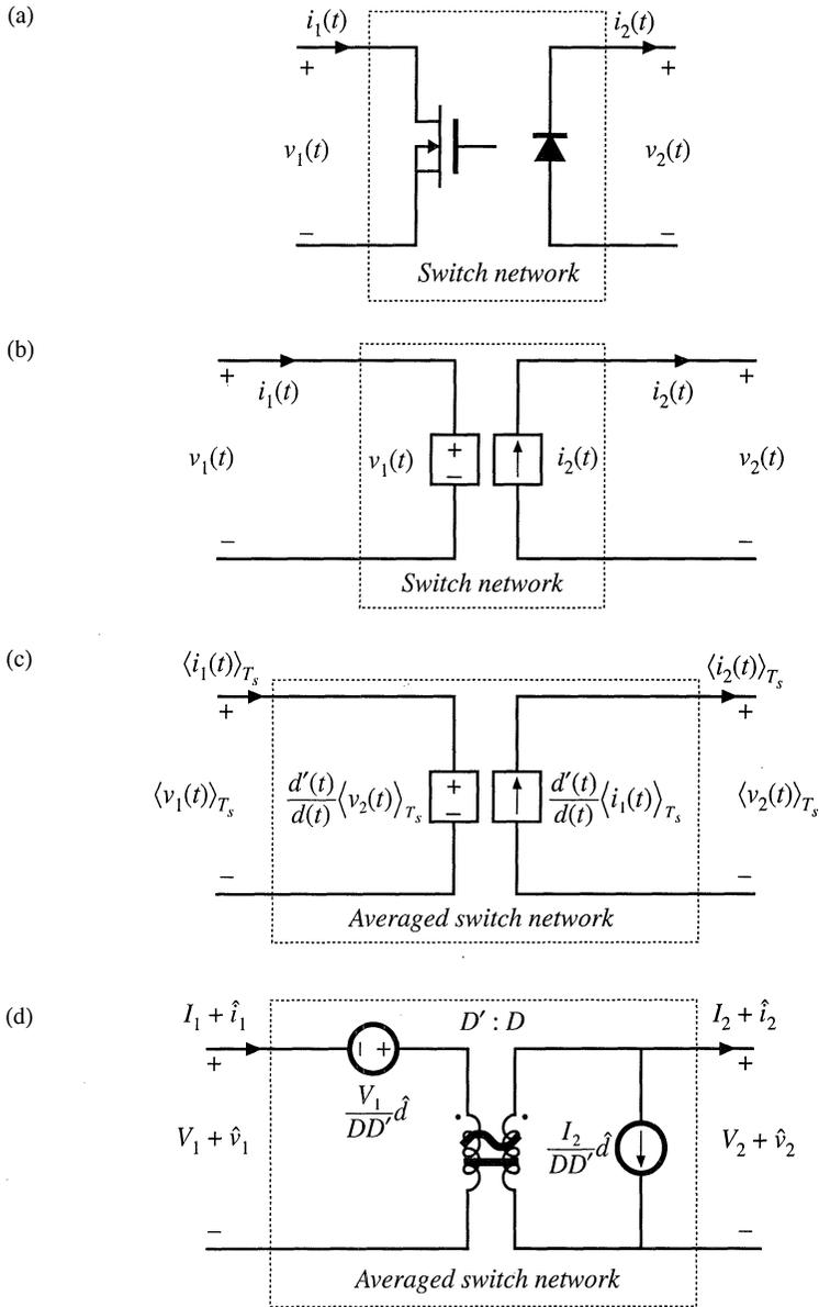
**Fig. 7.39** Derivation of the averaged switch model for the CCM SEPIC: (a) switch network; (b) switch network where the switches are replaced with dependent sources whose waveforms match the switch terminal dependent waveforms; (c) large-signal, nonlinear averaged switch model obtained by averaging the switch network terminal waveforms in (b); (d) dc and ac small-signal averaged switch model.
