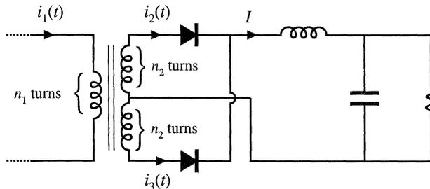
Fig. 14.9 PWM full-bridge transformer example.
