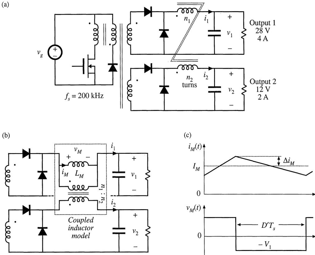
**Fig. 14.12** Two-output forward converter example: (a) circuit schematic, (b) coupled inductor model inserted into converter secondary-side circuit, (c) magnetizing current and voltage waveforms of coupled inductor, referred to winding 1.
