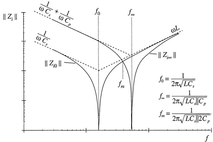
**Fig. 19.36** Variation of tank network input impedance  $\|Z_i\|$  with load resistance  $R$ , LCC inverter. As the load resistance is increased,  $\|Z_i\|$  changes monotonically from  $\|Z_{i0}\|$  to  $\|Z_{i\infty}\|$ .
