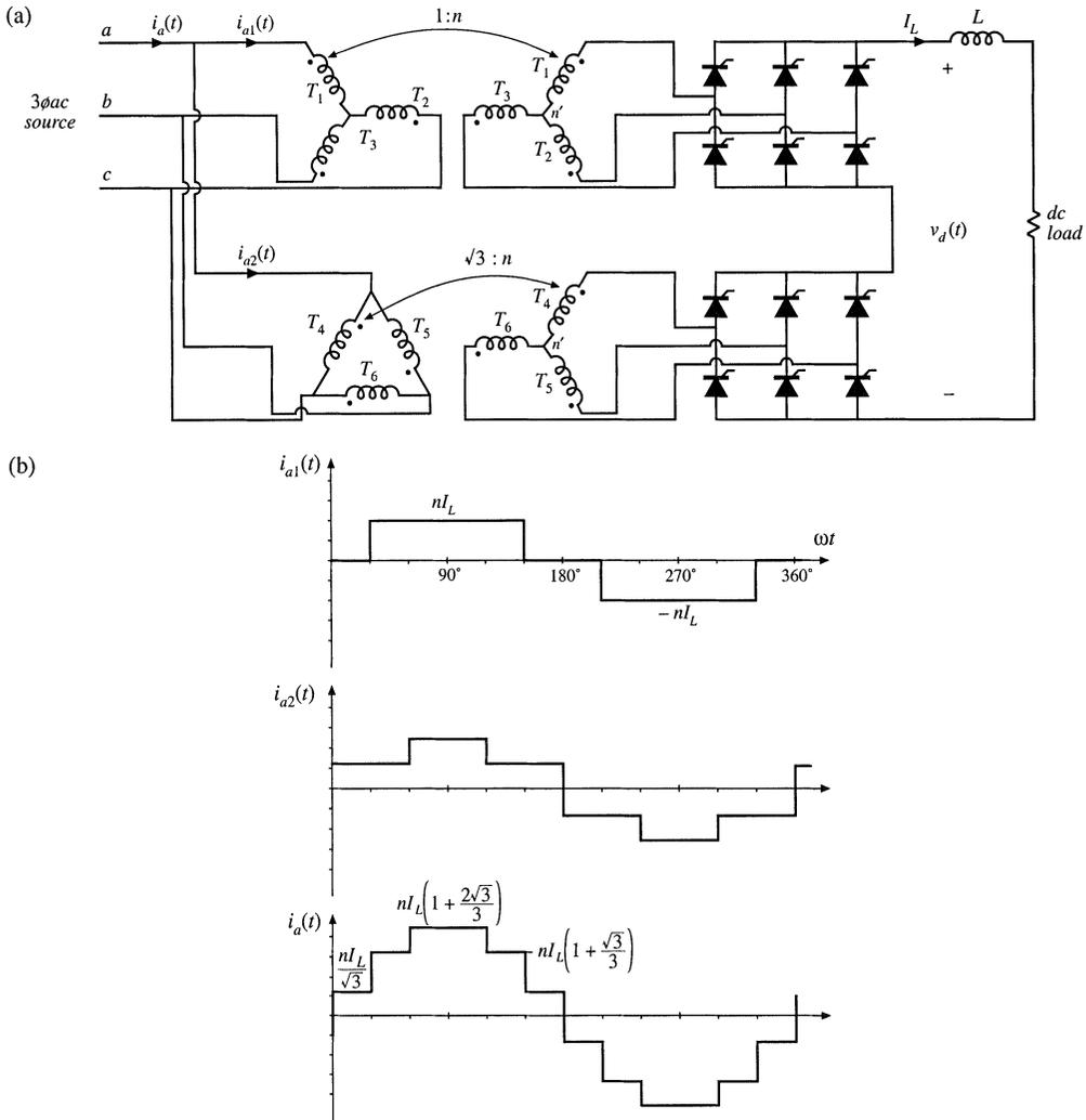
Fig. 17.27 Twelve-pulse rectifier: (a) circuit, (b) input phase *a* current waveforms.
