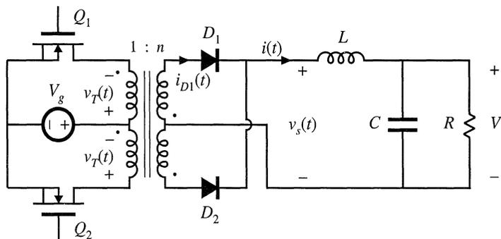
Fig. 6.28 Push-pull isolated buck converter.
