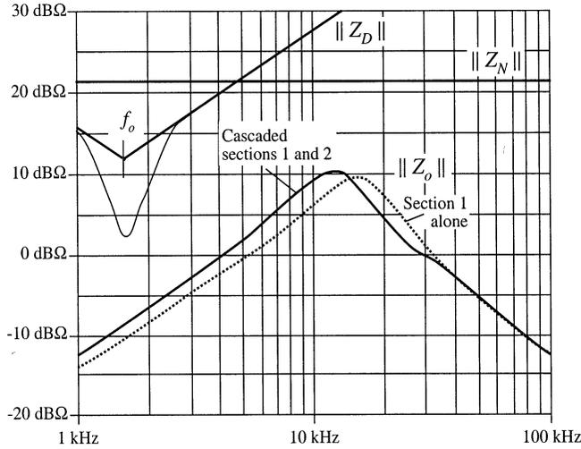
**Fig. 10.27** Comparison of the impedance design criteria  $\|Z_N(j\omega)\|$  and  $\|Z_D(j\omega)\|$ , Eq. (10.13), with the filter output impedance  $\|Z_o(j\omega)\|$ . *Solid line:*  $\|Z_o(j\omega)\|$  of cascaded design. *Dashed line:*  $\|Z_o(j\omega)\|$  of section 1 alone.
