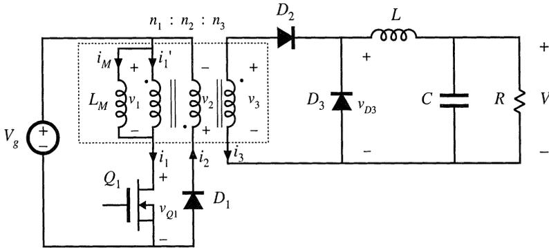
Fig. 6.23 Forward converter, with transformer equivalent circuit model.
