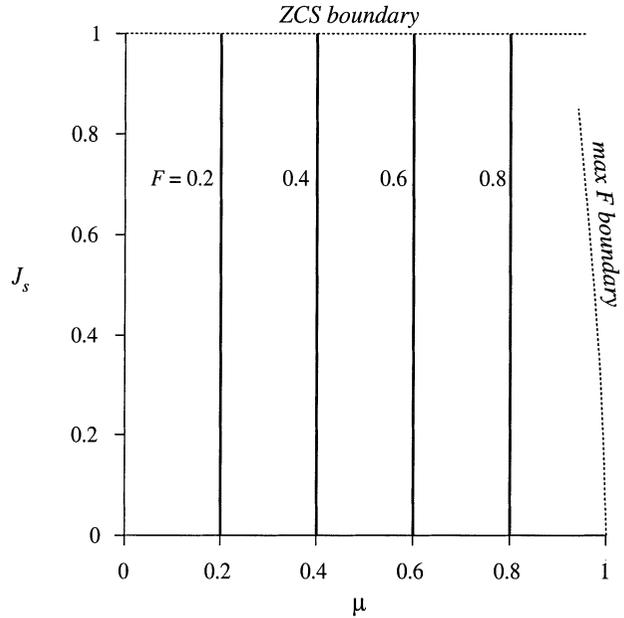
**Fig. 20.19** Characteristics of the full-wave ZCS quasi-resonant switch.
