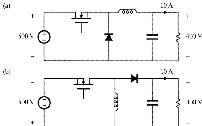
**Fig. 3.35** Problem 3.8: interfacing a 500 V source to a 400 V load, using (a) a buck converter, (b) a buck-boost converter.
