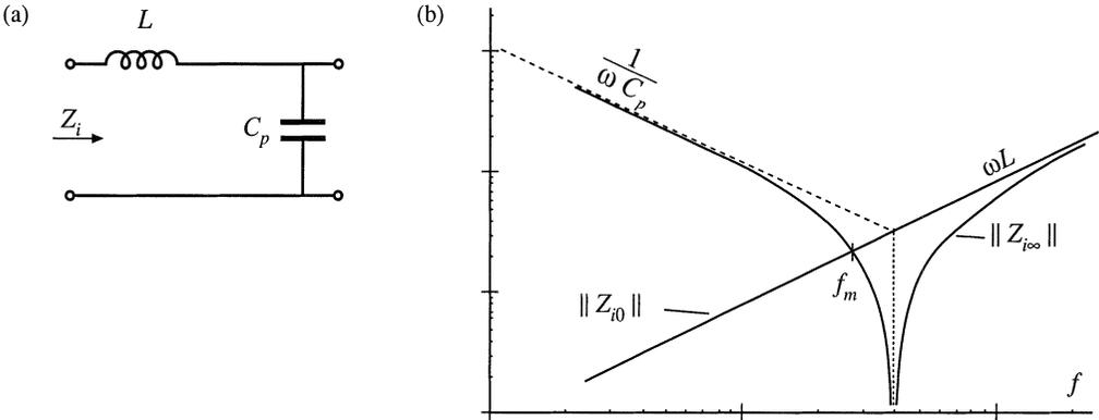
**Fig. 19.33** Tank network, parallel resonant converter example: (a) tank circuit, (b) Bode plot of input impedance magnitude  $\|Z_i\|$  for the limiting cases  $R \rightarrow 0$  and  $R \rightarrow \infty$ .
