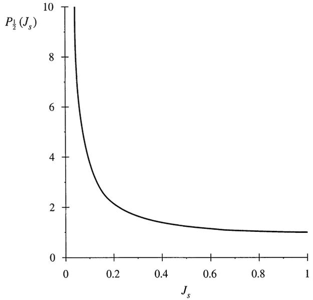
Fig. 20.16 Characteristics of the half-wave ZCS quasi-resonant switch.
