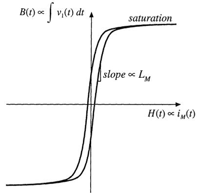
Fig. 6.17  $B$ – $H$  characteristics of transformer core.
