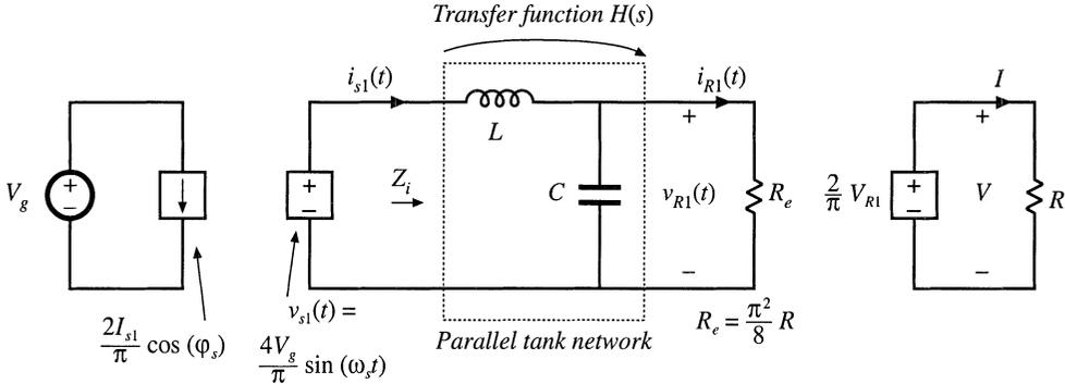
**Fig. 19.22** Equivalent circuit for the parallel resonant converter, which models the fundamental components of the tank waveforms, and the dc components of the converter input current and output voltage.
