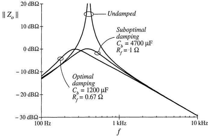
**Fig. 10.22** Comparison of the output impedances of the design with optimal parallel  $R_f$ - $C_b$  damping, the suboptimal design of Section 10.3.2, and the original undamped filter.
