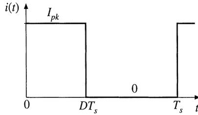
Pulsating waveform with linear ripple, Fig. A.6:
