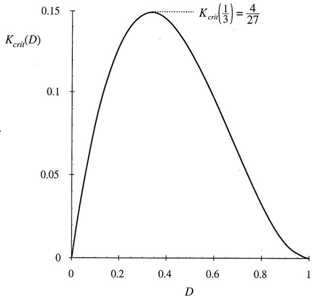
Fig. 5.13 Boost converter  $K_{crit}(D)$  vs.  $D$ .
