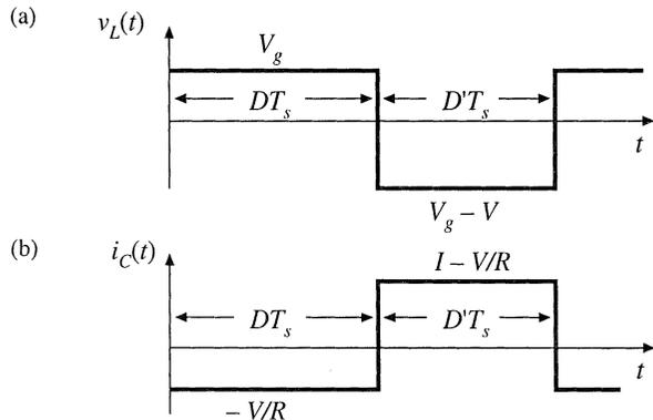
Fig. 2.15 Boost converter voltage and current waveforms.
