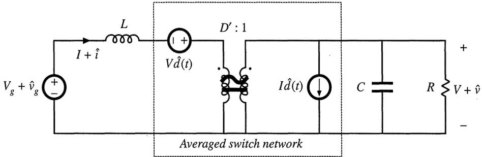
Fig. 7.47 Dc and small-signal ac averaged circuit model of the boost converter.
