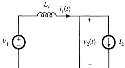
**Fig. 20.11** Circuit of the switch network during subinterval 1.
