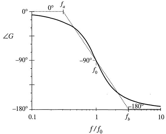
vicinity of the corner frequency  $f_0$ , as illustrated in Fig. 8.22. As in the case of the real single pole, we could choose the slope of this asymptote to be identical to the slope of the actual curve at  $f=f_0$ . It can be shown that this choice leads to the following asymptote break frequencies:
