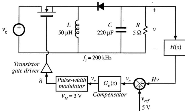
Fig. 9.46 Buck-boost voltage regulator system, Problem 9.9.
