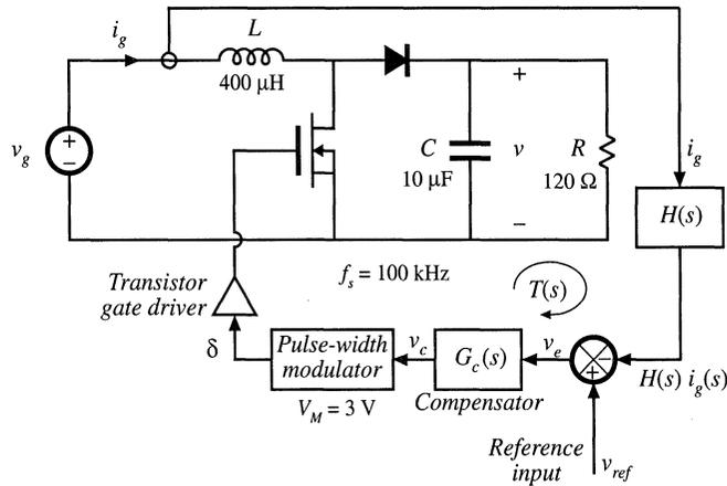
**Fig. 9.44** Boost converter system with current feedback, Problem 9.7.
