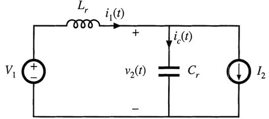
**Fig. 20.12** Circuit of the switch network during subinterval 2.
