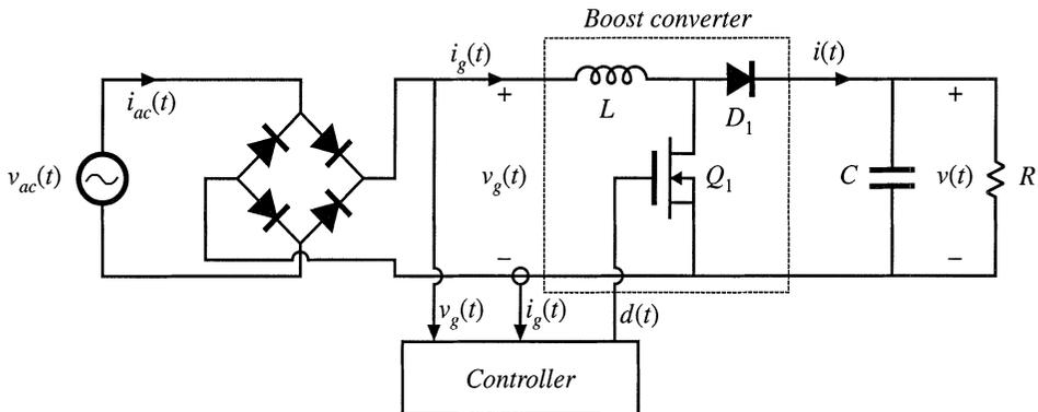
Fig. 18.5 Rectifier system based on the boost converter.
