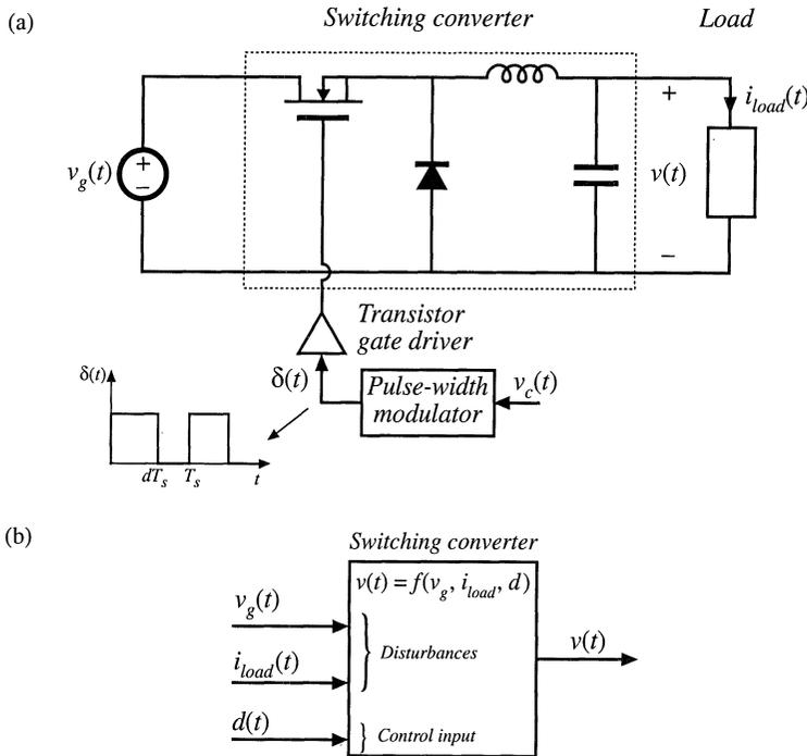
**Fig. 9.1** The output voltage of a typical switching converter is a function of the line input voltage  $v_g$ , the duty cycle  $d$ , and the load current  $i_{load}$ : (a) open-loop buck converter; (b) functional diagram illustrating dependence of  $v$  on the independent quantities  $v_g$ ,  $d$ , and  $i_{load}$ .
