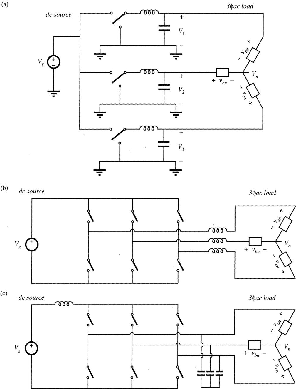
**Fig. 6.13** Dc-3 $\phi$ ac inverter topologies: (a) differential connection of 3 $\phi$  load across outputs of buck converters; (b) simplification of low-pass filters to obtain the dc-3 $\phi$ ac voltage-source inverter; (c) the dc-3 $\phi$ ac current-source inverter.
