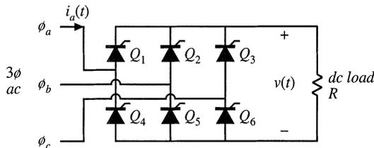
Fig. 17.30 Three-phase controlled rectifier circuit of Problem 17.3.
