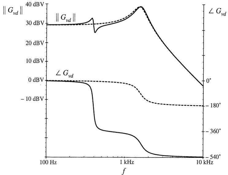
**Fig. 10.4** Control-to-output transfer functions predicted by the equivalent circuit models of Fig. 10.3. *Dashed lines:* without input filter [Fig. 10.3(a)]. *Solid lines:* with input filter [Fig. 10.3(b)].
