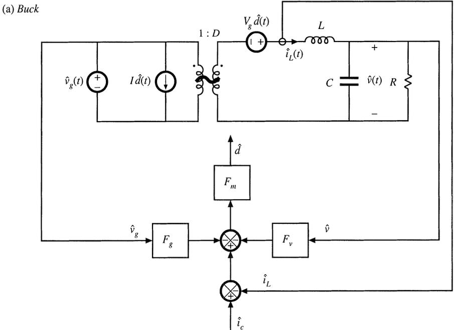
**Fig. 12.25** More accurate models of current-programmed converters: (a) buck, (b) boost, (c) buck-boost.
