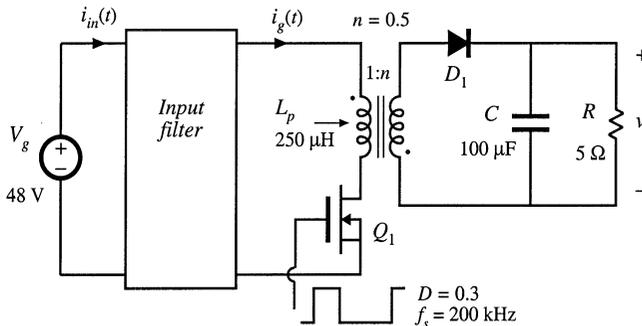
**Fig. 10.30** Flyback converter, Problems 10.1, 10.4, 10.6, 10.8, and 10.10.
