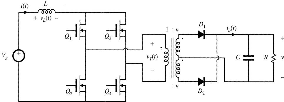
Fig. 6.34 Full-bridge transformer-isolated boost converter.
