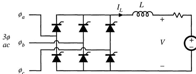
**Fig. 17.14** If the load is capable of supplying power, then the 3 $\phi$  bridge circuit functions as an inverter for  $V < 0$  and  $\alpha > 90^\circ$ .
