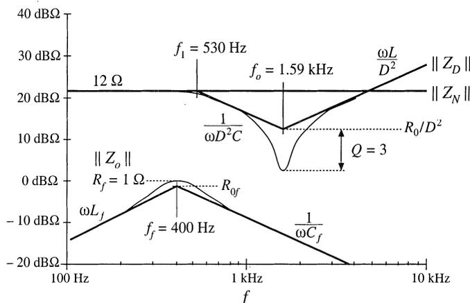
**Fig. 10.18** Impedance design criteria  $\|Z_N(j\omega)\|$  and  $\|Z_D(j\omega)\|$  from Fig. 10.10, with the filter output impedance  $\|Z_o(j\omega)\|$  of Fig. 10.17(b) superimposed. The design criteria of Eq. (10.13) are well satisfied.
