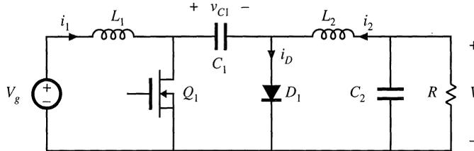
Fig. 5.23 Ćuk converter, Problems 5.5, 5.6, 5.11, and 5.12
