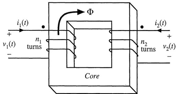
Fig. 13.14 Magnetic circuit that models the two-winding transformer of Fig. 13.13.
