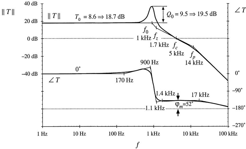
Fig. 9.28 The compensated loop gain of Eq. (9.59).
