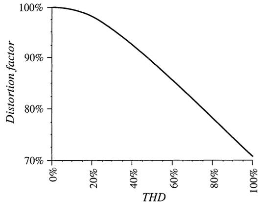
**Fig. 16.5** Distortion factor vs. total harmonic distortion.
