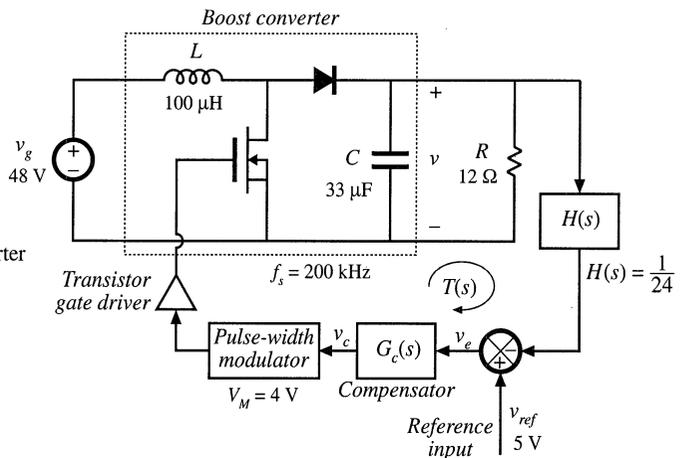
**Fig. 9.42** Boost converter system of Problem 9.3.
