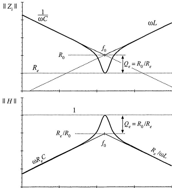
**Fig. 19.16** Construction of the Bode diagrams of  $Z_i(s)$  and  $H(s)$  for the series resonant converter.
