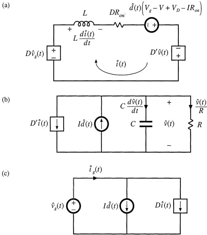
**Fig. 7.34** Circuits equivalent to the small-signal converter equations: (a) inductor loop, (b) capacitor node, (c) input port.
