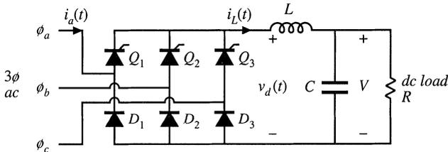
Fig. 17.29 Three-phase half-controlled rectifier circuit of Problem 17.2.
