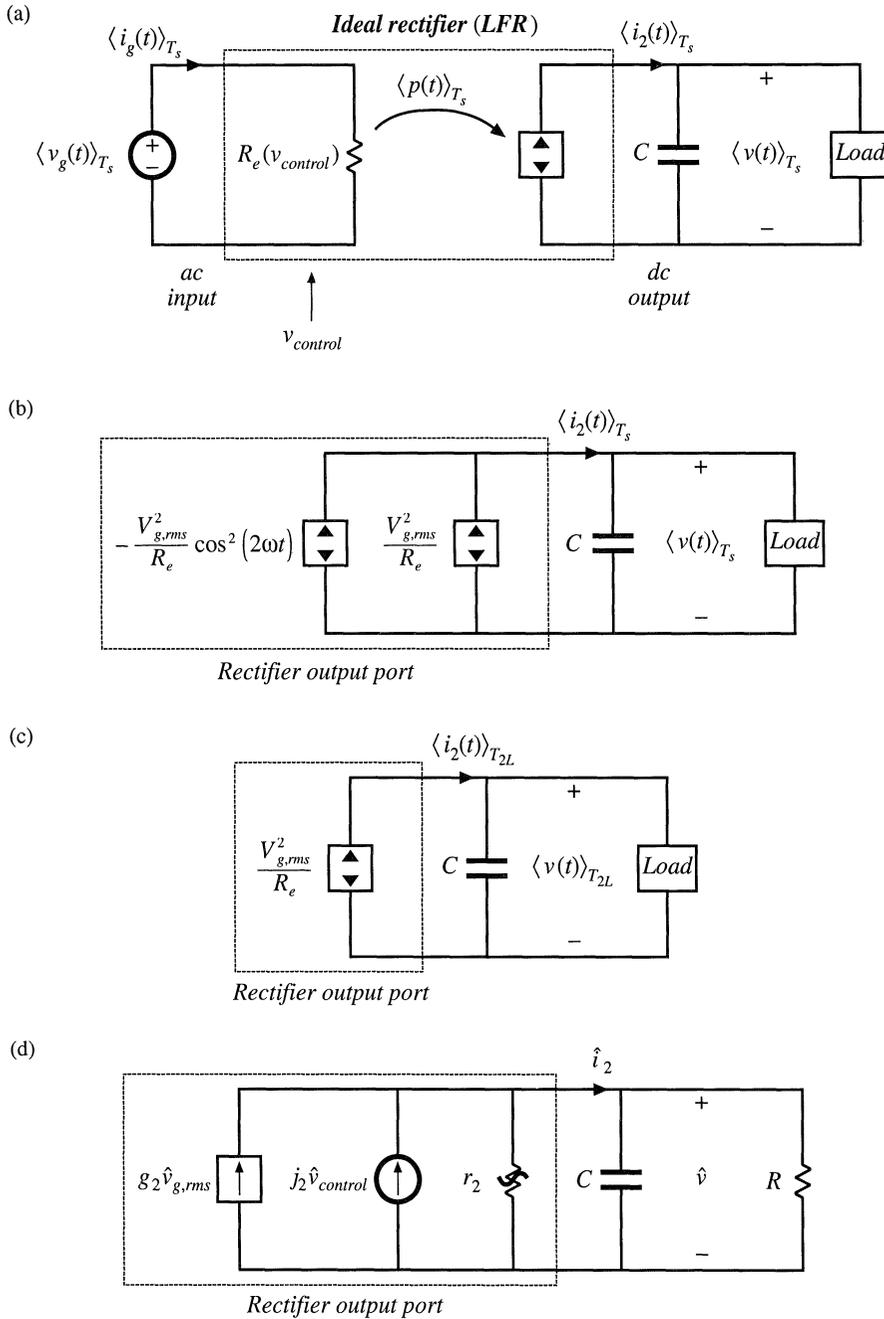
**Fig. 18.29** Steps in the derivation of low-frequency small-signal rectifier model: (a) large-signal LFR model, averaged over one switching period  $T_s$ ; (b) separation of power source into its constant and time-varying components; (c) removal of second-harmonic components by averaging over one-half of the ac line period,  $T_{2L}$ ; (d) small-signal model obtained by perturbation and linearization of Fig. 18.29(c).
