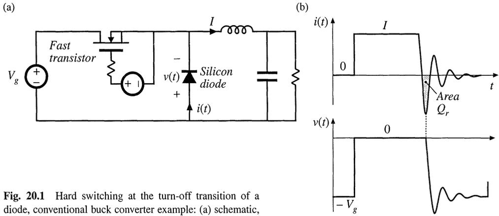
Fig. 20.1 Hard switching at the turn-off transition of a diode, conventional buck converter example: (a) schematic, (b) diode voltage and current waveforms.
