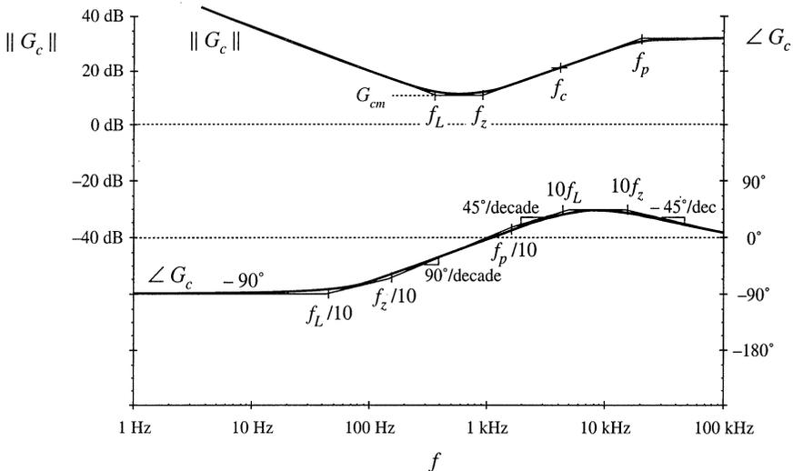
Fig. 9.30 PID compensator transfer function, Eq. (9.60).
