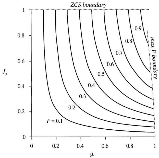
of the current  $I_2$ , via  $J_s$ . The characteristics end at  $J_s = 1$ ; according to Eq. (20.31), the zero current switching property is lost when  $J_s > 1$ . The characteristics also end at the maximum switching frequency limit given by Eq. (20.31). This expression can be simplified by use of Eq. (20.43), to express the limit in terms of  $\mu$  as follows:
