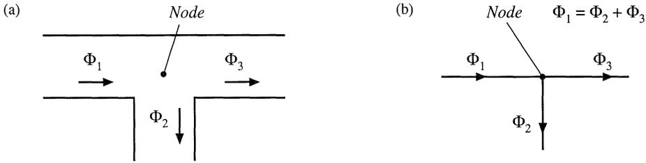
**Fig. 13.10** Kirchoff's current law, applied to magnetic circuits: the net flux entering a node must be zero: (a) physical element, in which three legs of a core meet at a node; (b) magnetic circuit model.
