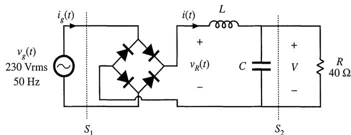
**Fig. 16.13** Passive rectifier circuit of Problem 16.1
