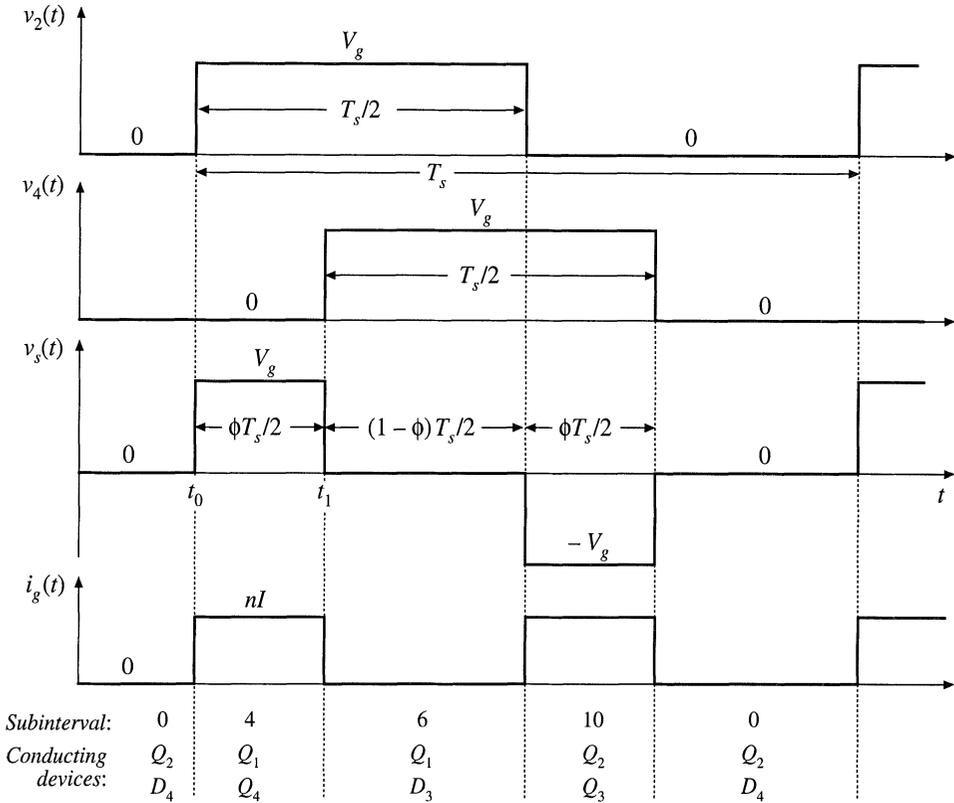
**Fig. 20.37** Phase-shift control of the ZVT full-bridge converter. Switching transitions are neglected in this figure, and subinterval numbering follows Fig. 20.38.
