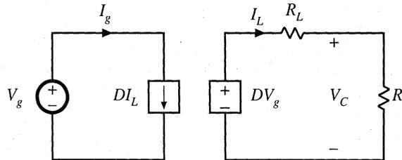
Fig. 3.21 Equivalent circuit of the buck converter, including a 1:D dc transformer and the inductor winding resistance  $R_L$ .
