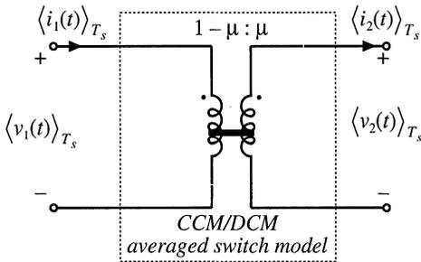
**Fig. B.11** A general averaged switch model using the equivalent switch conversion ratio  $\mu$ .
