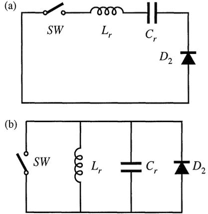
**Fig. 20.28** Elimination of converter low-frequency elements reduces the quasi-square-wave switch cells to these networks: (a) ZCS quasi-square-wave network, (b) ZVS quasi-square-wave network.
