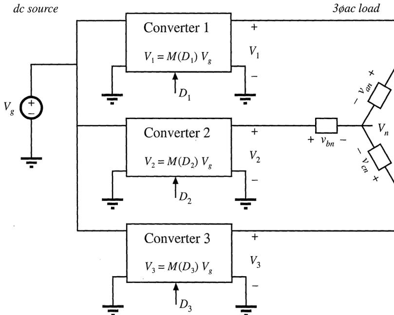
Fig. 6.12 Generation of dc-3φac inverter by differential connection of 3φ load.
