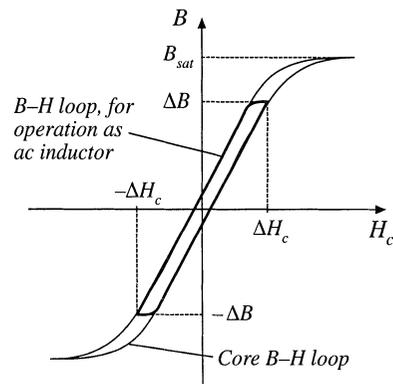
Fig. 13.44 Operational B-H loop of an ac inductor.
