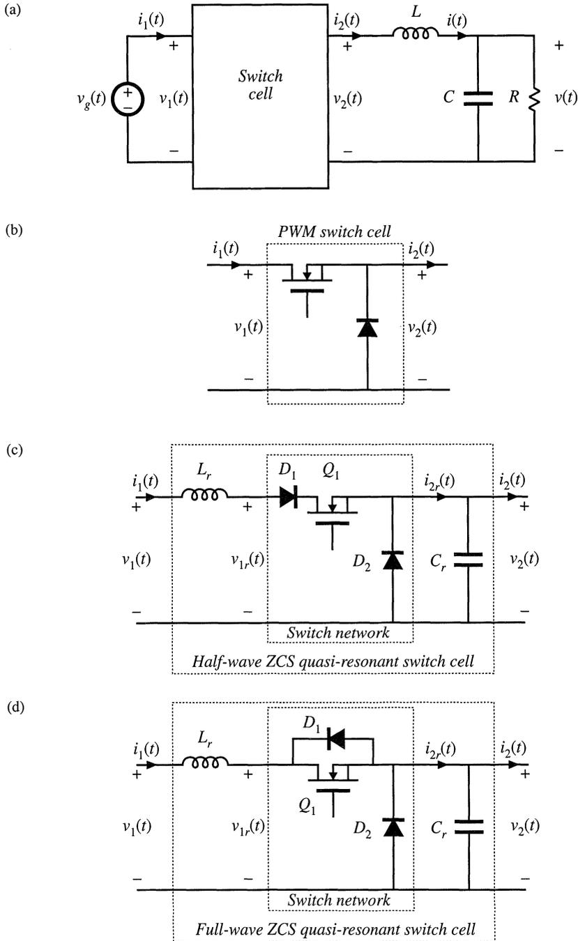
**Fig. 20.8** Implementation of the switch cell in a buck converter: (a) buck converter, with arbitrary switch cell; (b) PWM switch cell; (c) half-wave ZCS quasi-resonant switch cell; (d) full-wave ZCS quasi-resonant switch cell.
