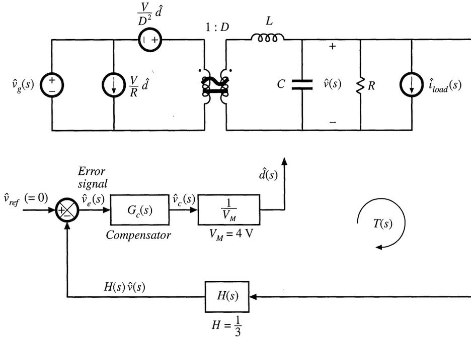
Fig. 9.23 System small-signal ac model, design example.
