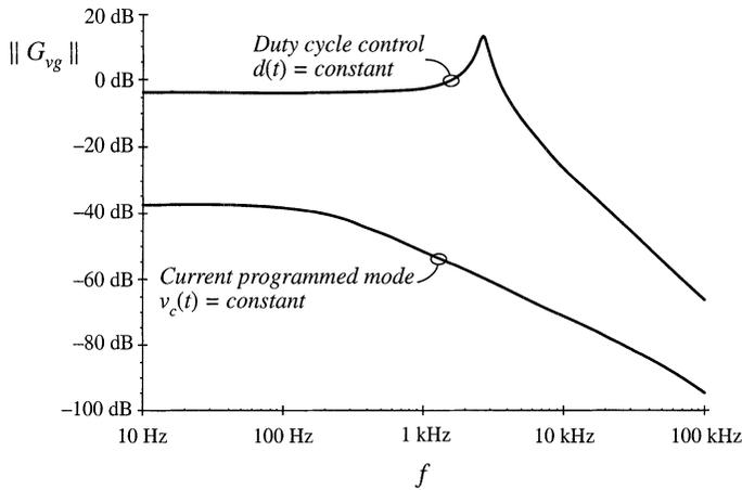
**Fig. 12.28** Comparison of CPM control with duty-cycle control, for the line-to-output frequency response of the buck converter example.
