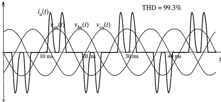
Fig. 17.10 Discontinuous conduction mode ac line-neutral voltages and phase *a* current.
