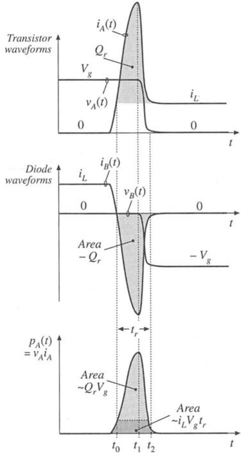
Fig. 4.51 Transistor-turn-on transition waveforms for the circuit of Fig. 4.50.
