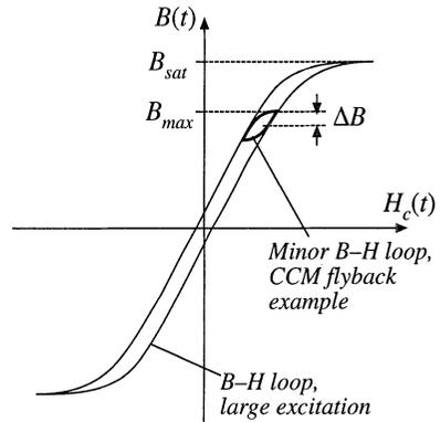
**Fig. 14.15** Variation of flux density  $B(t)$ , flyback transformer example.
