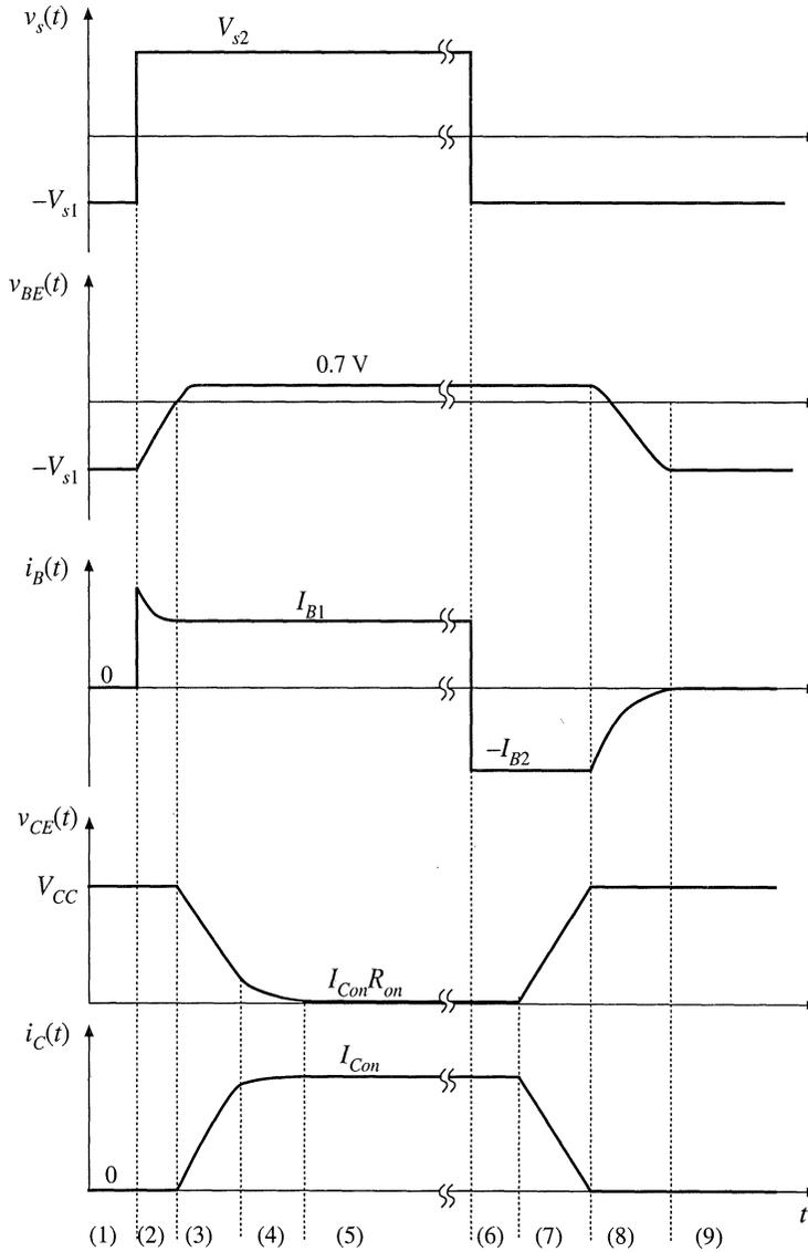
Fig. 4.32 BJT turn-on and turn-off transition waveforms.
