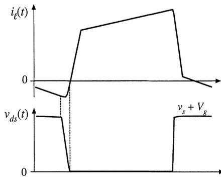
Fig. 20.40 Waveforms of the active-clamp snubber circuit of Fig. 20.39(a).
