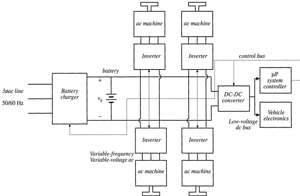
**Fig. 1.16** An electric vehicle power and drive system.
