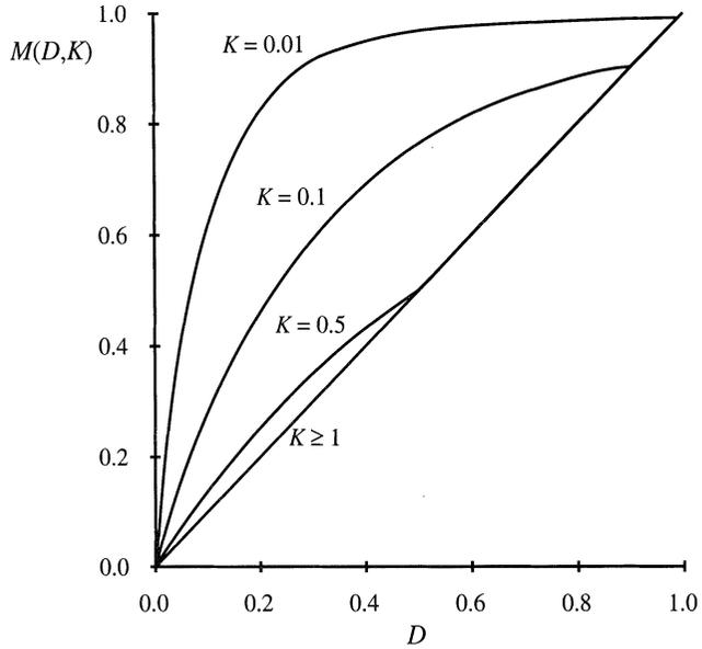
**Fig. 5.11** Voltage conversion ratio  $M(D, K)$ , buck converter.
