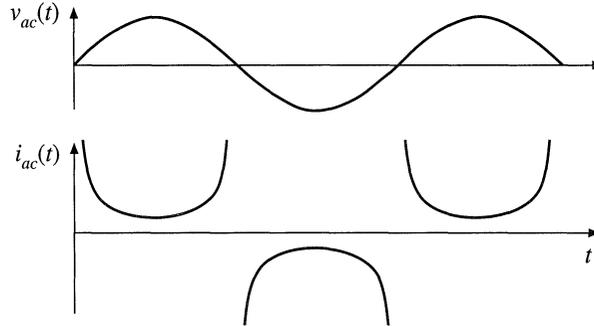
**Fig. 18.28** Ac line current waveform of the single-phase ideal rectifier with output voltage feedback, when it supplies constant instantaneous power to a dc load. The THD tends to infinity, and the power factor tends to zero.
