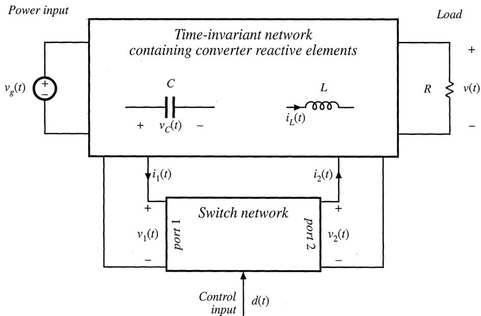
Fig. 7.36 A switching converter can be viewed as a switch network connected to a time-invariant network.
