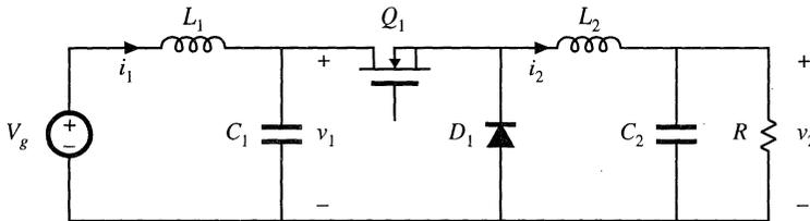
Fig. 5.25 Buck converter with input filter, Problems 5.9 and 5.10.
