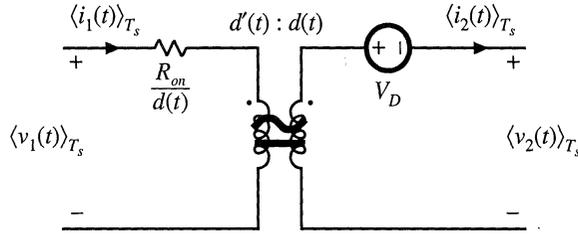
**Fig. 7.52** Large-signal averaged switch model for the general two-switch network of Fig. 7.50. This model includes conduction losses due to the transistor on-resistance  $R_{on}$  and the diode forward voltage drop  $V_D$ .
