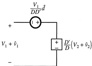
**Fig. 7.40** Linearization of the dependent voltage source.
