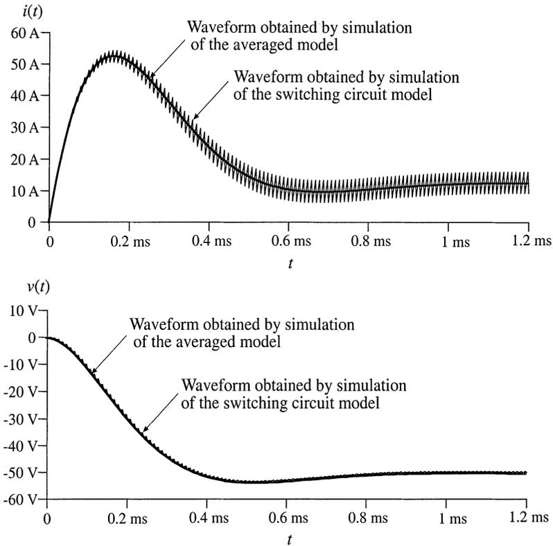
**Fig. B.9** Inductor current and output voltage waveforms obtained by transient simulation of the switching converter circuit shown in Fig. B.7, and by simulation of the averaged circuit model of Fig. B.8
