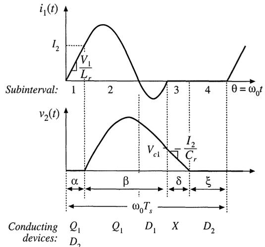
**Fig. 20.18** Tank inductor current and capacitor voltage waveforms, for the full-wave ZCS quasi-resonant switch cell of Fig. 20.8(d).
