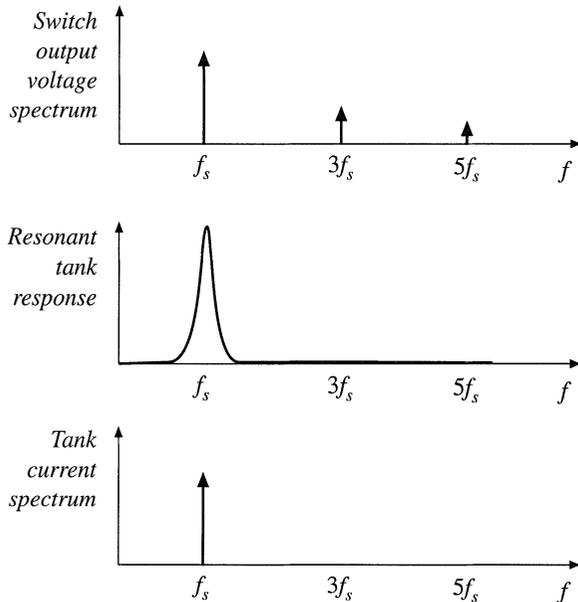
**Fig. 19.2** The tank network responds primarily to the fundamental component of the applied waveforms.
