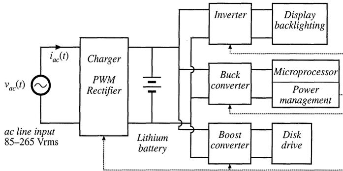
Fig. 1.14 A laptop computer power supply system.
