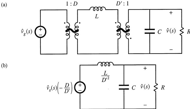
Fig. 8.30 Manipulation of buck-boost equivalent circuit to find the line-to-output transfer function  $G_{vg}(s)$ : (a) set  $\hat{d}$  sources to zero; (b) push inductor and  $\hat{v}_g$  source through transformers.
