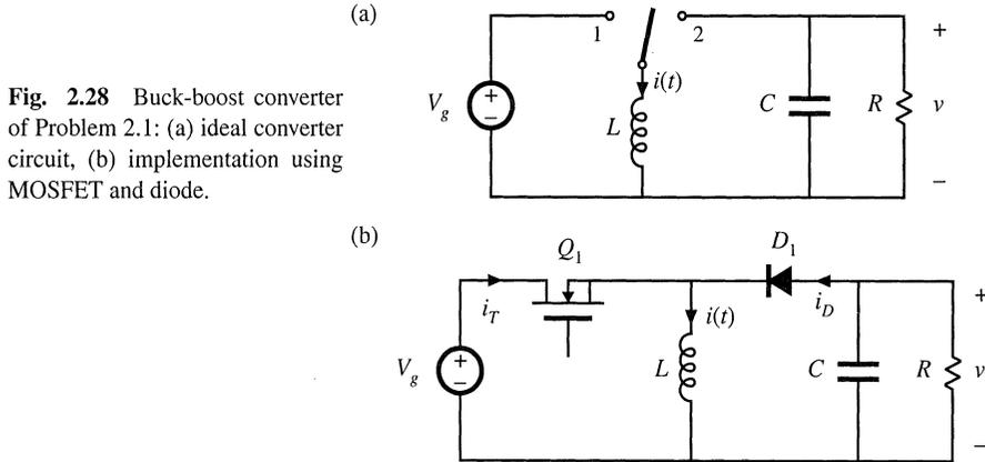
Fig. 2.28 Buck-boost converter of Problem 2.1: (a) ideal converter circuit, (b) implementation using MOSFET and diode.
