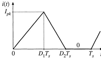
Triangular waveform, Fig. A.8:
