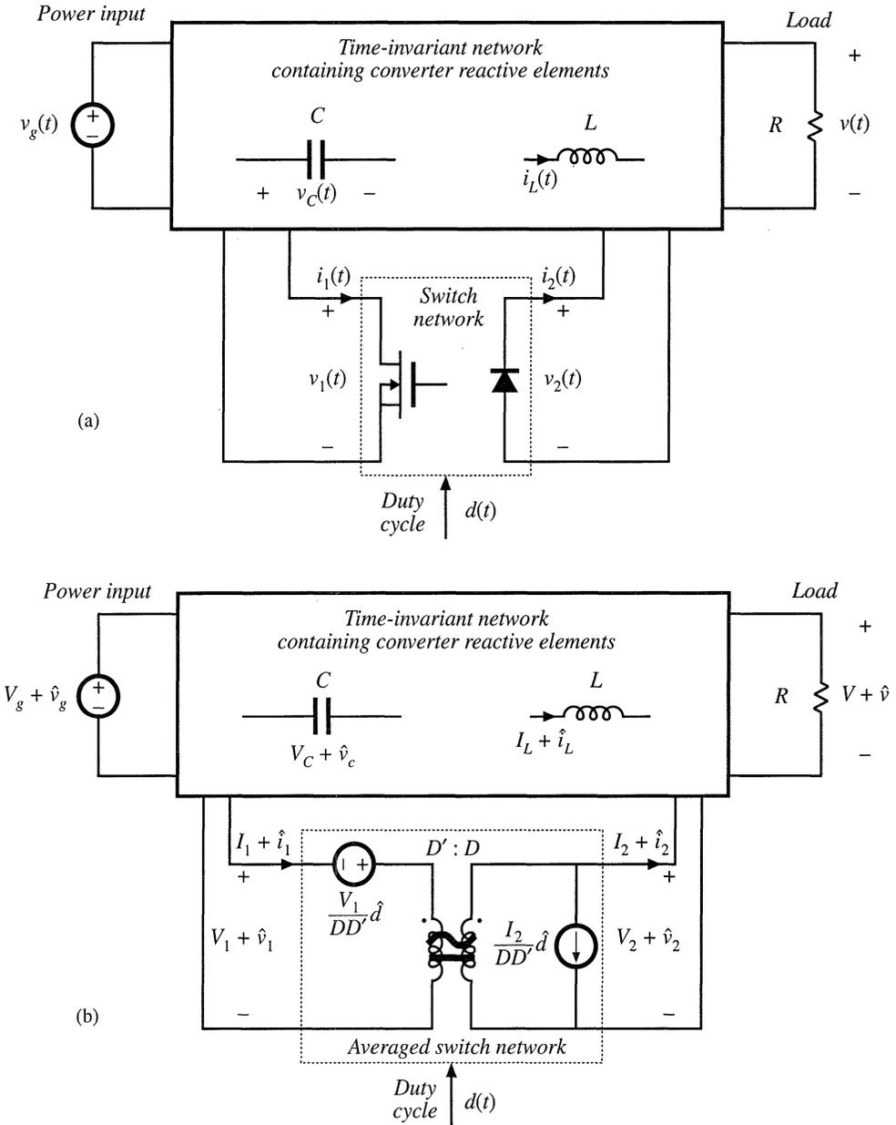
**Fig. 7.43** Construction of an averaged circuit model for a two-switch converter operating in CCM: (a) the converter circuit with the general two-switch network identified; (b) dc and ac small-signal averaged circuit model obtained by replacing the switch network with the averaged model.
