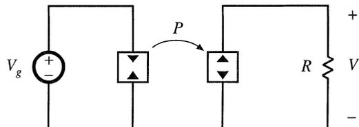
**Fig. 12.34** Averaged models of current-programmed DCM converters: (a) buck, (b) boost.
