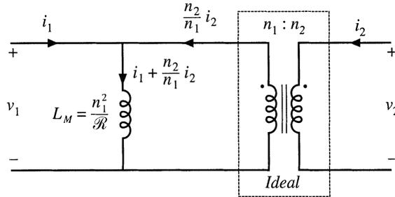
**Fig. 13.16** Transformer model including magnetizing inductance.
