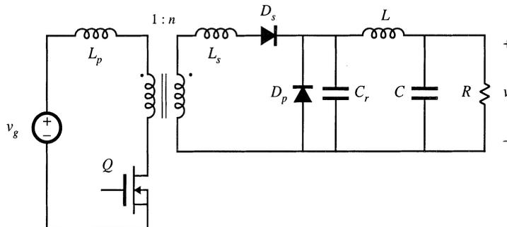
**Fig. 20.43** Forward converter with resonant switch, Problem 20.1.
