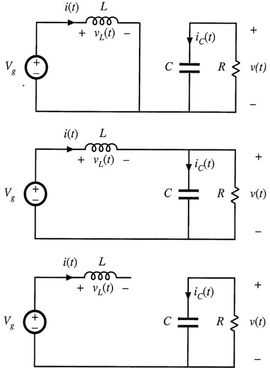
**Fig. 5.15** Boost converter circuits: (a) during subinterval 1,  $0 < t < D_1 T_s$ , (b) during subinterval 2,  $D_1 T_s < t < (D_1 + D_2) T_s$ , (c) during subinterval 3,  $(D_1 + D_2) T_s < t < T_s$ .
