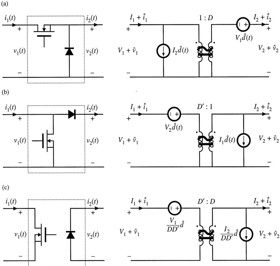
**Fig. 7.50** Three basic switch networks, and their CCM dc and small-signal ac averaged switch models: (a) the buck switch network, (b) the boost switch network, and (c) the general two-switch network.
