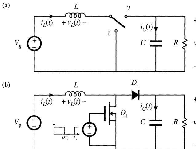
Fig. 2.13 Boost converter: (a) with ideal switch, (b) practical realization using MOSFET and diode.
