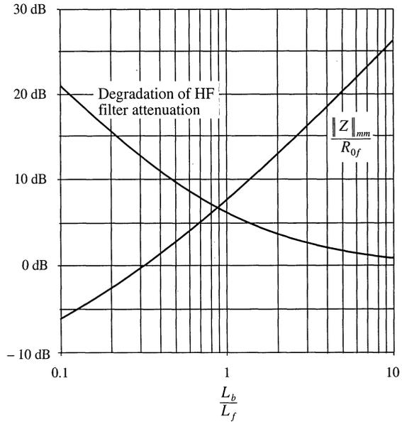
**Fig. 10.23** Performance attained via optimal design procedure, parallel  $R_f$ - $L_b$  circuit of 10.20(b). Optimum peak filter output impedance  $\|Z_o\|_{mm}$  and increase of filter high-frequency gain, vs.  $n = L_b/L_f$ .
