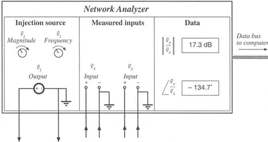
**Fig. 8.58** Key features and functions of a network analyzer: sinusoidal source of controllable amplitude and frequency, two inputs, and determination of relative magnitude and phase of the input components at the injection frequency.
