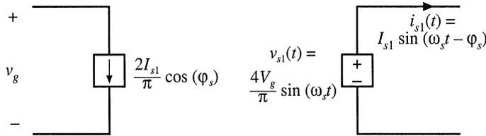
Fig. 19.9 An equivalent circuit for the switch network, which models the fundamental component of the output voltage waveform and the dc component of the input current waveform.
