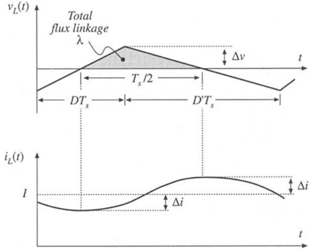
portion of the capacitor current waveform. By the capacitor relation  $Q = CV$ ,
