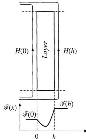
Fig. 13.30 The power loss is determined for a uniform layer. Uniform tangential magnetic fields  $H(0)$  and  $H(h)$  are applied to the layer surfaces.
