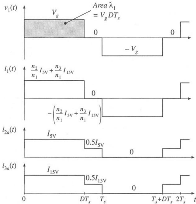
Fig. 15.9 Transformer waveforms, full-bridge converter example.
