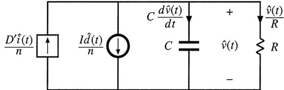
**Fig. 7.25** Circuit equivalent to the small-signal ac input source current equation, Eq. (7.76) or (7.74).
