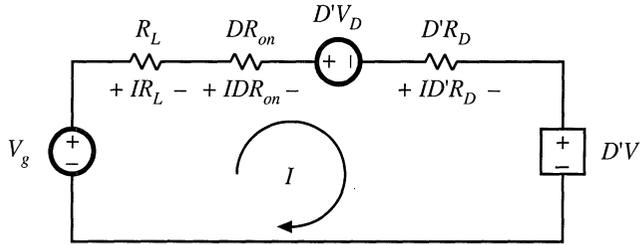
**Fig. 3.26** Equivalent circuit corresponding to Eq. (3.32).
