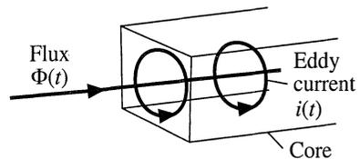
Fig. 13.19 Eddy currents in an iron core.
