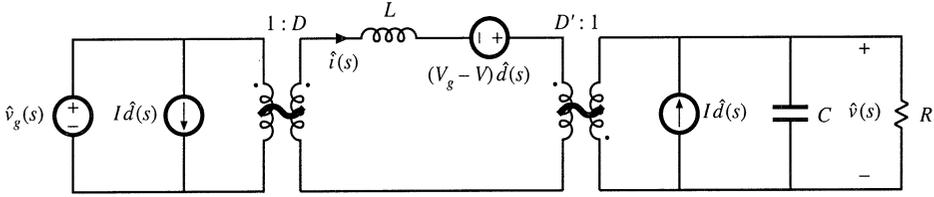
Fig. 8.29 Buck-boost converter equivalent circuit derived in Section 7.2.
