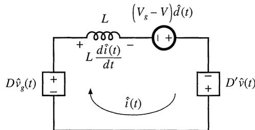
Fig. 7.13 Circuit equivalent to the small-signal ac inductor loop equation of Eq. (7.43) or (7.36).
