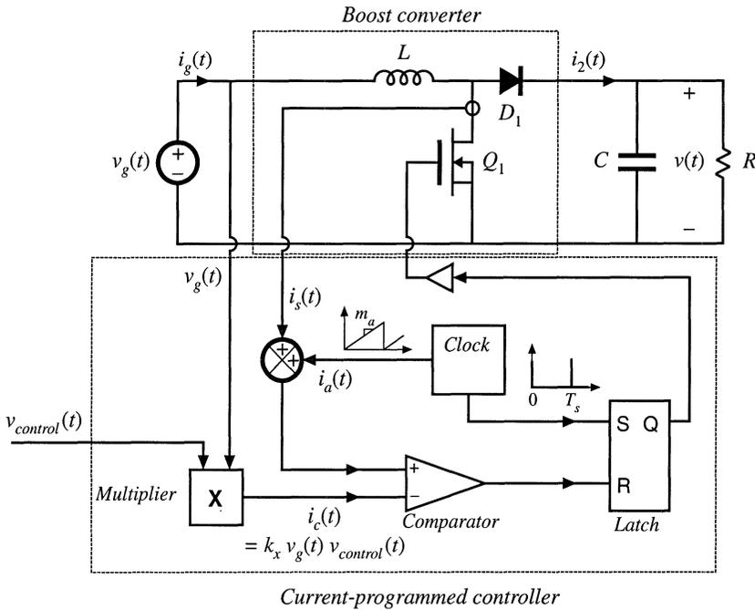
Fig. 18.16 Current-programmed control of a boost rectifier.
