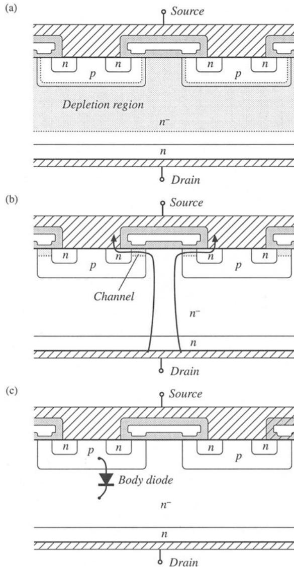
**Fig. 4.27** Operation of the power MOSFET: (a) in the off state,  $v_{ds}$  appears across the depletion region in the  $n^-$  region; (b) current flow through the conducting channel in the on state; (c) body diode due to the  $p$ - $n^-$  junction.
