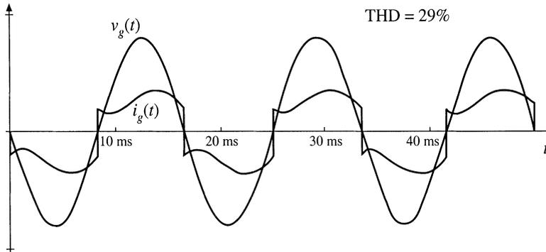
**Fig. 17.2** Typical ac line current and voltage waveforms, continuous conduction mode.  $f_0/f_L = 5$ ,  $Q = 0.25$ .
