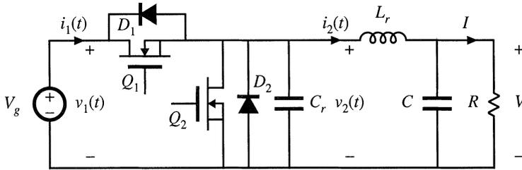
Fig. 20.33 Quasi-square wave ZVS buck converter containing a synchronous rectifier.
