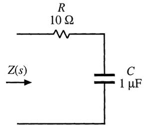
Fig. 8.38 Series  $R$ - $C$  network example.
