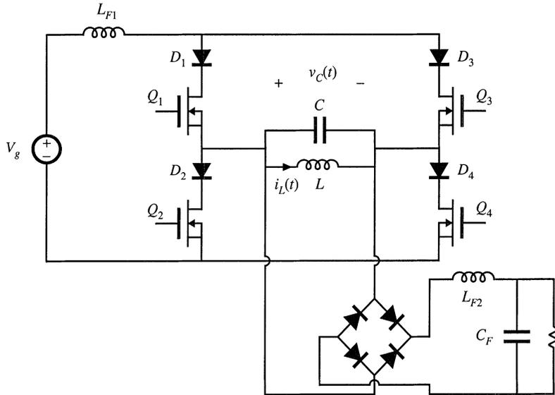
**Fig. 19.54** Dual of the series resonant converter, Problem 19.3.
