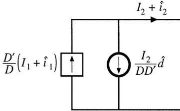
Fig. 7.41 Linearization of the dependent current source.
