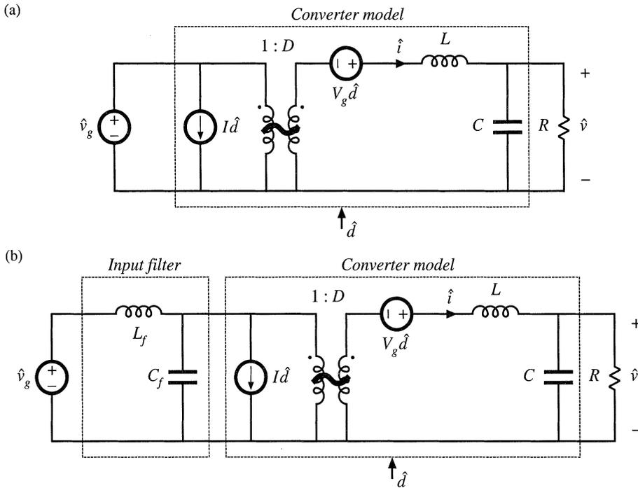
**Fig. 10.3** Small-signal equivalent circuit models of the buck converter: (a) basic converter model, (b) with addition of input filter.
