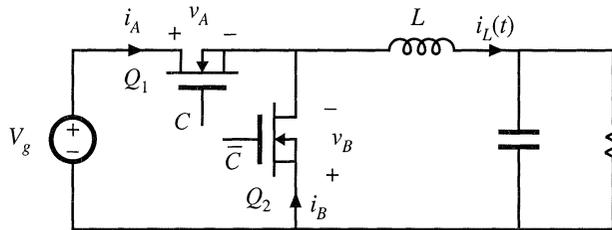
Fig. 4.23 Buck converter, implemented using a synchronous rectifier.
