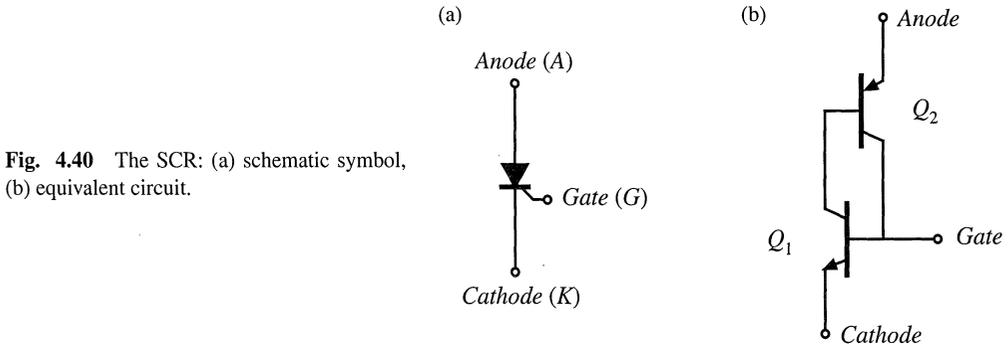
**Fig. 4.40** The SCR: (a) schematic symbol, (b) equivalent circuit.
