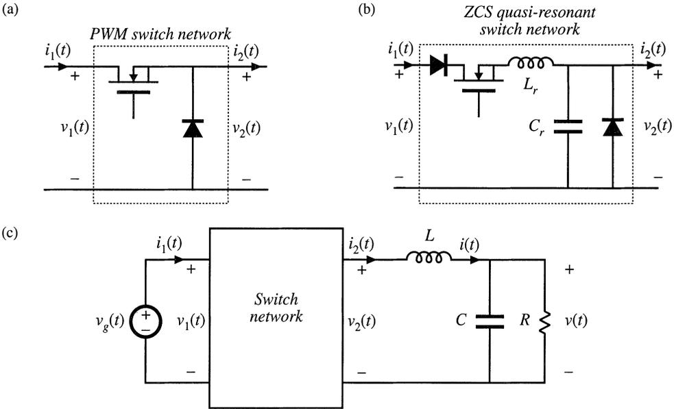
**Fig. 19.5** Derivation of a quasi-resonant converter: (a) conventional PWM switch network, (b) a ZCS quasi-resonant switch network, (c) a quasi-resonant buck converter is obtained by employing a quasi-resonant switch network such as (b) in a buck converter.
