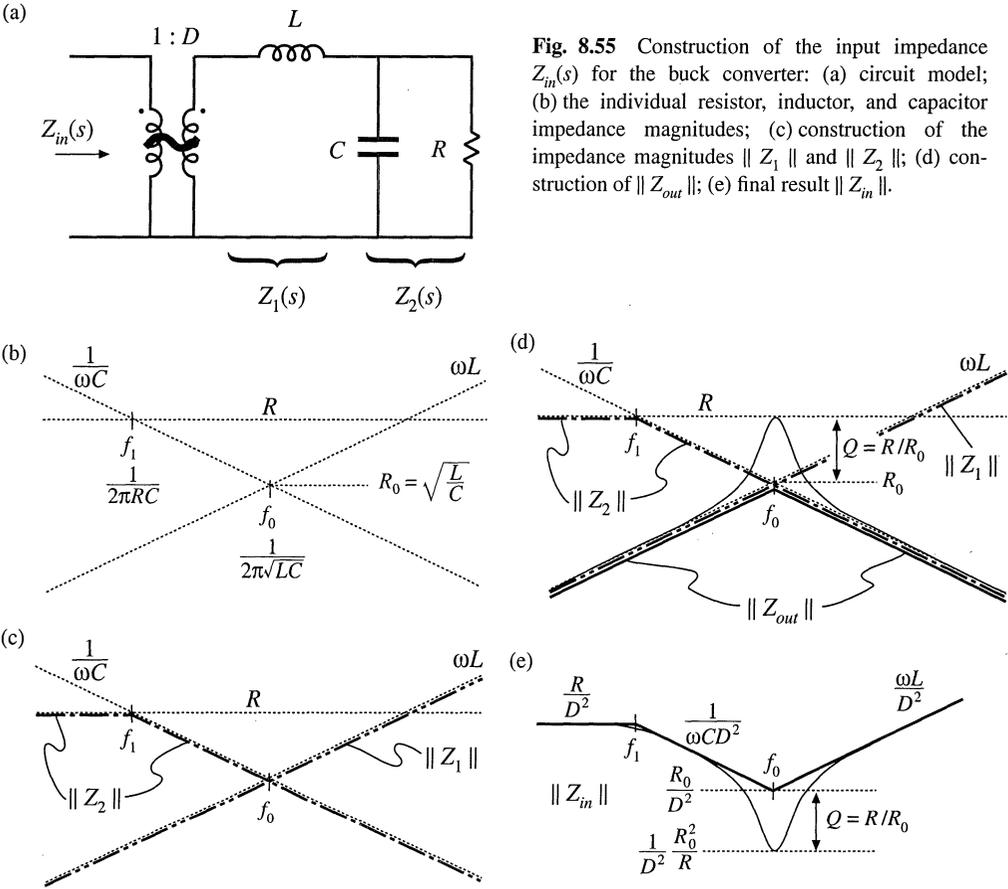
**Fig. 8.55** Construction of the input impedance  $Z_{in}(s)$  for the buck converter: (a) circuit model; (b) the individual resistor, inductor, and capacitor impedance magnitudes; (c) construction of the impedance magnitudes  $\|Z_1\|$  and  $\|Z_2\|$ ; (d) construction of  $\|Z_{out}\|$ ; (e) final result  $\|Z_{in}\|$ .
