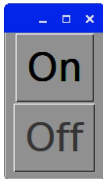
Figure 11-13. An on/off switch in guizero
