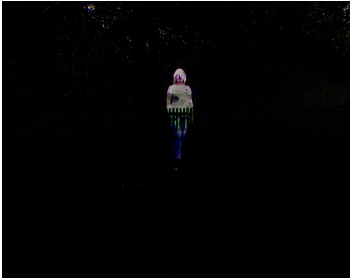
Figure 8-6. Movement detection, the difference image
