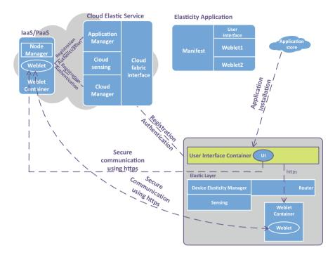
Fig. 1.13 Security framework for elastic computation
