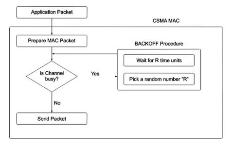
Fig. 27.2 Simple CSMA procedure
