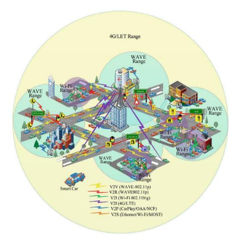
Fig. 22.3 Technologies for IoV communication
