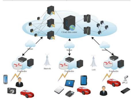
Fig. 20.3 Hierarchical architecture of fog computing
