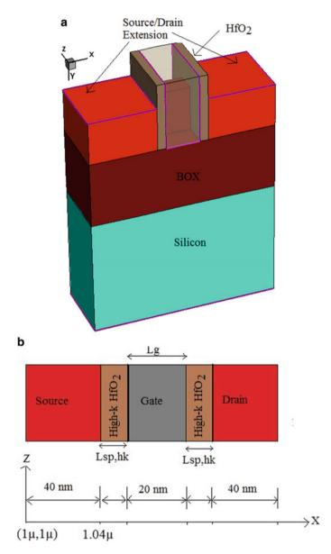
Fig. 12.1 (a) Device-D1 (high-k SOI FinFET) and (b) cross-section of device-D1
