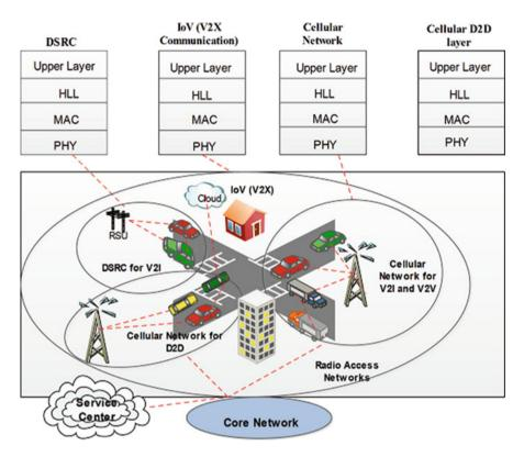
Fig. 22.5 Heterogeneous vehicular framework
