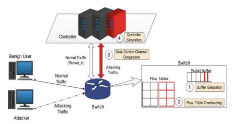
Fig. 15.9 DDoS attack in SDN
