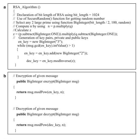
Fig. 24.11 (a) Pseudo code of RSA algorithm. (b) Pseudo code of RSA encryption and decryption
