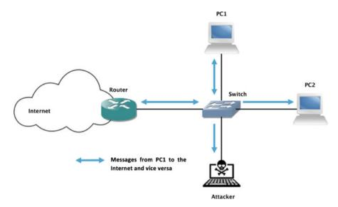
Fig. 6.12 Switch behaving like a hub when its CAM table has been overflown
