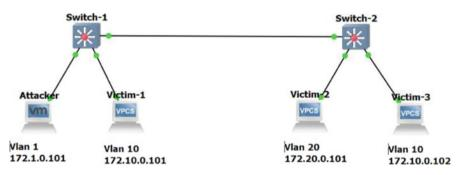
Fig. 6.17 A scenario with pre-configured VLANs and default settings
