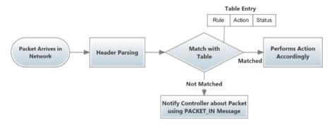
Fig. 15.4 Packet parsing in OpenFlow switch
