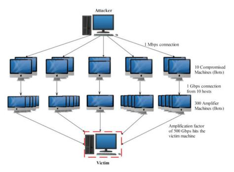
Fig. 15.6 Amplified DDoS attack
