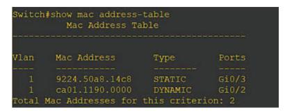
Fig. 6.14 Switch's CAM table with the port-security restrict policy
