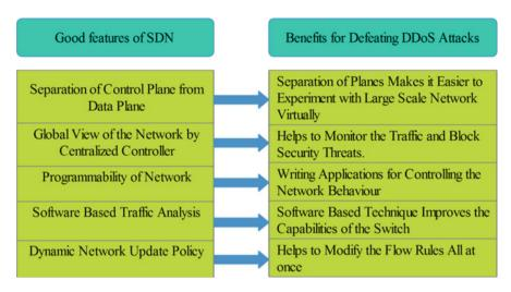
Fig. 15.8 Good features in SDN for defeating DDoS attack
