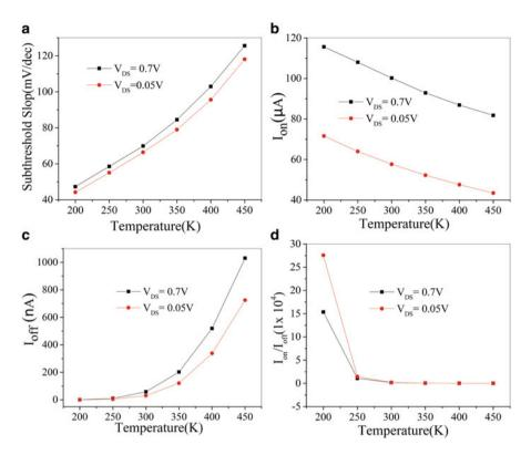
Fig. 12.2 (a) SS, (b)  $I_{on}$  current, (c)  $I_{off}$  current, and (d)  $I_{on}/I_{off}$  ratio versus temperature characteristics for high-k SOI FinFET at  $V_{DS} = 0.05$  V and  $V_{DS} = 0.7$  V
