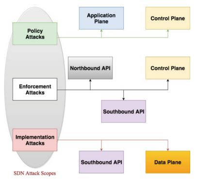
Fig. 14.5 The relation between SDN's five main components and the attack scopes
