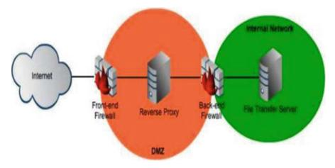
Fig. 13.6 Firewall architecture
