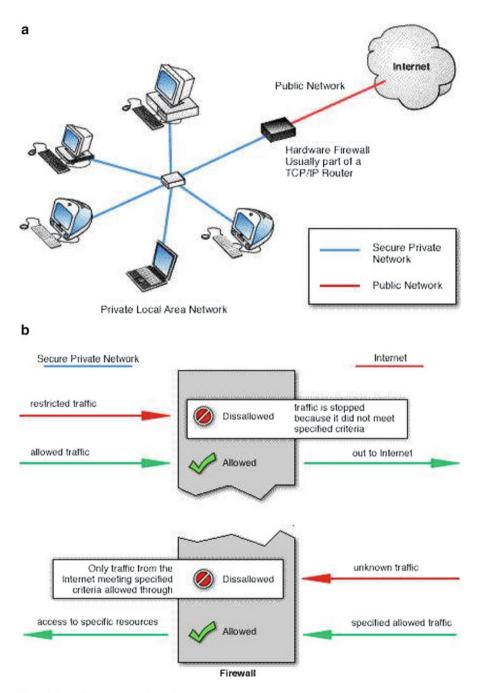
Fig. 13.7 (a, b) Hardware firewall
