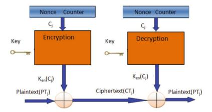
Fig. 7.7 CTR encryption and decryption processes
