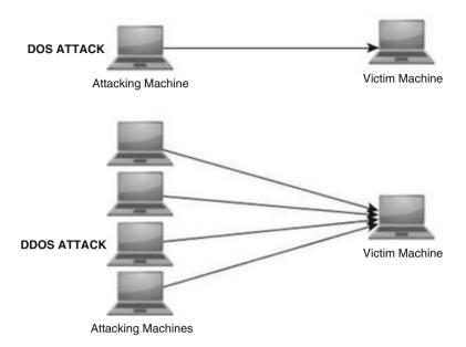
Fig. 16.1 DoS vs DDoS attack
