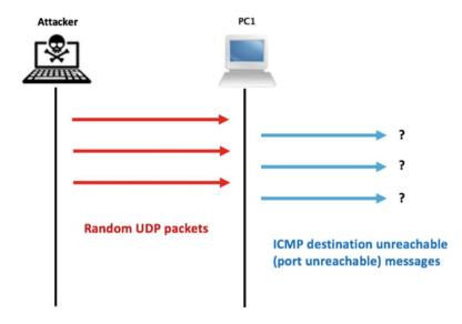
Fig. 6.27 UDP flooding attack
