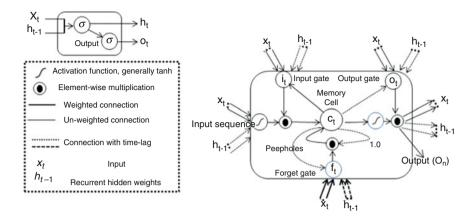
Fig. 37.2 Architecture of recurrent neural network (RNN) unit (left) and Long short-term memory (LSTM) memory block (right)
