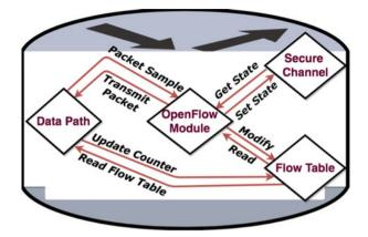
Fig. 14.10 Simplified data flow diagram for an OpenFlow-enabled forwarding device
