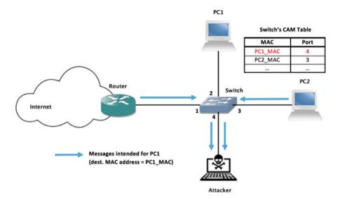
Fig. 6.9 Effects of the port stealing attack
