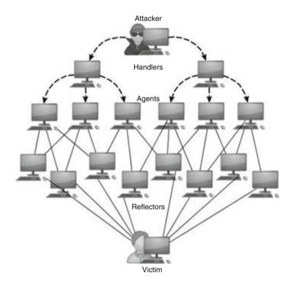
Fig. 16.6 Reflector model of DDoS attack network
