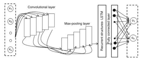
Fig. 37.4 An overview of combination of convolutional neural network (CNN) and long short-term memory (LSTM) architectures
