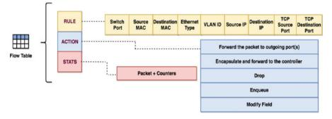
Fig. 14.2 Flow table of an OpenFlow-enabled forwarding device
