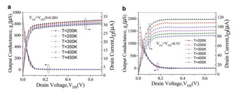
Fig. 12.4 I<sub>D</sub> and  $g_d$  versus  $V_{DS}$  characteristics of high-k SOI FinFET with temperature variation at (a)  $V_{GS} = 0.35$  V and (b)  $V_{GS} = 0.7$  V
