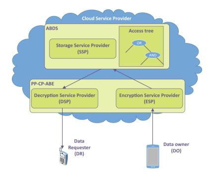
Fig. 1.9 System architecture for the secure data storage framework
