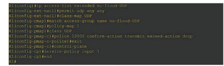
Fig. 6.31 The configuration of a policy to limit the input packet rate
