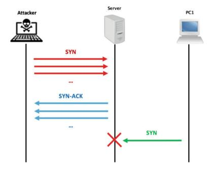
Fig. 6.33 TCP SYN flooding attack
