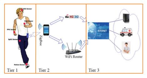
Fig. 7.2 Three tier architecture of WBAN
