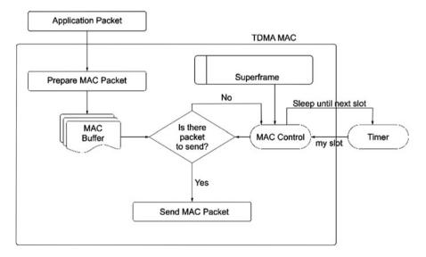
Fig. 27.1 Simple TDMA procedure
