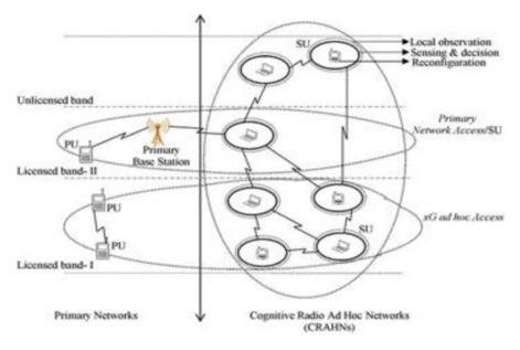
Fig. 10.1 Architecture block diagram of CRAHNs
