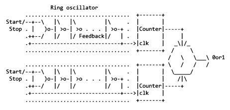
Fig. 18.3 Ring oscillator Physical Unclonable Function (PUF)
