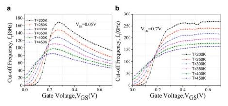
Fig. 12.6 Cutoff frequency ( $f_T)$  versus  $V_{GS}$  characteristics with temperature variation at (a)  $V_{DS}=0.05~V$  and (b)  $V_{DS}=0.7~V$
