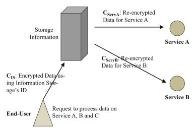
Fig. 4.5 Proxy re-encryption
