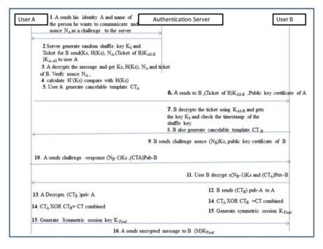
Fig. 31.1 The proposed model for biometric based session key generation protocol
