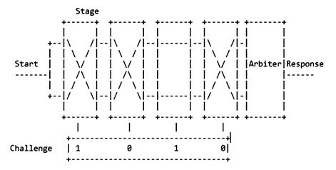
Fig. 18.2 Arbiter Physical Unclonable Function (PUF)
