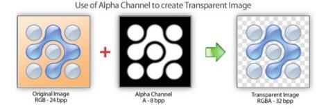
Fig. 33.2 Creation of a transparent image with an Alpha channel
