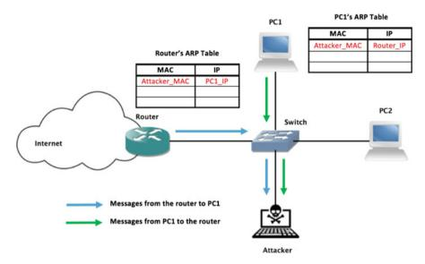
Fig. 6.1 Effects of a MITM attack
