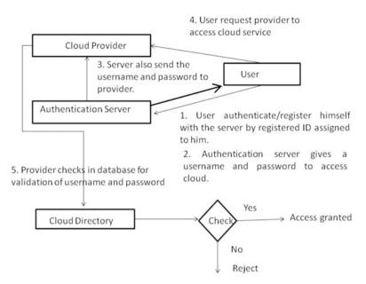
Fig. 31.6 Overall framework for implementation of the proposed protocol in cloud scenario
