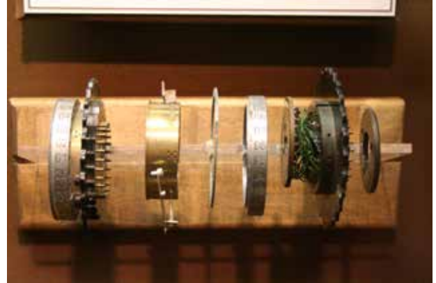
Image 7: Internal connections of rotors, pins, and surfaces cross-linking cables, letter ring
