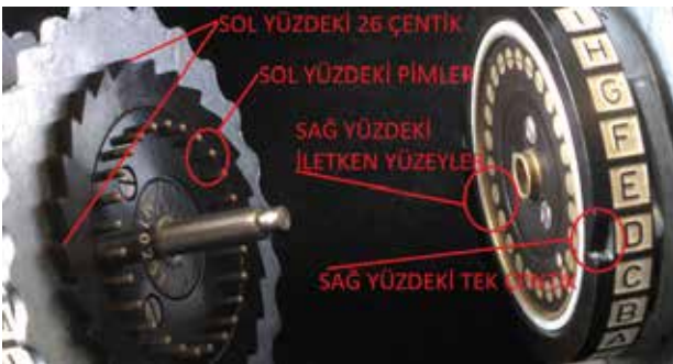
Image 6: Side surfaces of the rotors, pins, and notches
