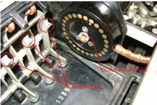
Image 5: Black Round Track is Stationary Rotor, silver colored 3 Piece is Latches
