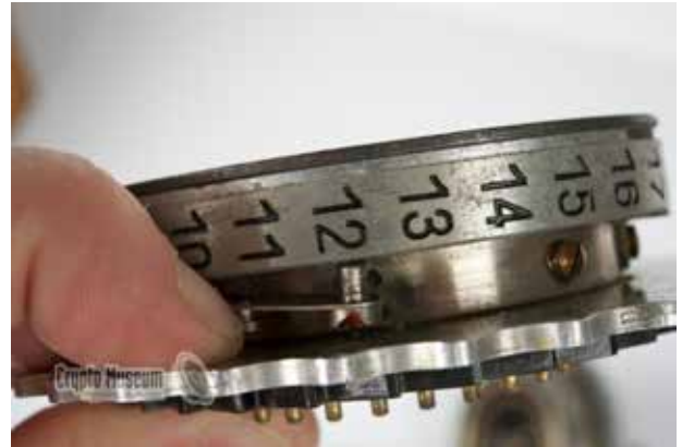
Image 8: Letter ring lock ( http://www.cryptomuseum.com/crypto/enigma/working.htm )
