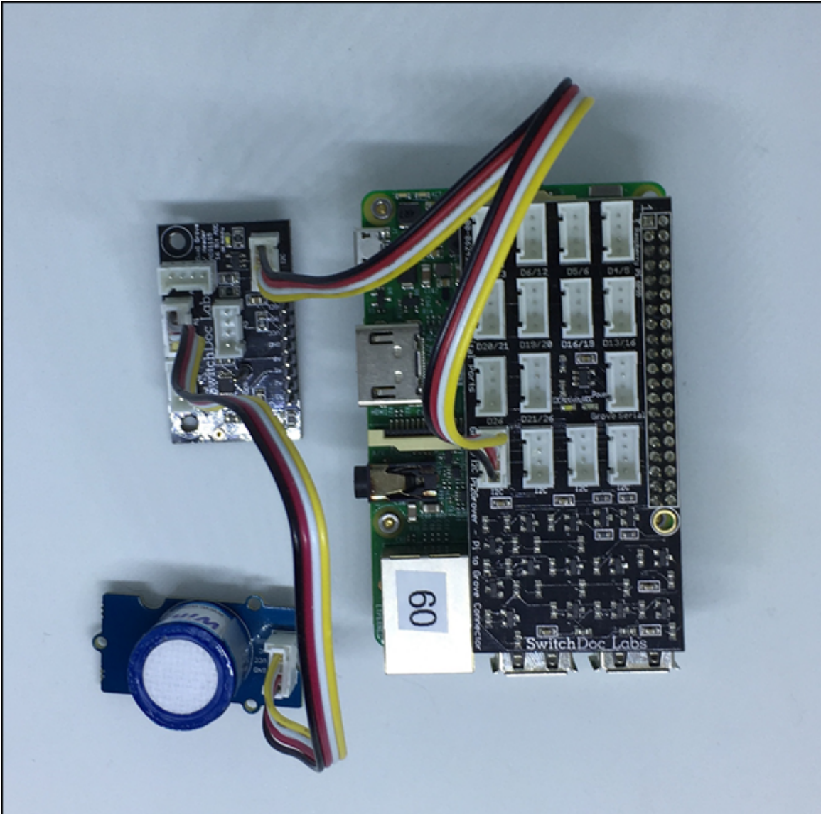
FIGURE 3-7: The complete Raspberry Pi/ADC/oxygen sensor hookup.
