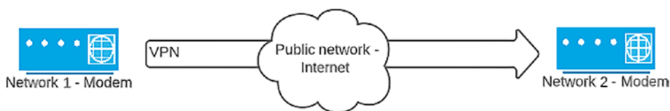
Figure 13-46. How a VPN works at its basic level
