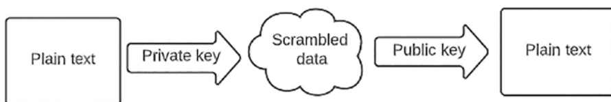
Figure 13-33. Basic encryption flow
