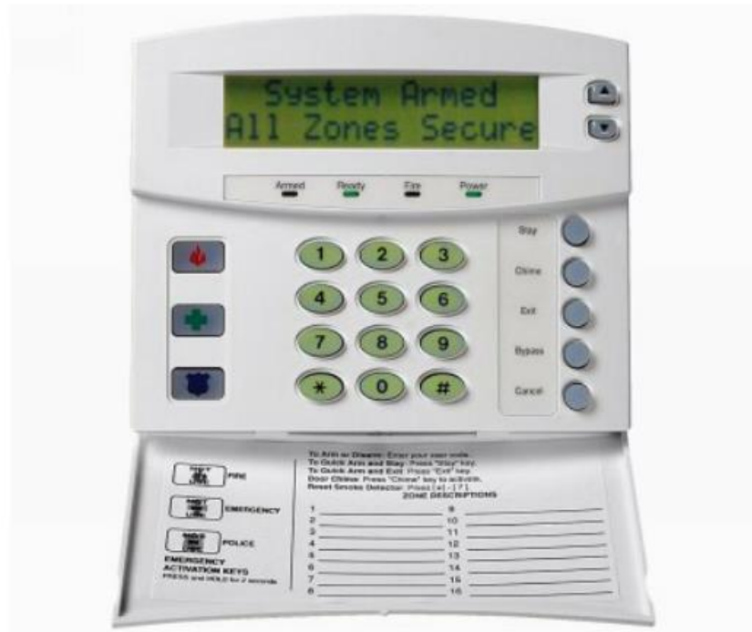
Figure 57. Typical Alarm Control Center
