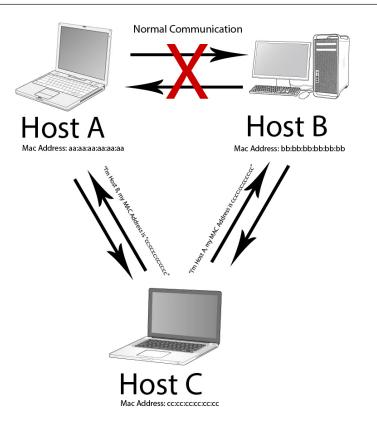
Figure 4.9 – A diagram of an ARP spoof
