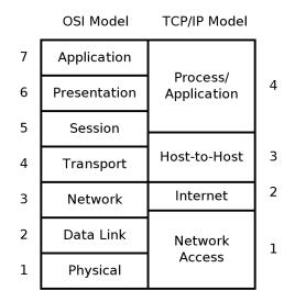
Figure 4.4 – OSI versus TCP/IP
