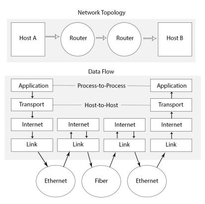
Figure 4.1 - Diagram of a TCP/IP data flow
