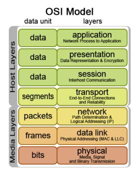
Figure 4.2 – Diagram of the OSI model
